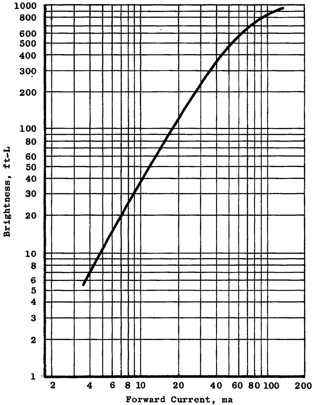
Fig. 1 Light Emitting Diode Brightness, Forward Current Characteristics
