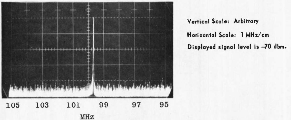
c. Phatomultiplier Tube Response to 100-MHz Input (Spectrum Analyzer)
