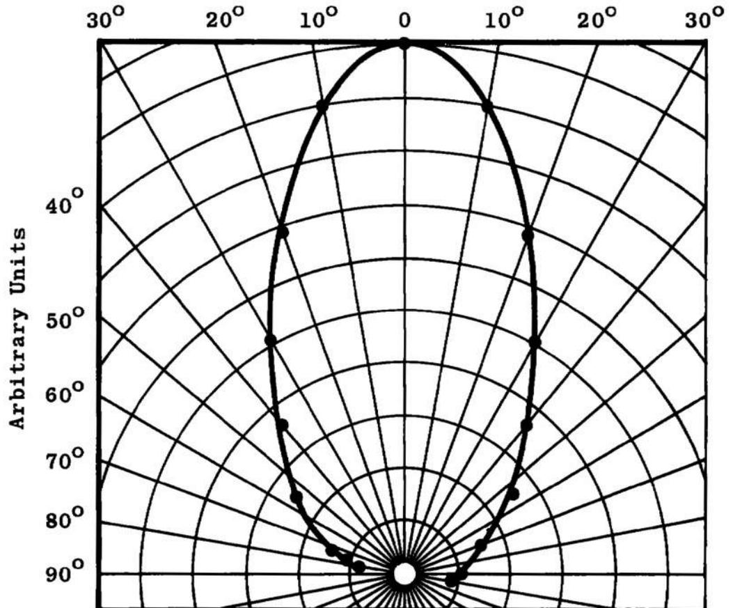
Fig. 3 Light Emitting Diode Radiated Power Angular Distribution
