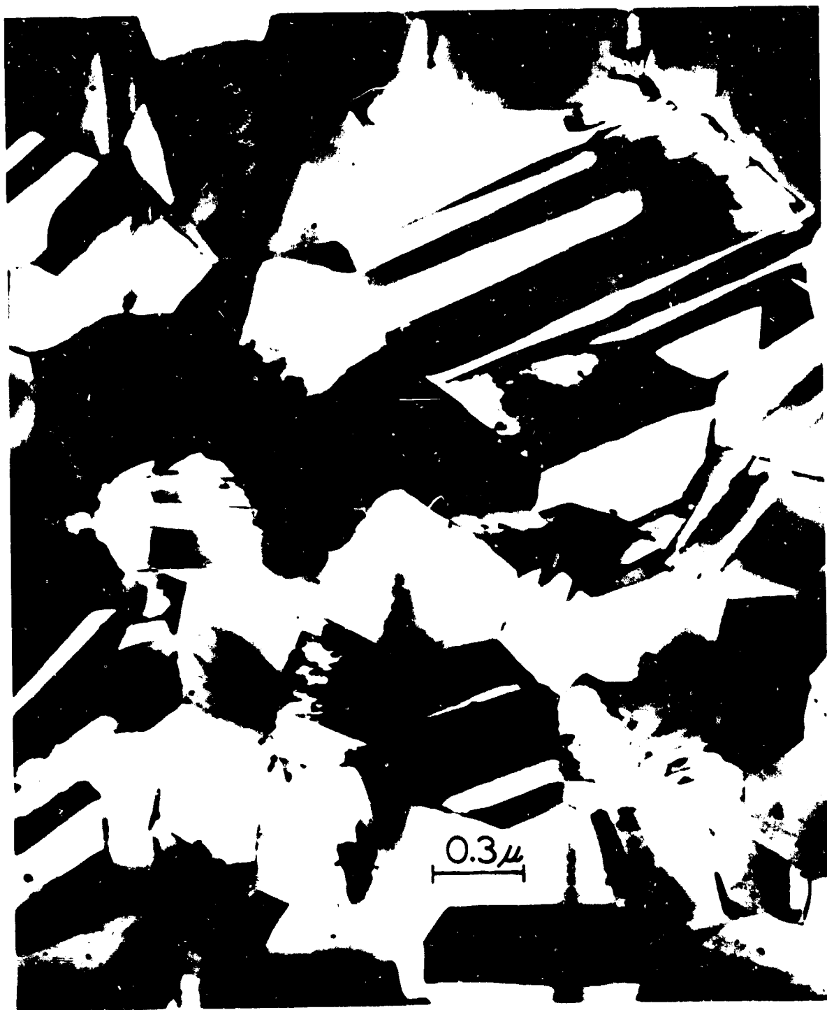
Fig. 2 Bright-field electron transmission micrograph of an indium foil area vapor deposited onto an NaCl (001) substrate at 130°C. The evaporation rate was approximately 1000 Å/sec; and the film thickness shown was approximately 1000 Å.
