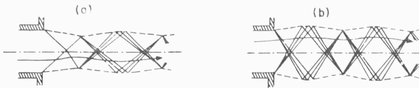
Fig. 2-6 Schematic diagram of exit flow when the value of the exit pressure lies between the second and third critical pressures overexpanded, diagram (a) and when the value of the exit pressure lies below the third critical (design) exit pressure underexpanded, diagram (b). Single lines are oblique shocks, multiple lines are expansion or compression fans, dashed lines are jet boundaries and arrows are flow streamlines.
