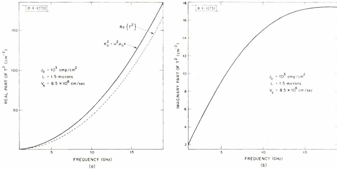
Fig. 6. The real and imaginary parts of  $T^2$  vs frequency ( $f$ ) for an X-band diode with  $L = 1.5$  microns,  $J_0 = 10^3$  amp/cm<sup>2</sup>,  $\alpha_0 = 6.6 \times 10^3$ ,  $\alpha'_0 = 0.164$ , and  $\epsilon = 10^{-12}$  farads/cm. The square of the radial wavenumber (for a TEM cylindrical wave)  $K_0^2$  (which is purely real) is indicated for comparison. (a)  $\text{Re}\{T^2\}$ ; (b)  $\text{Im}\{T^2\}$ .
