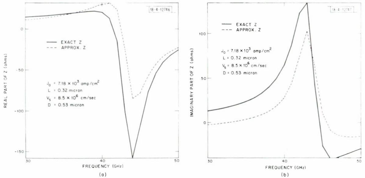
Fig. 4. The approximate and exact silicon IMPATT diode impedance vs frequency ( $f$ ) for a diode in which the avalanche zone ( $L$ ) is 0.32 micron in length, the drift zone ( $D$ ) is 0.53 micron,  $J_0 = 7.18 \times 10^3$  amp/cm<sup>2</sup>,  $\alpha_0 = 3.125 \times 10^4$ ,  $\alpha'_0 = 0.427$ . (a) Real part; (b) imaginary part.
