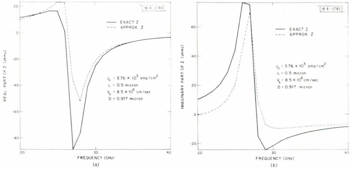
Fig. 3. The approximate and exact silicon IMPATT diode impedance vs frequency ( $f$ ) for a diode in which the avalanche zone ( $L$ ) is 0.5 micron in length, the drift zone ( $D$ ) is 0.92 micron,  $J_0 = 3.76 \times 10^3$  amp/cm<sup>2</sup>,  $\alpha_0 = 2 \times 10^4$ ,  $\alpha'_0 = 0.315$ . (a) Real part; (b) imaginary part.
