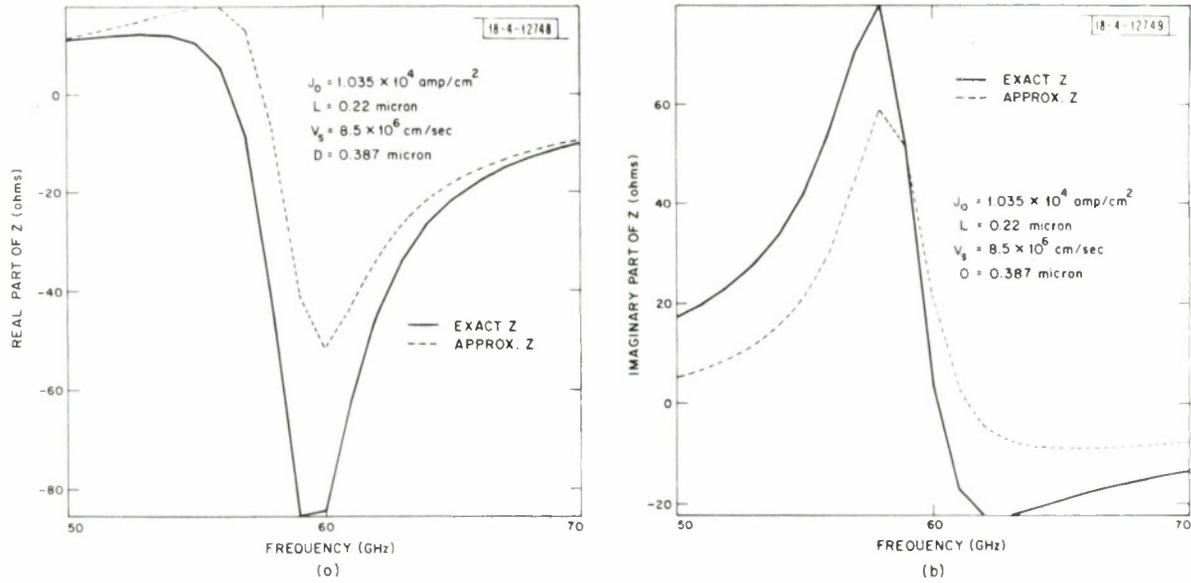
Fig. 5. The approximate and exact silicon IMPATT diode impedance vs frequency ( $f$ ) for a diode in which the avalanche zone ( $L$ ) is 0.22 micron in length, the drift zone ( $D$ ) is 0.387 micron,  $J_0 = 1.035 \times 10^4$  amp/cm<sup>2</sup>,  $\alpha_0 = 4.545 \times 10^4$ ,  $\alpha'_0 = 0.542$ . (a) Real part; (b) imaginary part.
