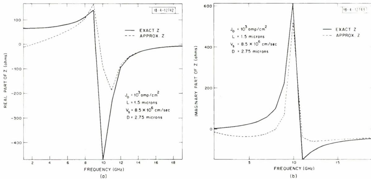
Fig. 2. The approximate and exact silicon IMPATT diode impedance vs frequency ( $f$ ) for a diode in which the avalanche zone ( $L$ ) is 1.5 microns in length, the drift zone ( $D$ ) is 2.75 microns,  $J_0 = 10^3 \text{ amp/cm}^2$ ,  $\alpha_0 = 6.6 \times 10^3$ ,  $\alpha'_0 = 0.164$ . (a) Real part; (b) imaginary part.
