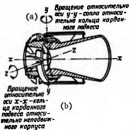
Figure 6.26. Turning cone with universal joint suspension. a -- Turning relative to y-y axis relative to ring of universal joint suspension; b -- Turning relative to x-x axis of the ring of the universal joint suspension with respect to stationary casing.
