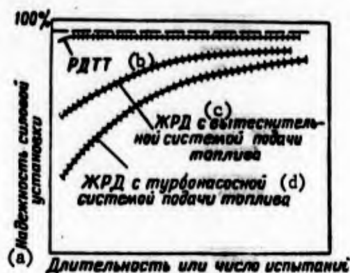
Figure 4.8. Dependence of reliability factor on number of flight tests in process of working through. a -- Reliability of power apparatus; b -- RDTT [solid-fuel rocket engine/]; c -- ZhRD [liquid-fuel rocket engine?] with displacer system of fuel feed; d -- ZhRD with turbine-pump system of fuel feed.
