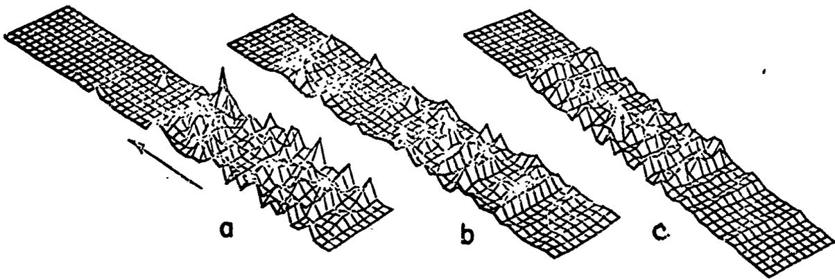
Fig. 14. Equal time comparison of energy penetration into a harmonic lattice containing 15% heavy impurities (a) with that into a 15% light impurity region (b). Impurity sites are identical in the two pictures. (c) corresponds to heavy impurities in anharmonic case.
