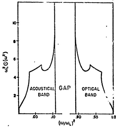
Fig. 8. Distribution of  $\omega^2$  for diatomic lattice with  $M_2 = 8M_1$  and  $\gamma_1/\gamma_2 = 8$ .
