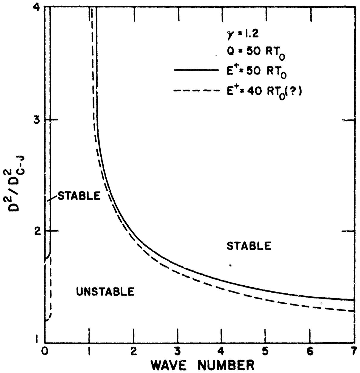
Figure 5. Stability of the steady one-dimensional solution to perturbations as a function of detonation velocity  $D$  and transverse (spatial) wave number of the perturbation. The wave number is in units of  $2\pi$  divided by the distance from the shock to the point at which the reaction is half completed ( $\lambda=1/2$ ) in the steady solution for the given value of  $D$ . Most of the  $E^+=40RT_0$  curve is guessed from other results.
