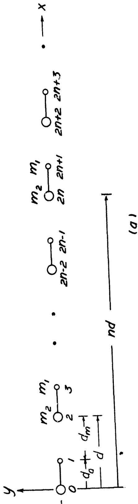
(a) Schematic drawing of a one-dimensional row lattice with two values of point masses ( $m_2 > m_1$ ) used to represent a diatomic lattice. The notation is chosen so that all even-numbered points have masses,  $m_2$ , and odd-numbered points have masses,  $m_1$ . The distance between atoms,  $d_a$ , is taken to be smaller than the distance between molecules,  $d_m$ , in this drawing, but in general any relative values for intra and intermolecular distances can be assumed.
