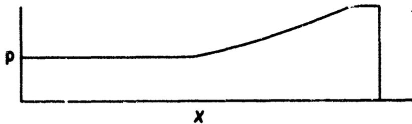
Figure 1. The flow behind a detonation initiated at the closed end of a tube.
