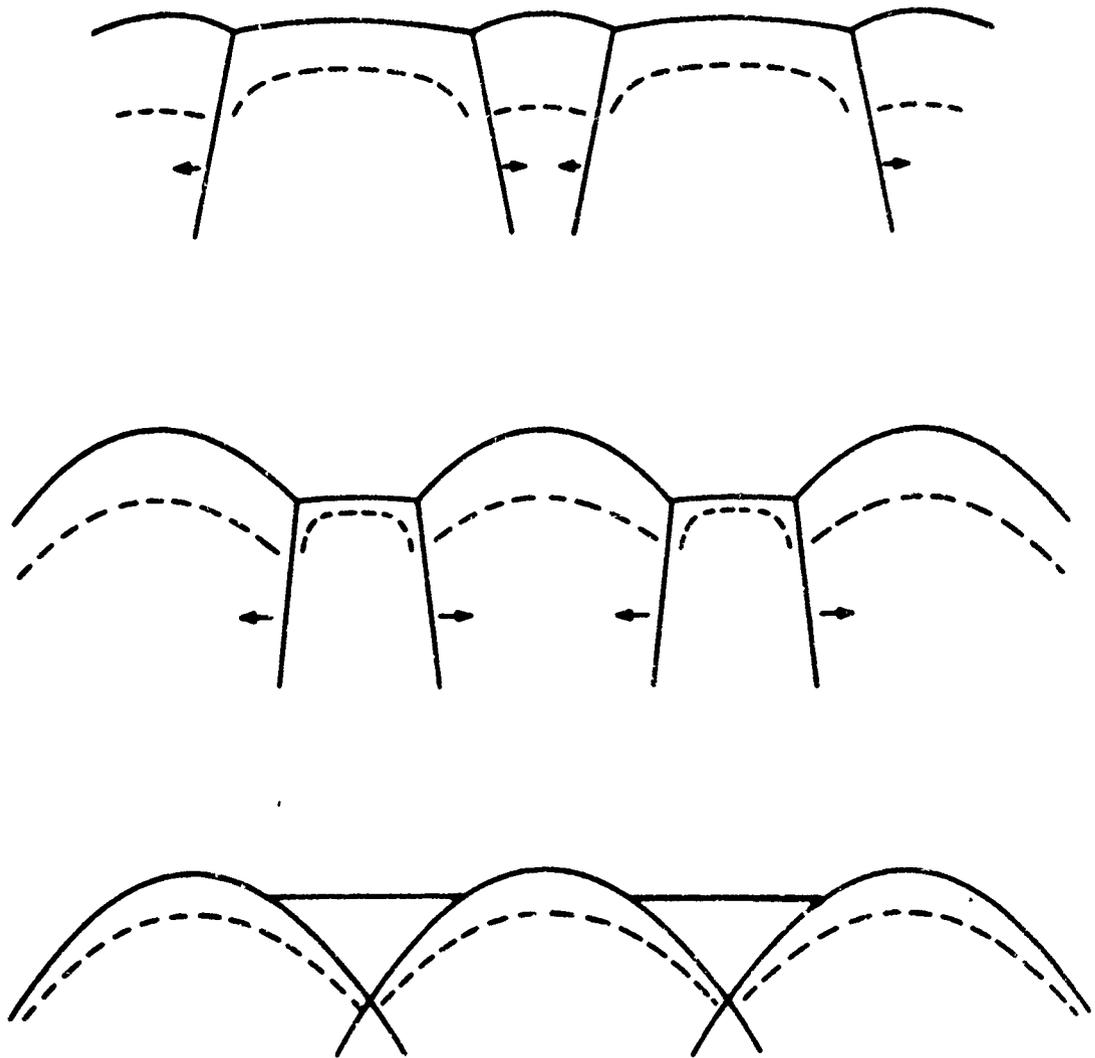
Figure 9. Development of front structure. The wave moves from bottom to top of the figure. The dashed lines indicate the end of the reaction zone.
