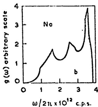
Fig. 7. (b) Experimental frequency spectrum of sodium.
