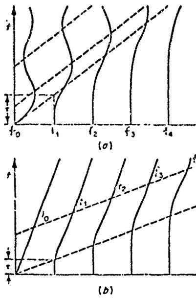
Fig. 1. Curves (a) represent the trajectories of various masses when the end particle is given an initial impulse. Curves (b) represent the situation in which the end particle is driven with a constant velocity.
