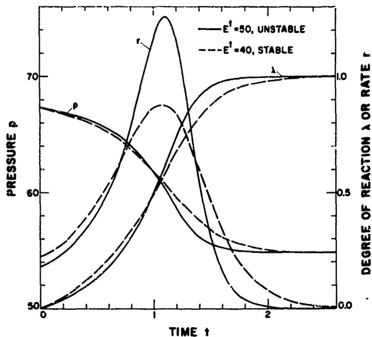
Figure 6. Steady solutions for the cases  $\gamma=1.2$ ,  $Q=50RT_0$ ,  $D^2=1.6 D_{CJ}^2$ ,  $E^+=50RT_0$  (stable) and  $E^+=40RT_0$  (unstable). The time origin and unit are such that the fluid element passes through the shock at  $t=0$  and is half-reacted ( $\lambda=1/2$ ) in a given steady solution at  $t=1$ . The pressure is in units of the initial pressure.
