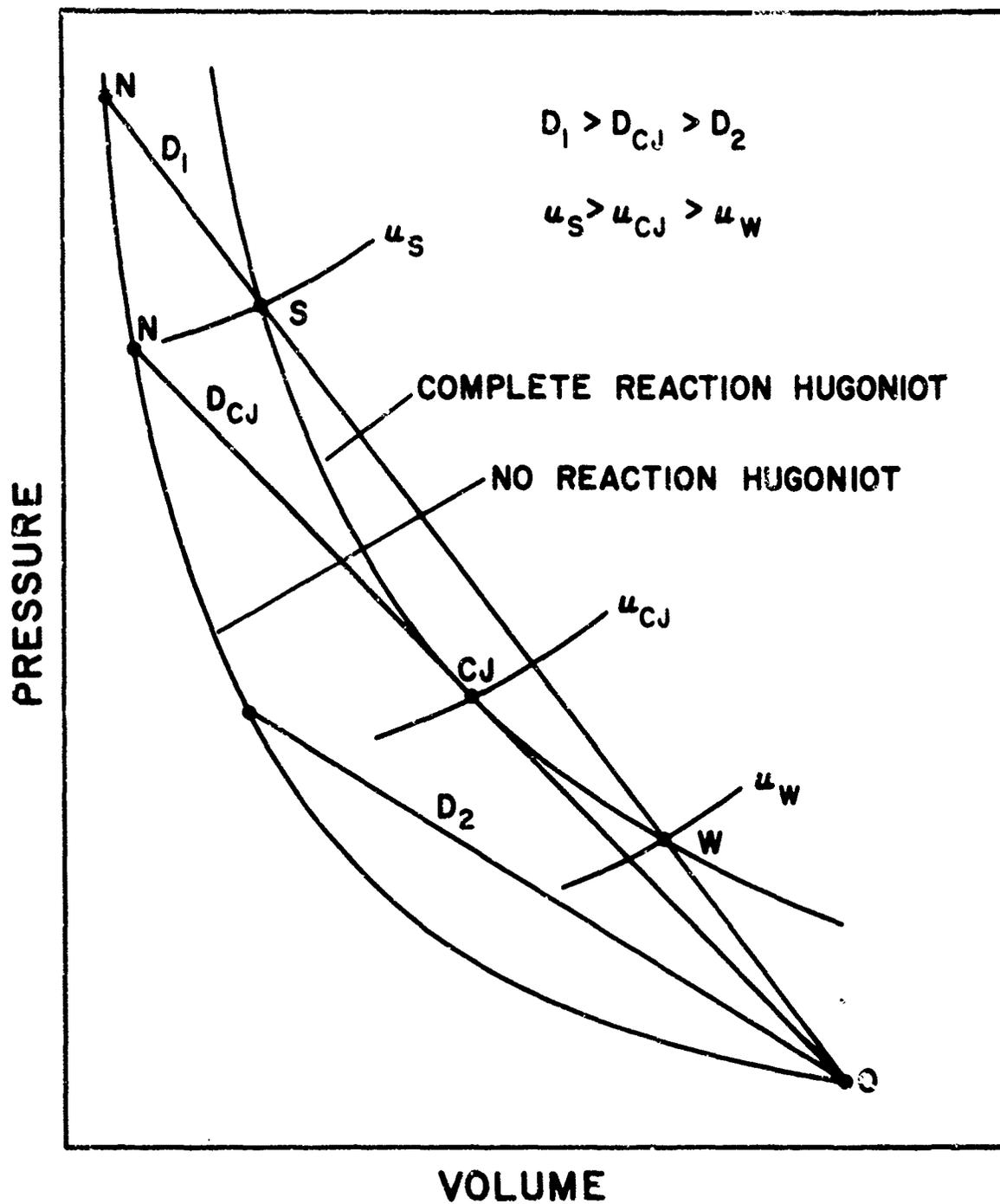
Figure 2. Curves of constant  $D$  and constant  $u$  and solutions of the Hugoniot equation in the  $p - v$  plane. Point  $O$  is the initial state.
