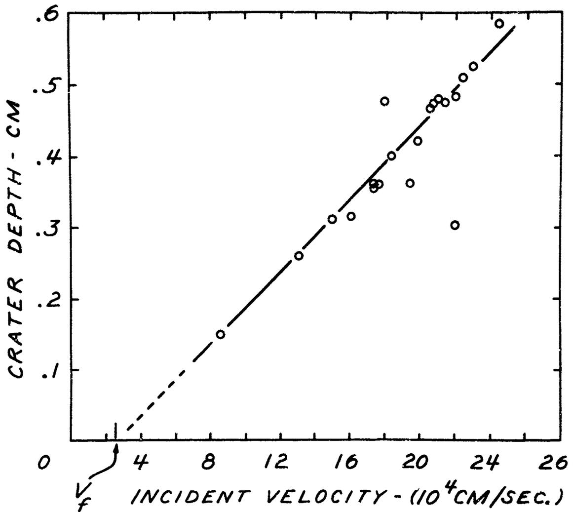
**FIG. 12** Crater depth vs. projectile velocity for 0.483-cm iron spheres fired into semi-infinite iron targets. (Data from reference 17.)
