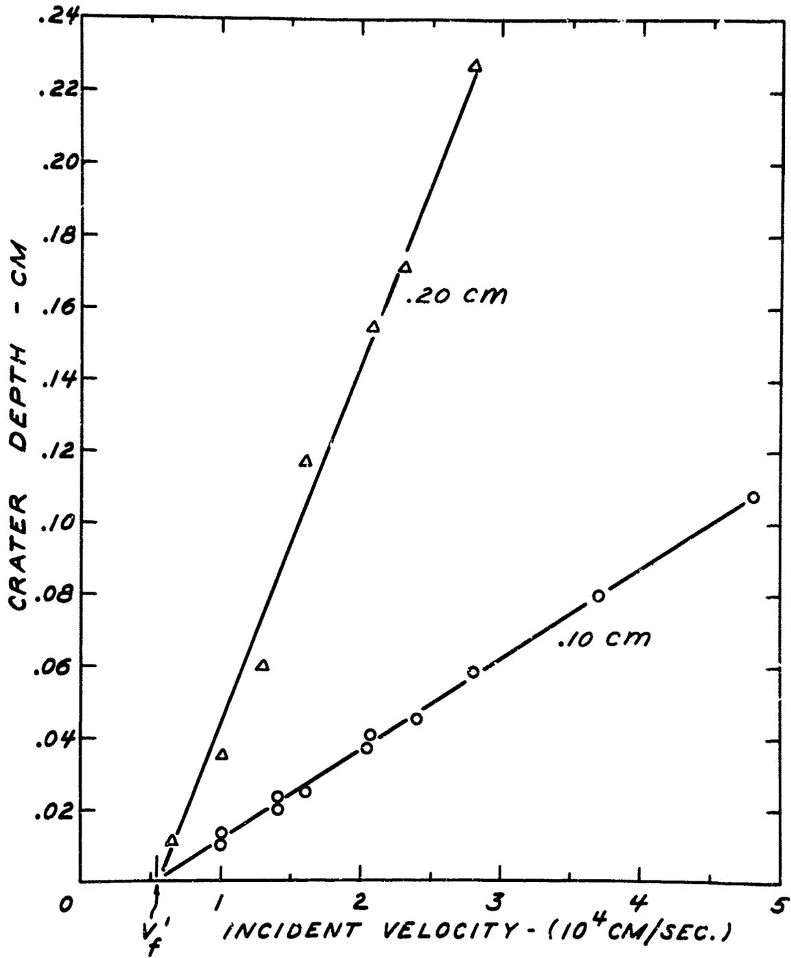
**FIG. 11** Crater depth vs. incident velocity for two sizes of mercury drops impacting lead target plates. (Data from Olive G. Engel.<sup>16</sup>)
