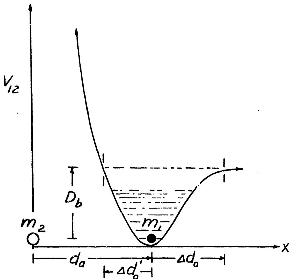
**FIG. 9** Representation of the interatomic "pair" interaction potential,  $V_{12}$ , between two masses (atoms) of the diatomic row lattice of Fig. 7 as a function of the distance,  $x$ , between atoms. If the bond distance is shortened an amount  $\Delta d_2$  the resulting potential energy of  $m_1$  (relative to  $m_2$ ) may equal the bond dissociation energy,  $D_b$ , and bond breaking or rupture can result as discussed in the text.
