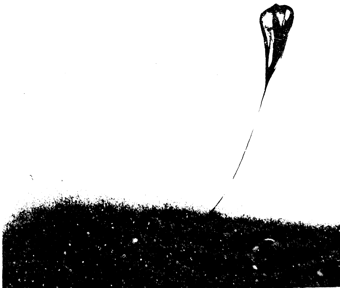
Figure 1. The 28.7-million-cubic-foot balloon just before launch. The major portion of the balloon's 587-foot length is still encased in the launch sleeve.
