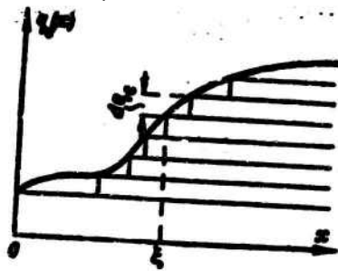
Fig. 8-6. Heat exchange in a round tube with arbitrary variation in heat-flow density at the wall.
