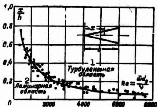
Fig. 5-15. Laminar- and turbulent-flow regions in triangular tube with acute angle. 1) Turbulent region; 2) laminar region.
