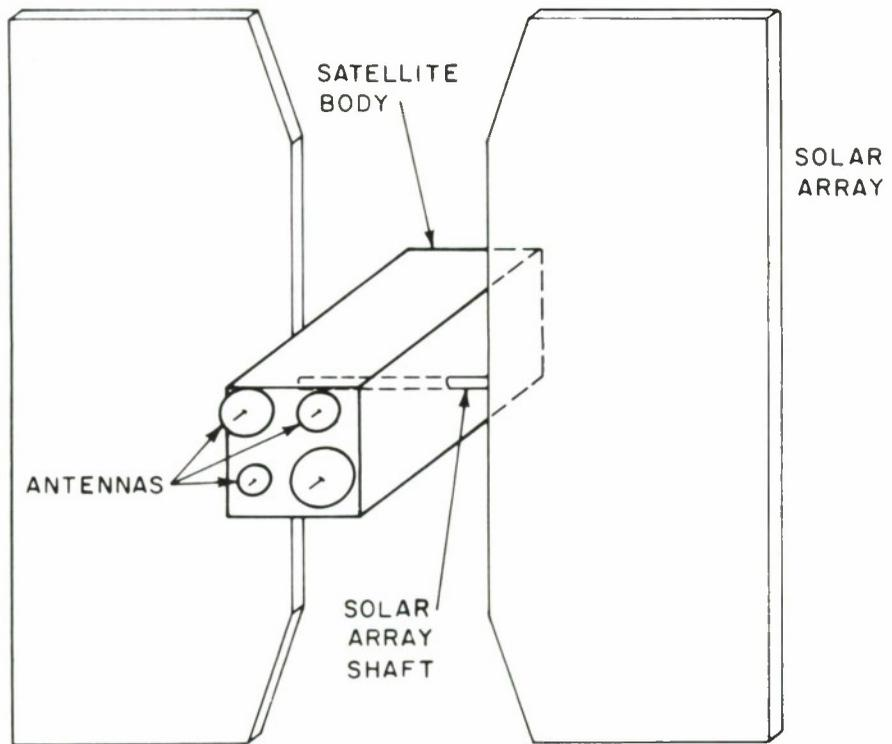
Fig. 9. Satellite configuration.
