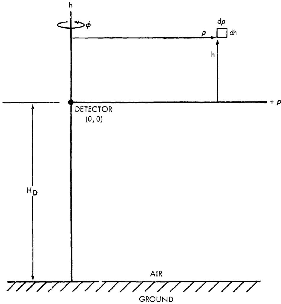
Figure 1. Geometry for Calculation of Last-Collision Fraction
