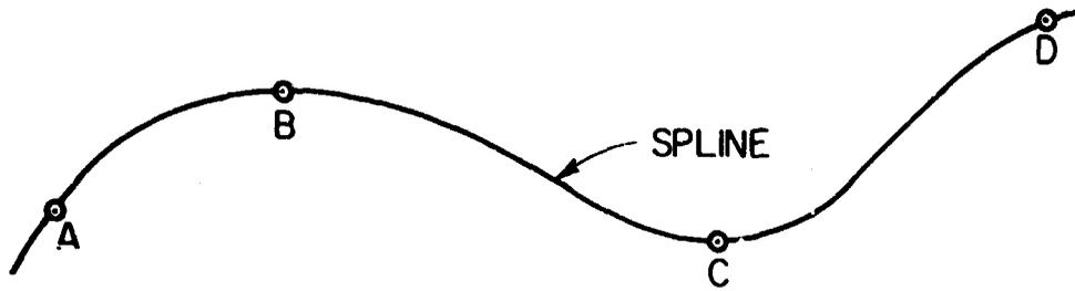
Fig. 1a: Spline passing through points A, B, C, and D.
