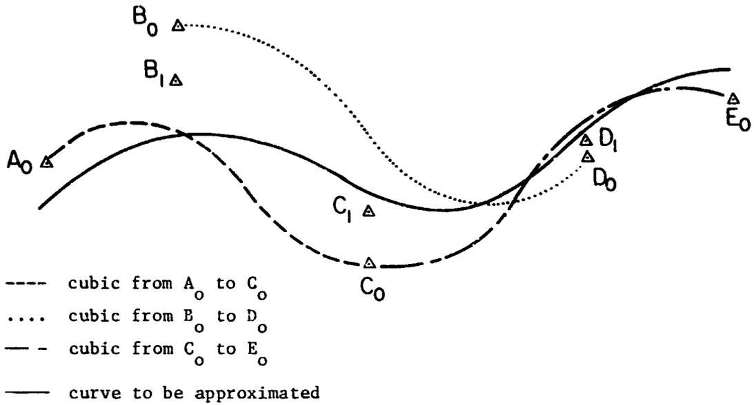
Fig. 4a: Set of three cubic splines approximating a curve.
