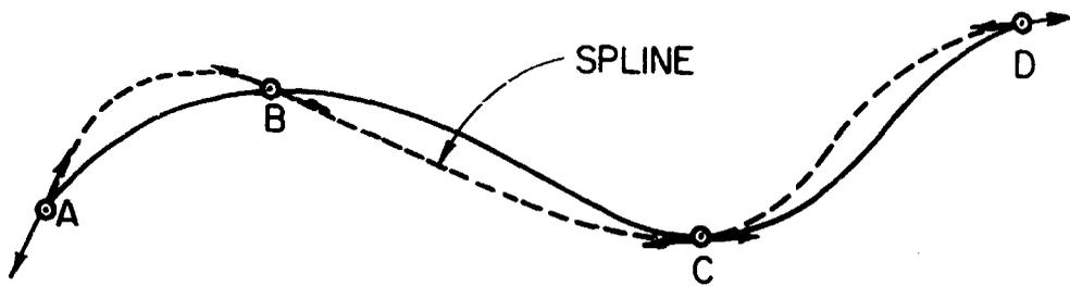
Fig. 1b: Spline passing through points A, B, C, and D where slopes have been prescribed at the points.
