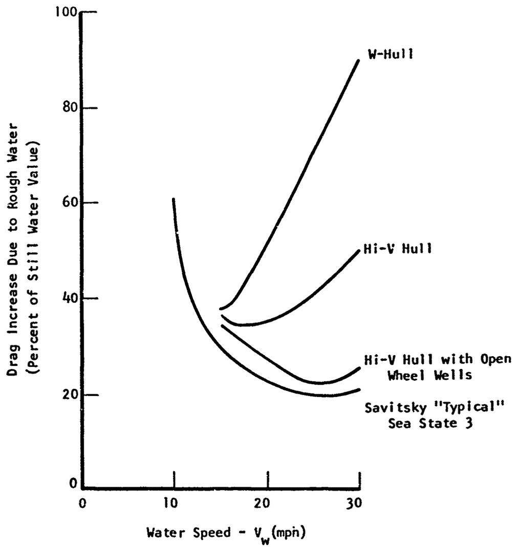
FIG. 47. INCREASED DRAG EXPERIENCED IN 3'x60' REGULAR HEAD SEAS, WHEN COMPARED TO STILL WATER DRAG<sup>1,79</sup>
