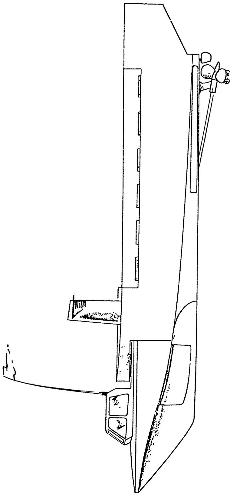
FIG. 15. CONCEPT NO. 1 - A 5-TON, 6x6, LOW-CHINE, V-BOTTOM PLANING AMPHIBIAN WITH RETRACTABLE PROPELLER AND TUNNEL, RETRACTABLE WHEELS, ROLLER DRIVE, "GOER"-TYPE ARTICULATED STEERING
