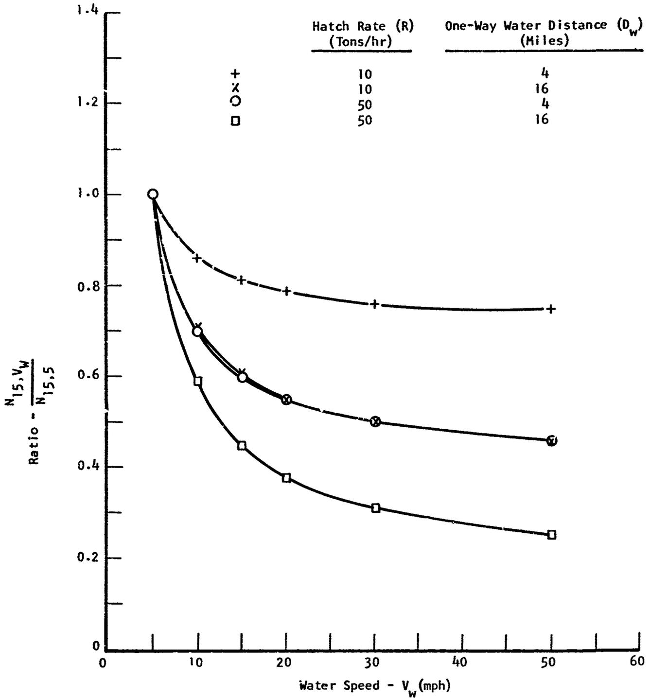
FIG. 6. REDUCTION IN THE REQUIRED NUMBER OF 15-TON VEHICLES ACHIEVED BY INCREASING WATER SPEED WHEN COMPARED TO A STANDARD OF 5 MPH
