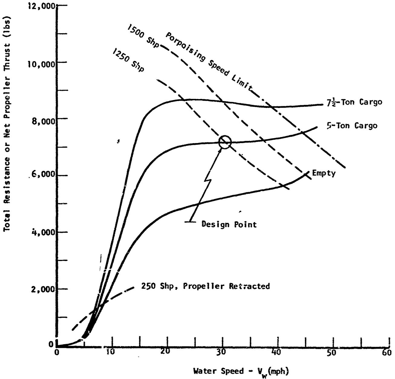
FIG. 29. CONCEPT NO. 1 - CALCULATED STILL WATER PERFORMANCE
