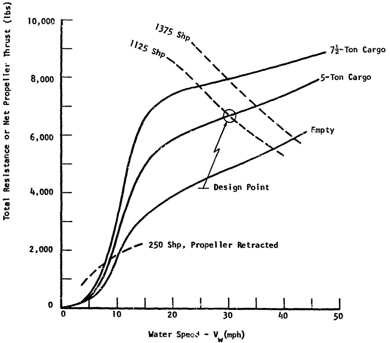
FIG. 3i. CONCEPT NO. 3 - CALCULATED STILL WATER PERFORMANCE
