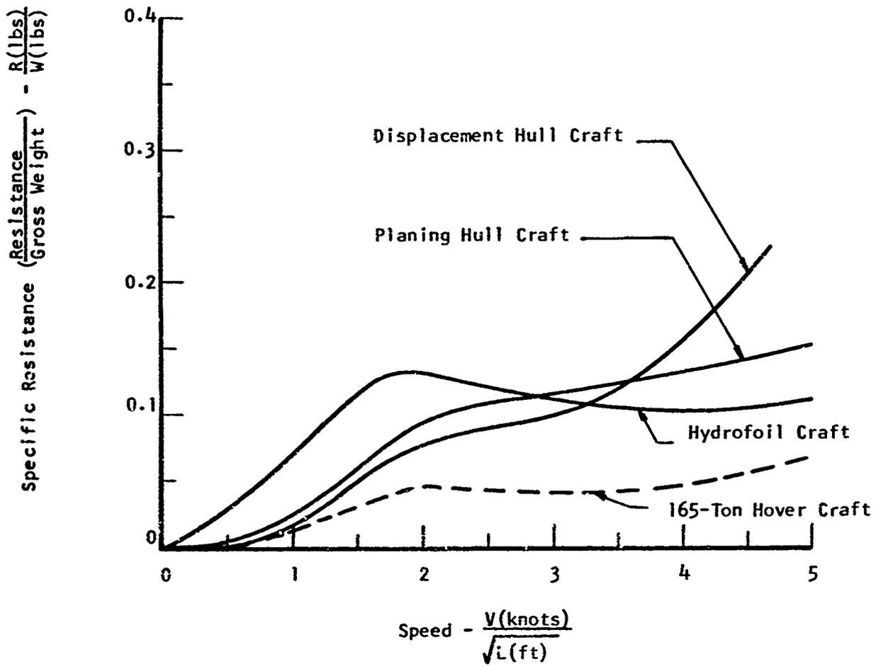
FIG. 2. SPECIFIC RESISTANCE OF WELL DESIGNED BOATS<sup>18,23</sup>
