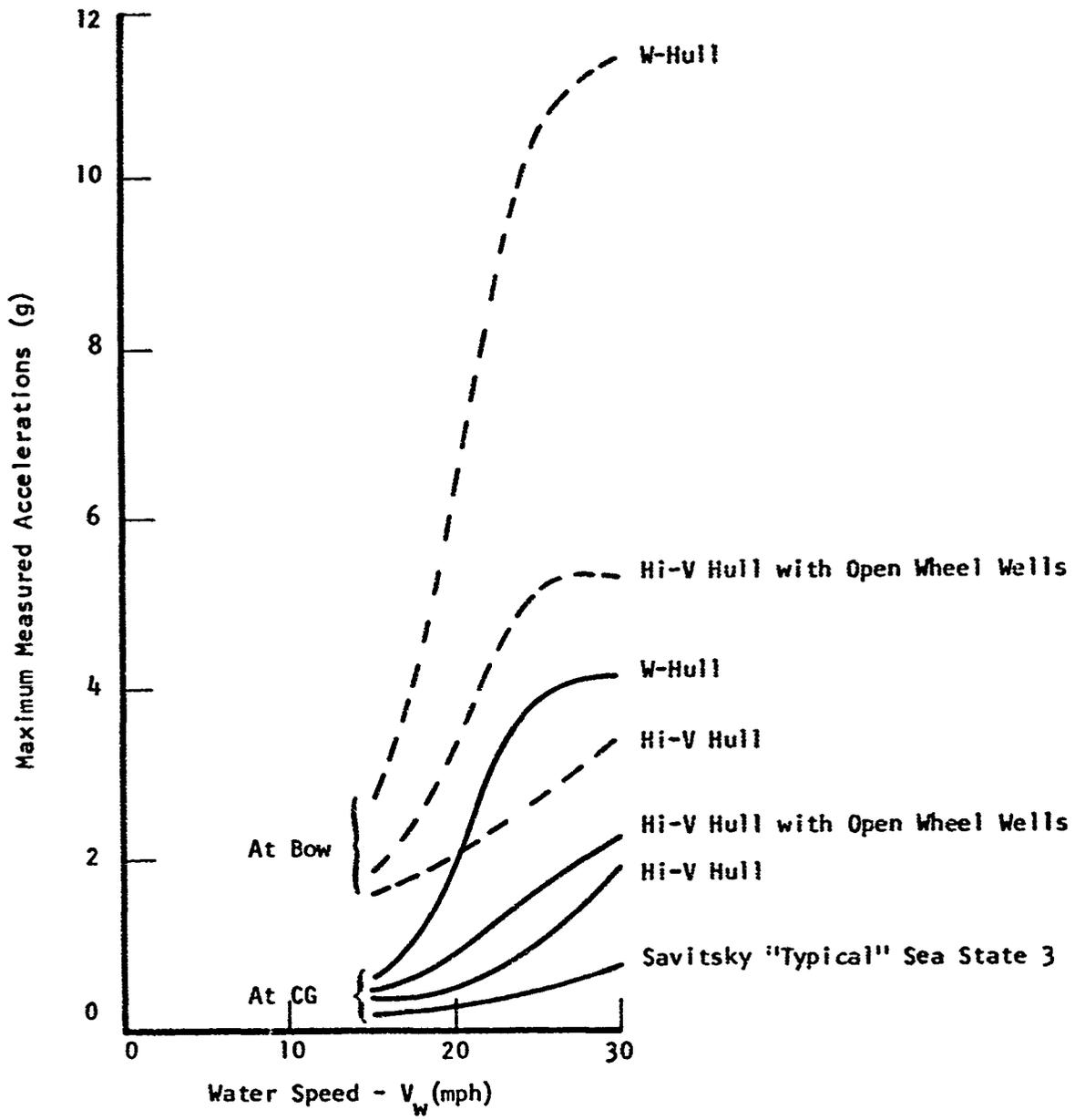
FIG. 48. MAXIMUM ACCELERATIONS MEASURED IN 3'x60' REGULAR HEAD SEAS<sup>1,79</sup>
