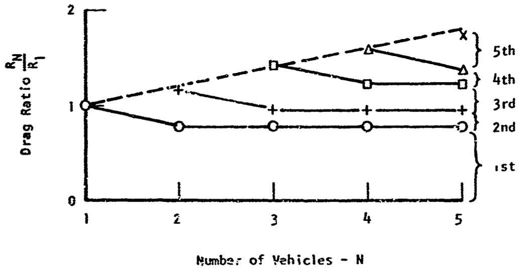
FIG. 51. DRAG BREAKDOWN BY VEHICLE LOCATION IN A TRAIN OF LVT-5 LANDING CRAFT AT ABOUT 7 MPH<sup>50</sup>
