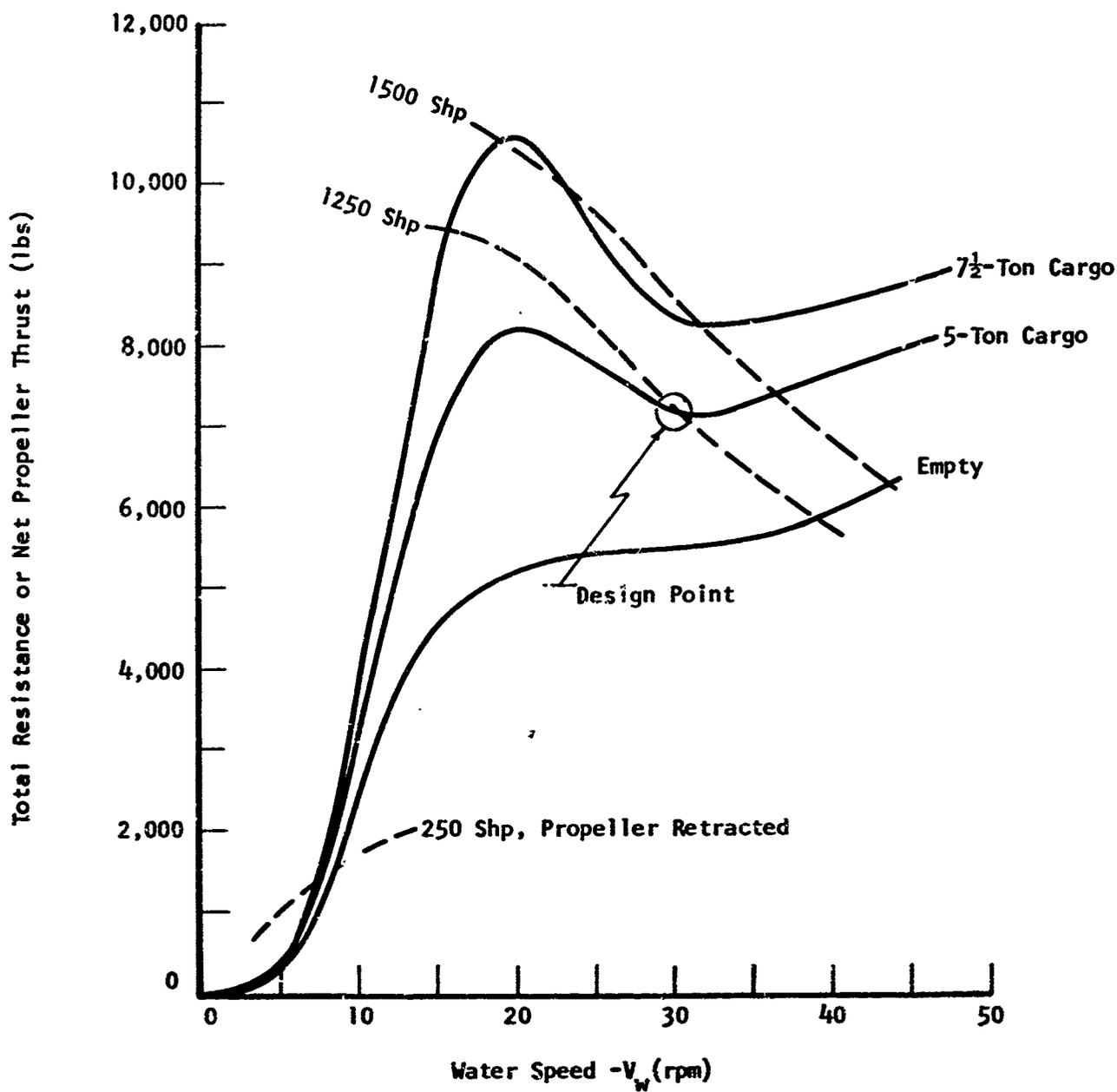
FIG. 32. CONCEPT No. 4 - CALCULATED STILL WATER PERFORMANCE
