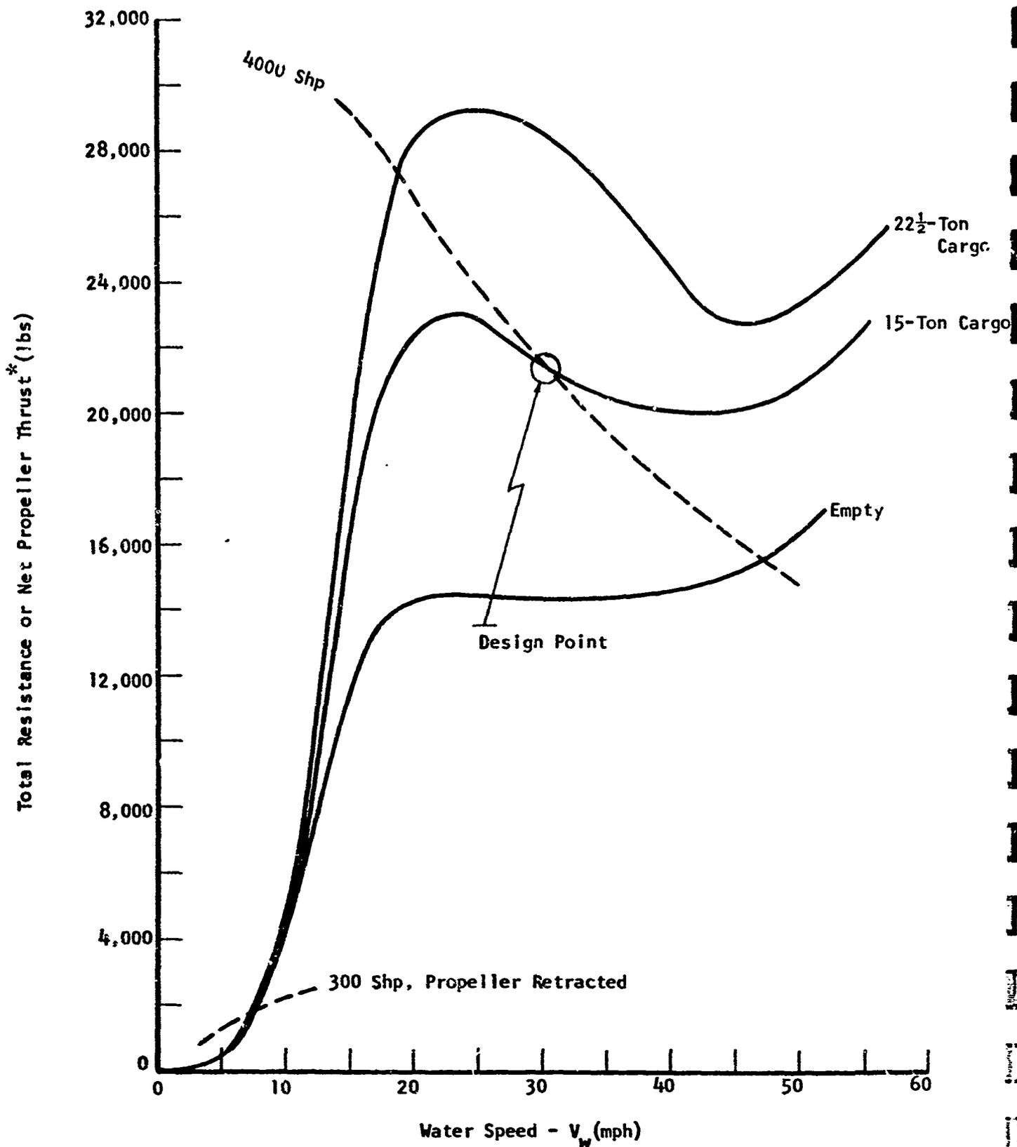
FIG. 33. CONCEPT NO. 5 - CALCULATED STILL WATER PERFORMANCE
