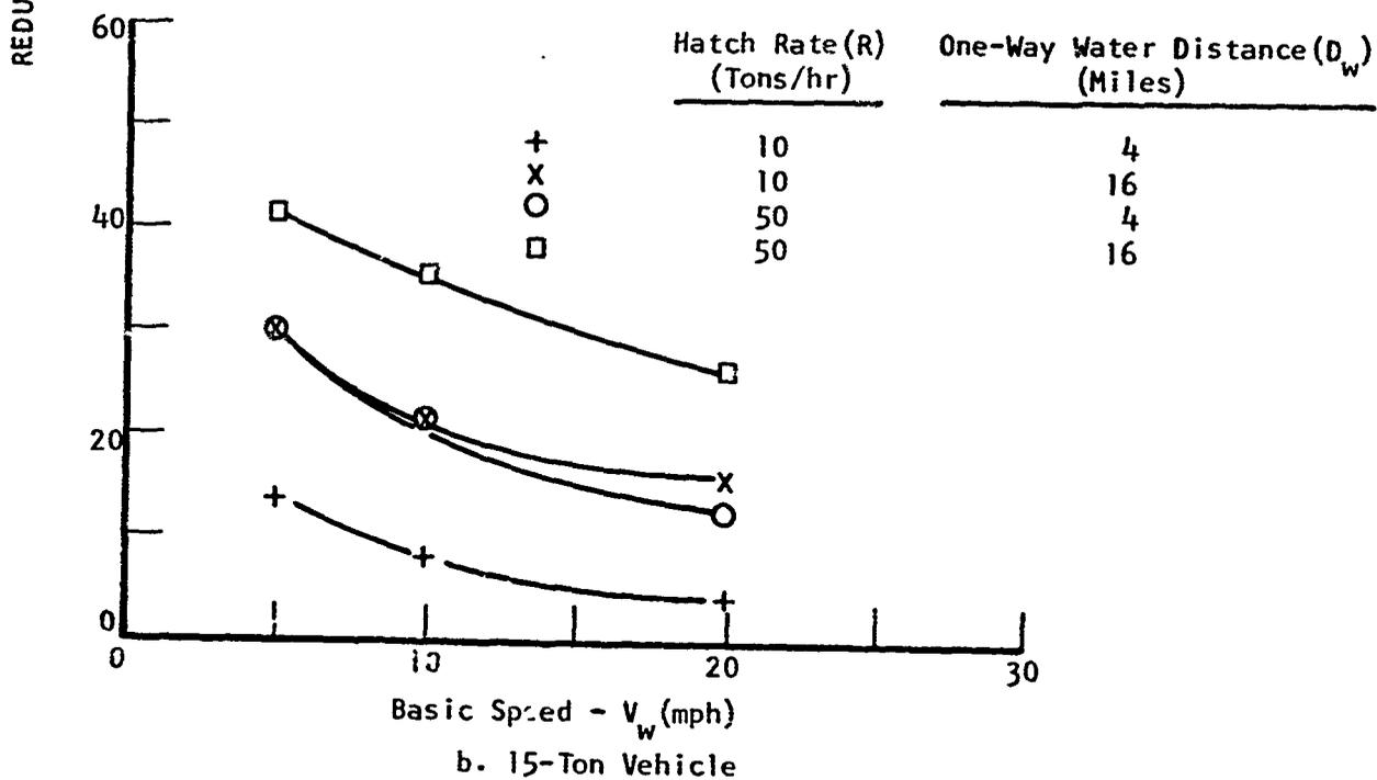
FIG. 7. REDUCTION IN THE REQUIRED NUMBER OF VEHICLES TO BE ACHIEVED BY DOUBLING A GIVEN SPEED, 5 AND 15-TON VEHICLES
