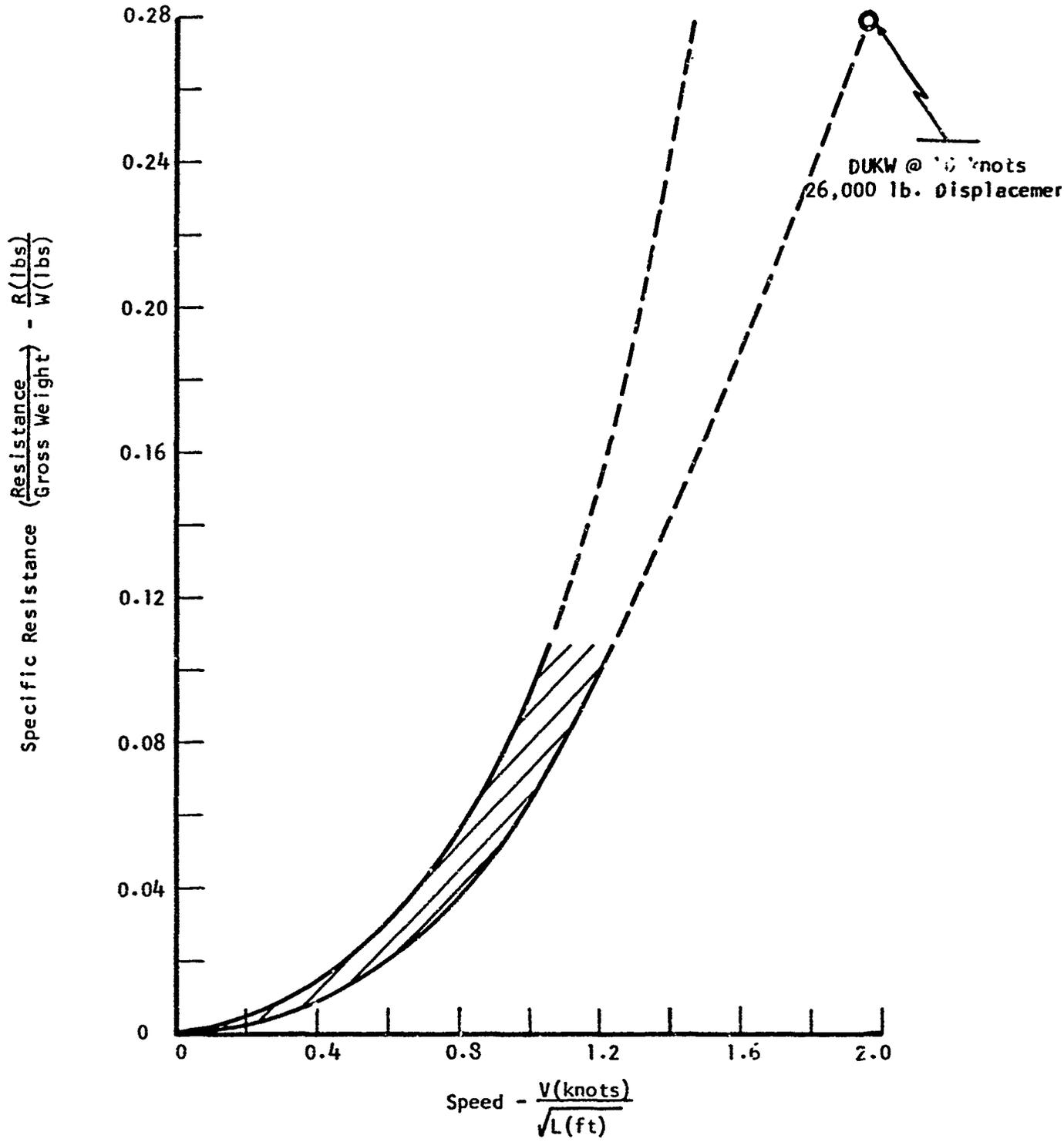
FIG. 1. SPECIFIC RESISTANCE FOR A RANGE OF WHEELED AMPHIBIANS<sup>19</sup>
