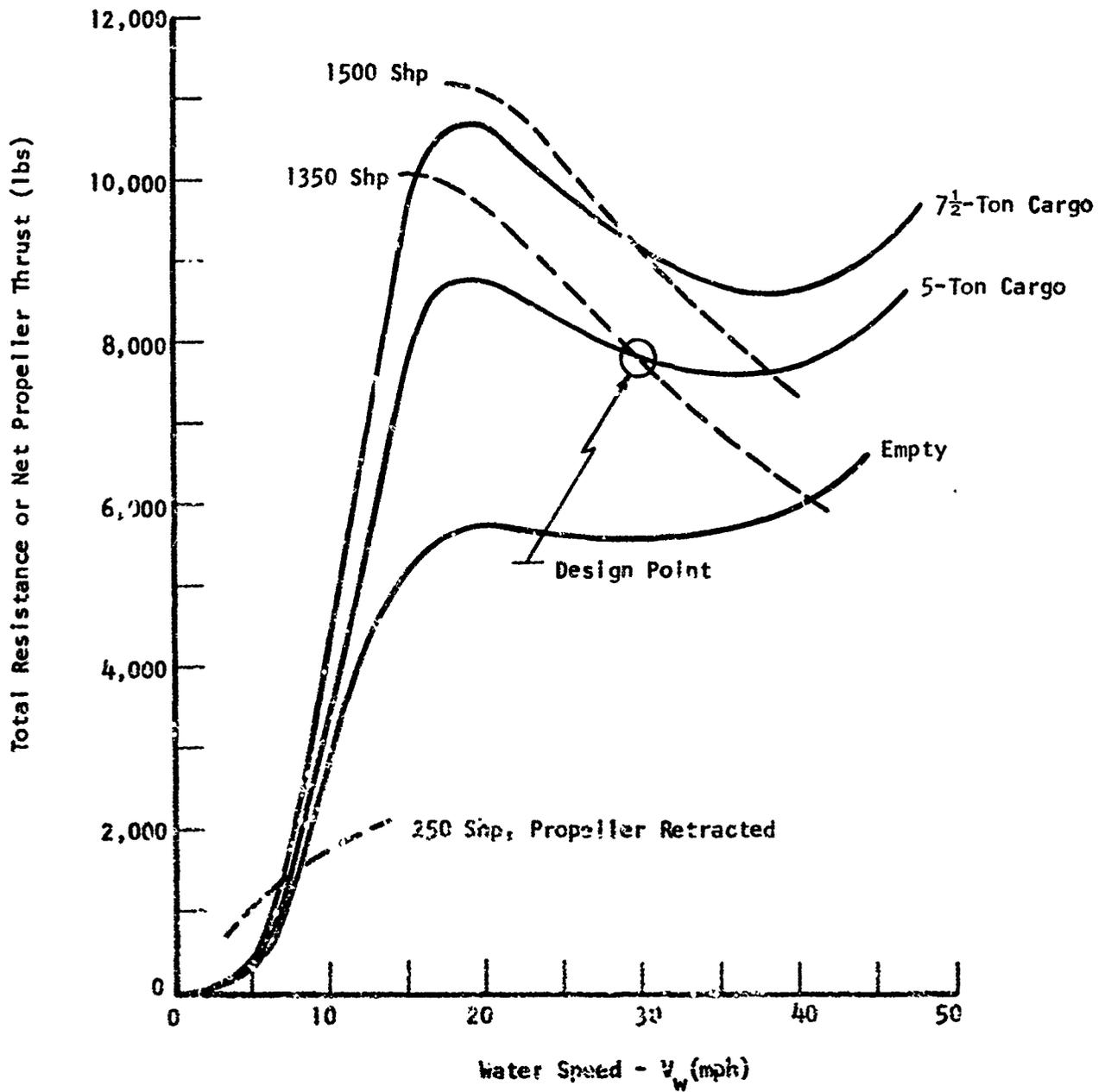
FIG. 30. CONCEPT NO. 2 - CALCULATED STILL WATER PERFORMANCE
