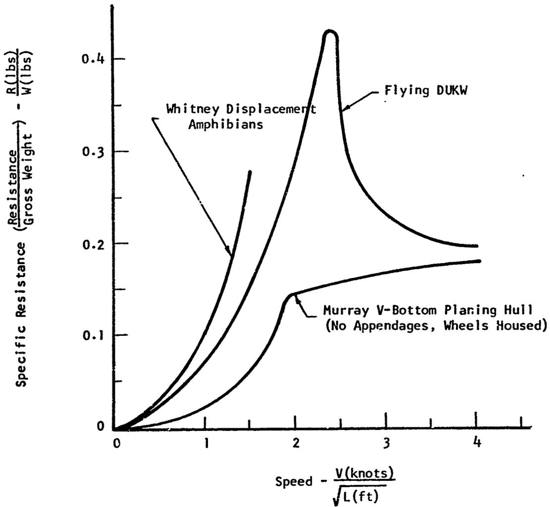
FIG. 4. SPECIFIC RESISTANCE OF VARIOUS TYPES OF AMPHIBIOUS TRUCKS<sup>1,19,25</sup>
