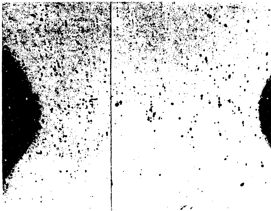
Fig. 31. Unetched Cross-Section of Cold Welded Annealed Tough Pitch Copper of 10\mu Grain Size (a) L_C/L_{F_0} = 0.5 (b) L_C/L_{F_0} = 1.0 Orig. Mag. 60x
