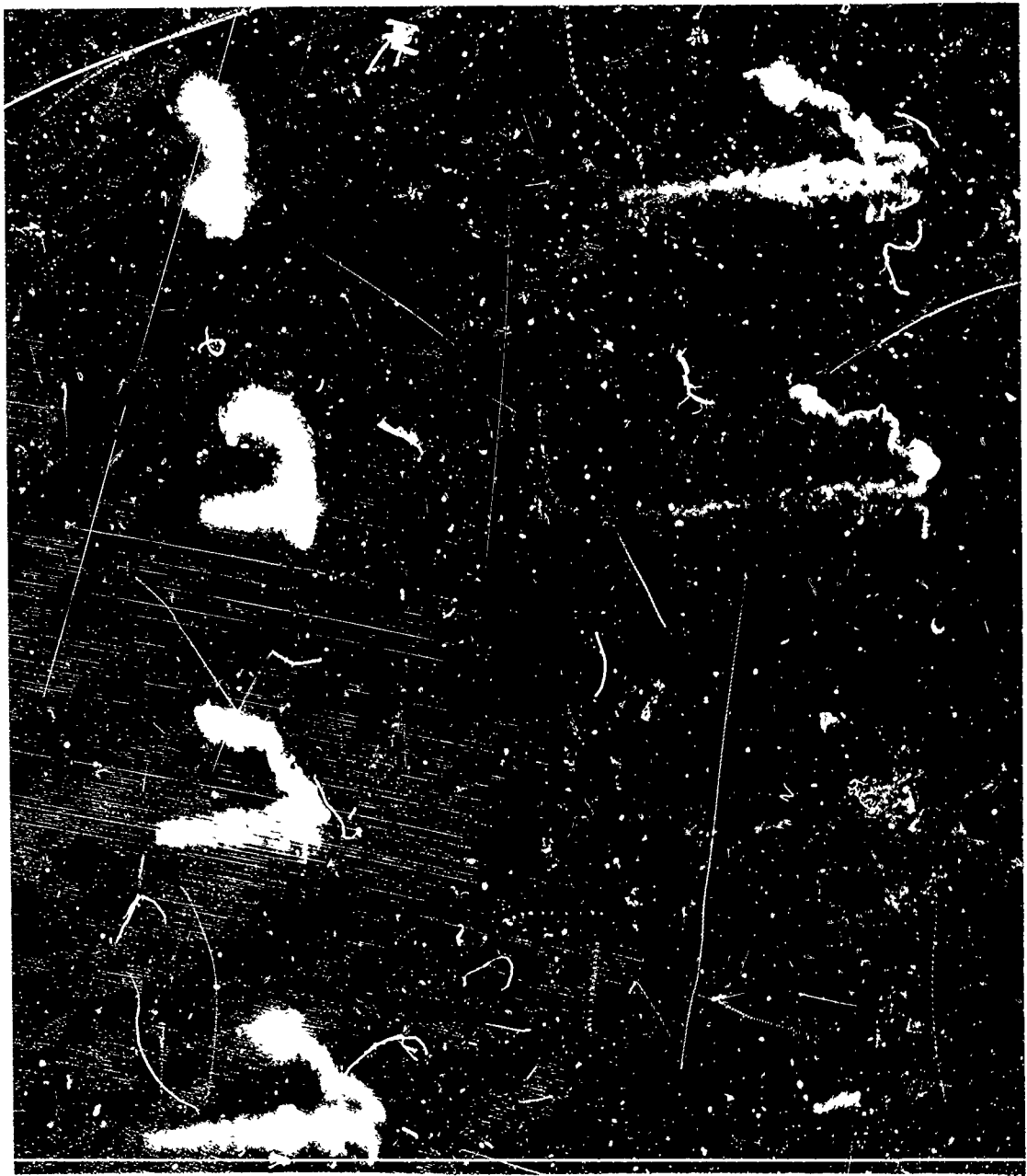
Figure 13 Sequence from Fastax film of swept artificial lightning discharge with approximately five milliseconds separation per photograph and an air speed of 155 mph. Discharge from electrode above contacts skin and hangs-on to forward point while arc is swept nearly the full length of the five foot panel.
