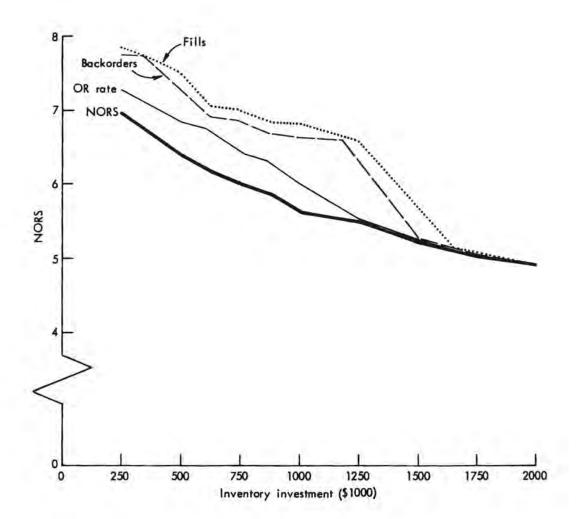
Fig. 1--NORS vs. cost of various stockage policies
