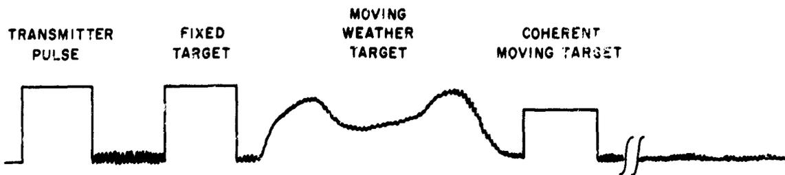
Figure 2a. Typical "A" Scope Display of Radar Video
