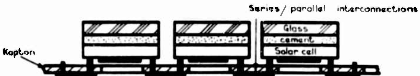
D Wrap-round contacts. Solder-through technique with windows in Kapton
