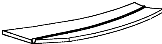
(b) LONGITUDINAL BENDING DISTORTION OF A SINGLE-VEE BUTT WELD
