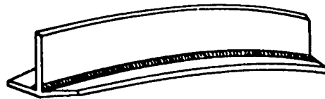
(a) LONGITUDINAL DISTORTION OF A BUILT-UP BEAM
