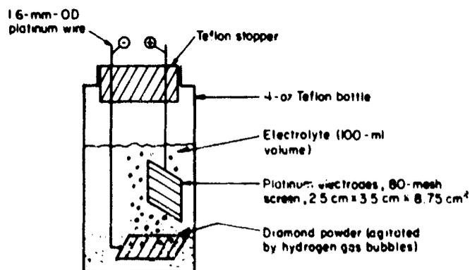
FIGURE 10. ELECTROLYSIS CELL FOR PURIFYING DIAMOND POWDER
