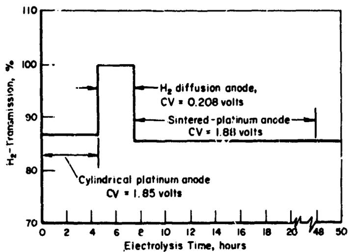
FIGURE 2. RESULTS OF ELECTROLYSIS WITH KOH ELECTROLYTE
