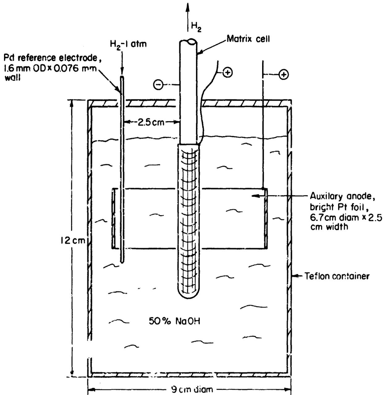
FIGURE 11. FREE-ELECTROLYTE EXPERIMENTAL UNIT
