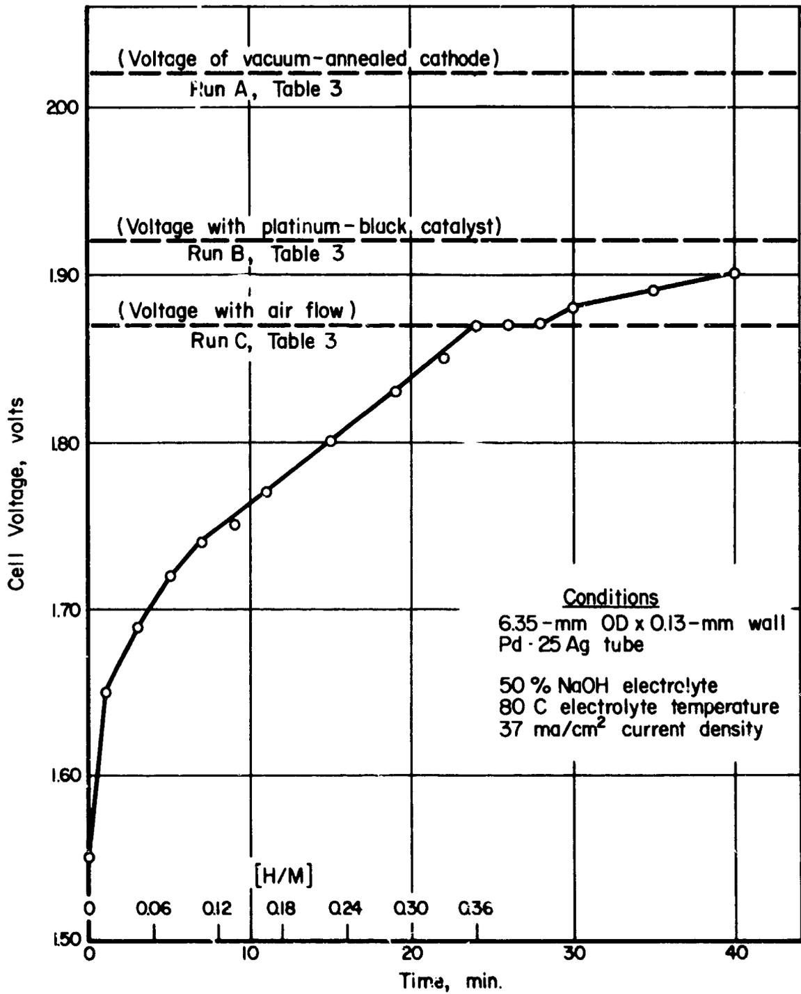
FIGURE 7. HYDROGEN ABSORPTION AND DIFFUSION EFFECTS ON CELL VOLTAGE
