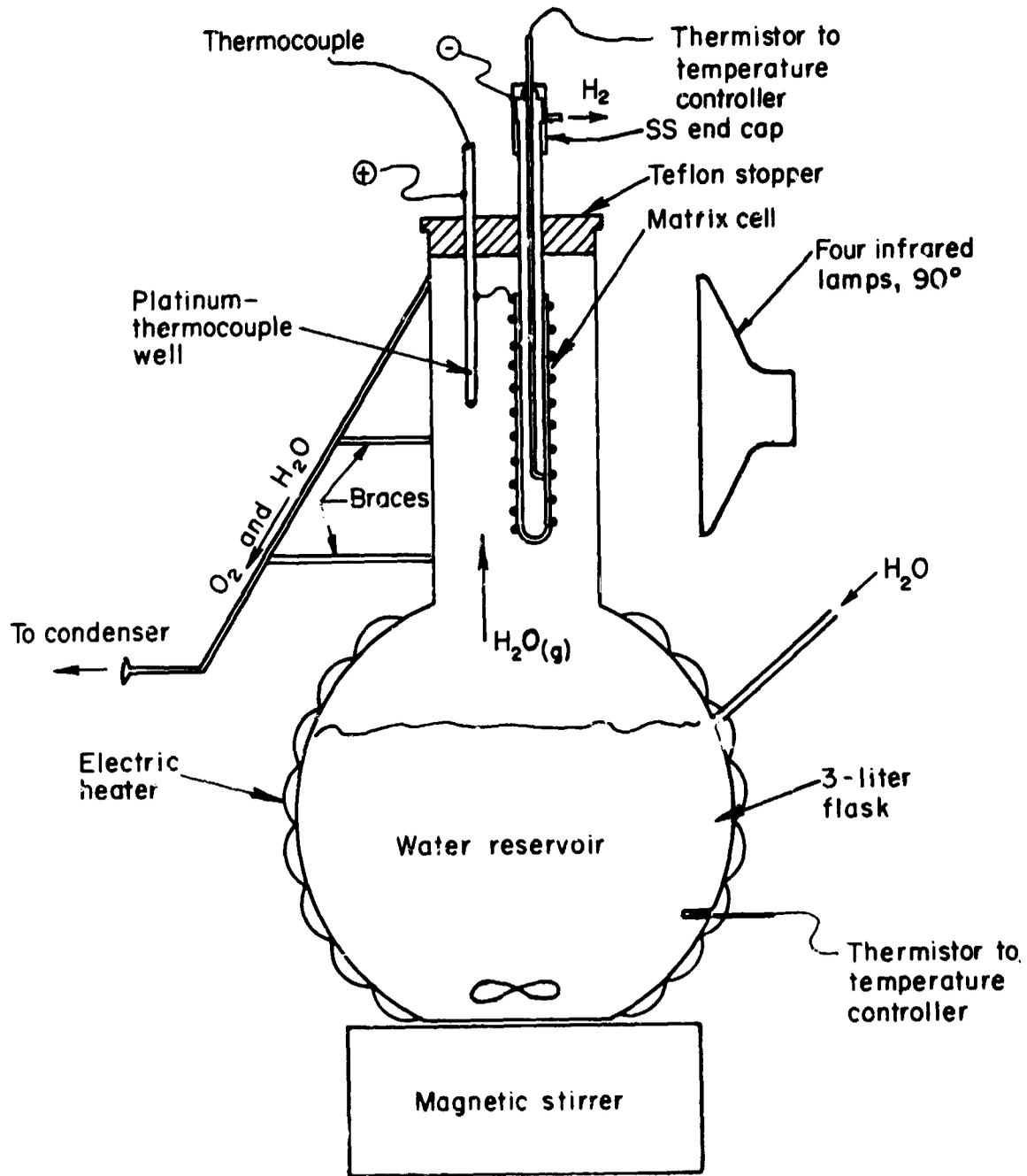
FIGURE 12. STATIC VAPOR-FEED EXPERIMENTAL UNIT
