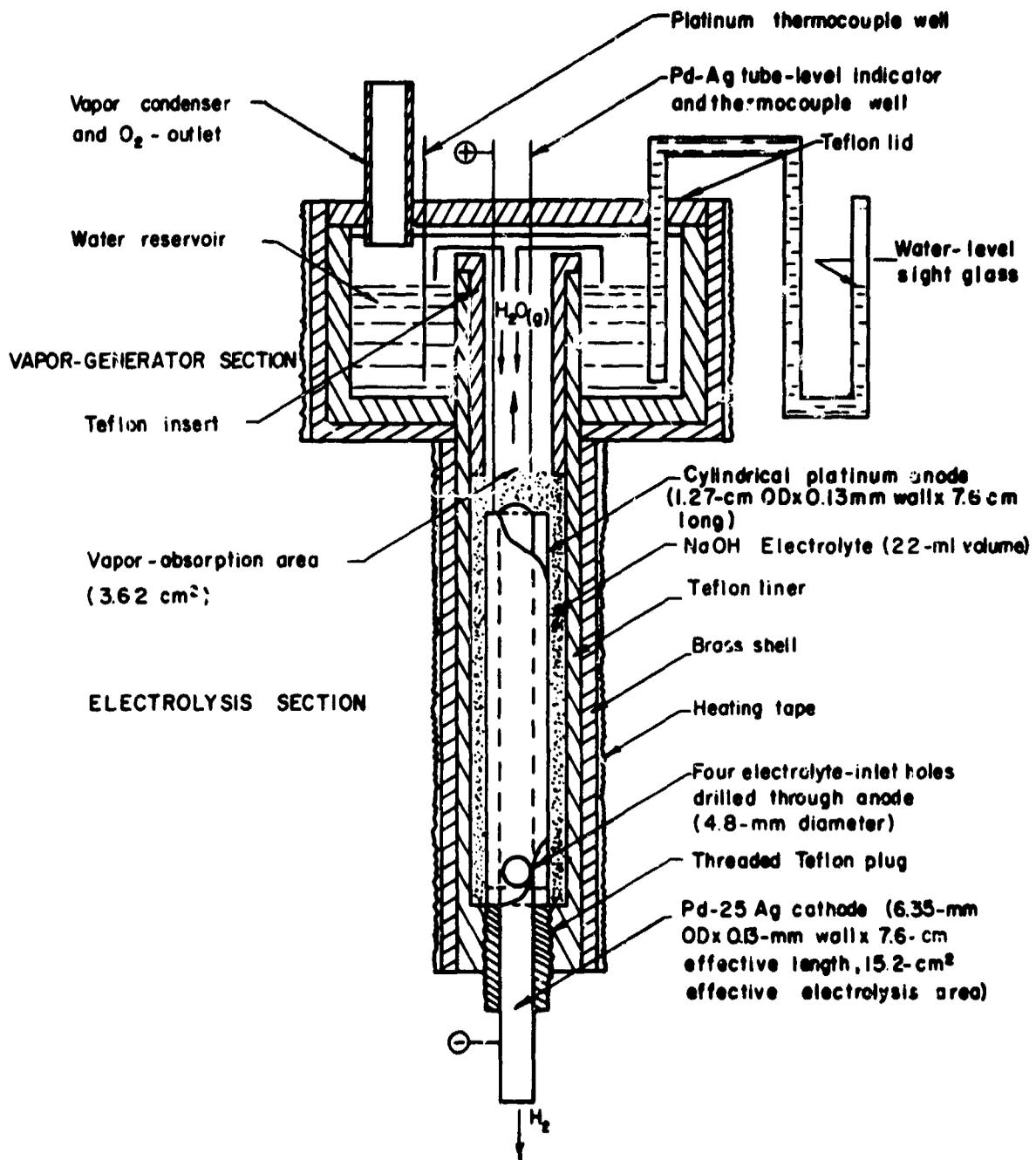
FIGURE 1. VAPOR-FEED FREE-ELECTROLYTE UNIT
