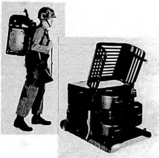
Figure 3. Mock-up of 200-watt unit. Hydrogen accumulator is at right of replaceable fuel canister. Inset indicates size and carrying position.
