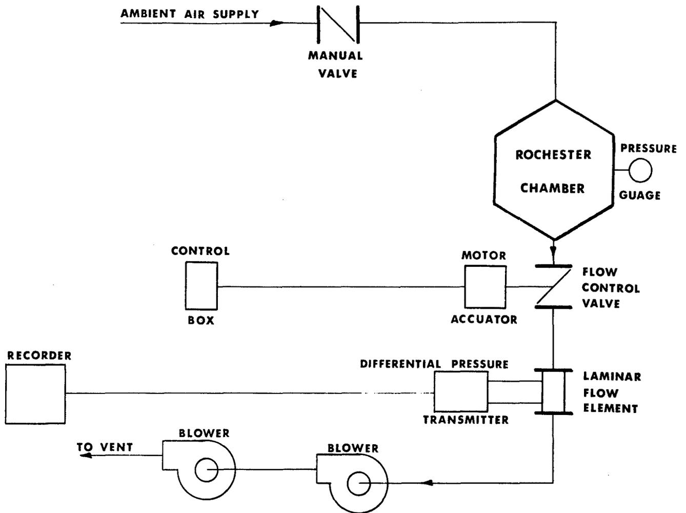
Figure 3. Modified Rochester Chamber Air Flow Control System
