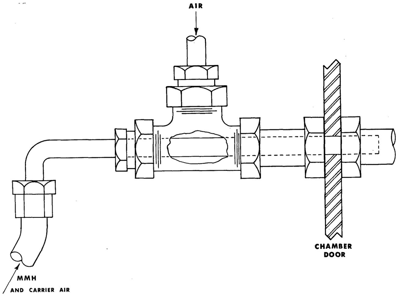
Figure 2. Apparatus for Final Dilution of MMH
