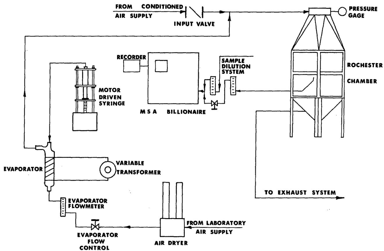
Figure 4. Rochester Chamber System for Toxicity Tests on Large Animals
