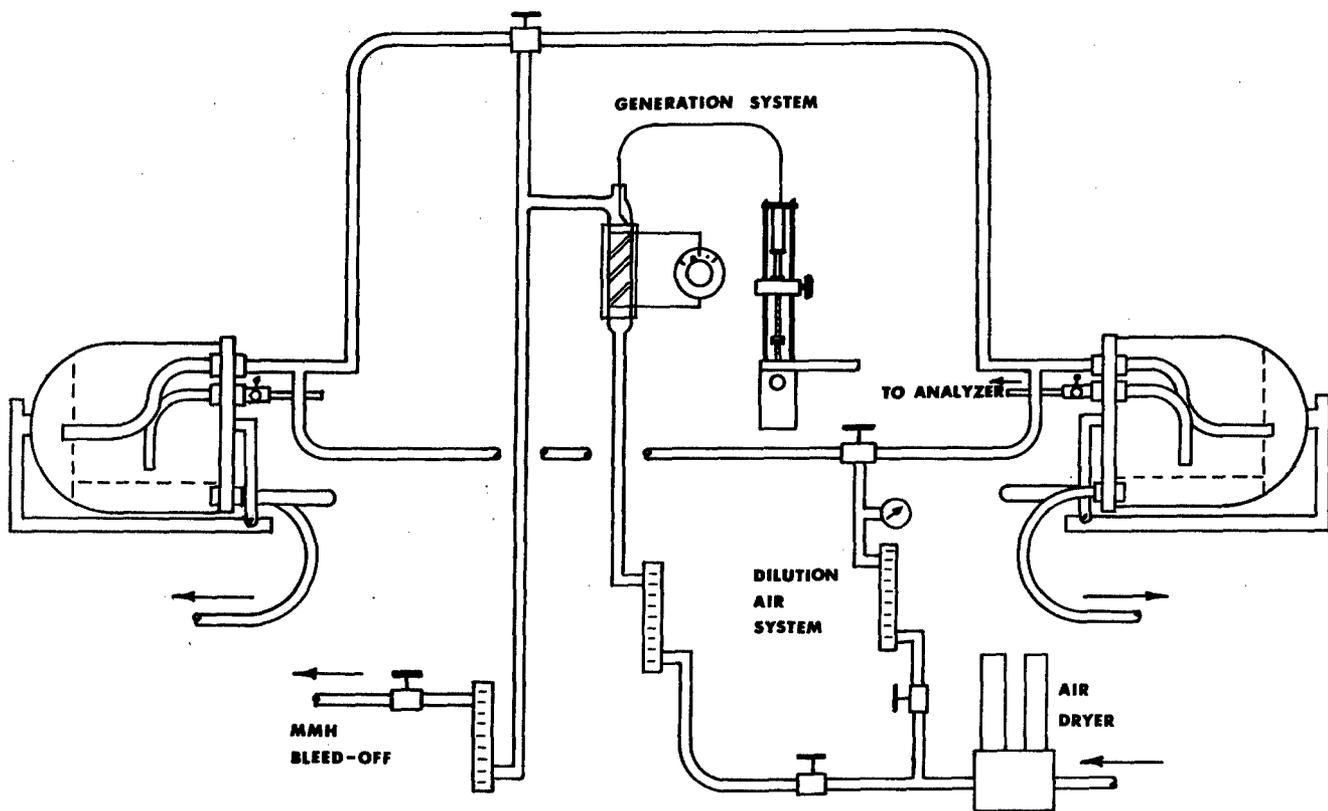
Figure 1. Rodent Inhalation Toxicity Exposure System
