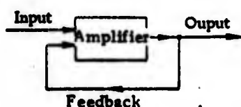
Fig. 7. 1. The principle of feedback in an amplifier.
