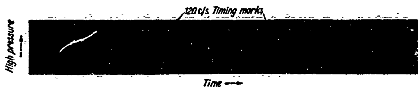
Figure 49. Development of high frequency unstable oscillations. (By courtesy of American Rocket Society and the General Electric Company of America)
