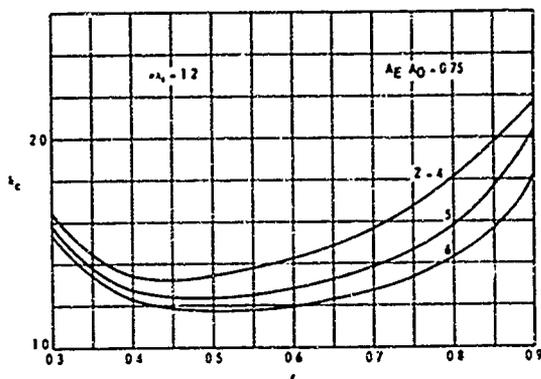
Fig. 11 Camber correction factor for  $\pi\lambda_i = 1.2$  and  $A_E/A_0 = 0.75$
