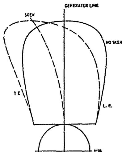
Fig. 4 Expanded blade outlines,  $A_E/A_0 = 0.75$ ,  $Z = 5$ , with symmetrical blade outline and 14-deg skew
