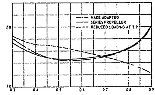
Fig. 21 Comparison of correction factors for ideal angle due to loading for three pitch distributions of Fig. 19
