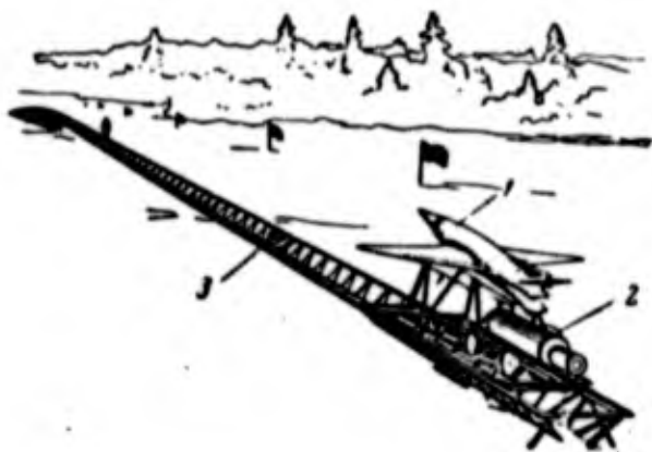
Fig. I.19. Soviet 212 winged rocket: 1 - winged rocket on catapult trolley; 2 - trolley booster; 3 - catapult rail.
