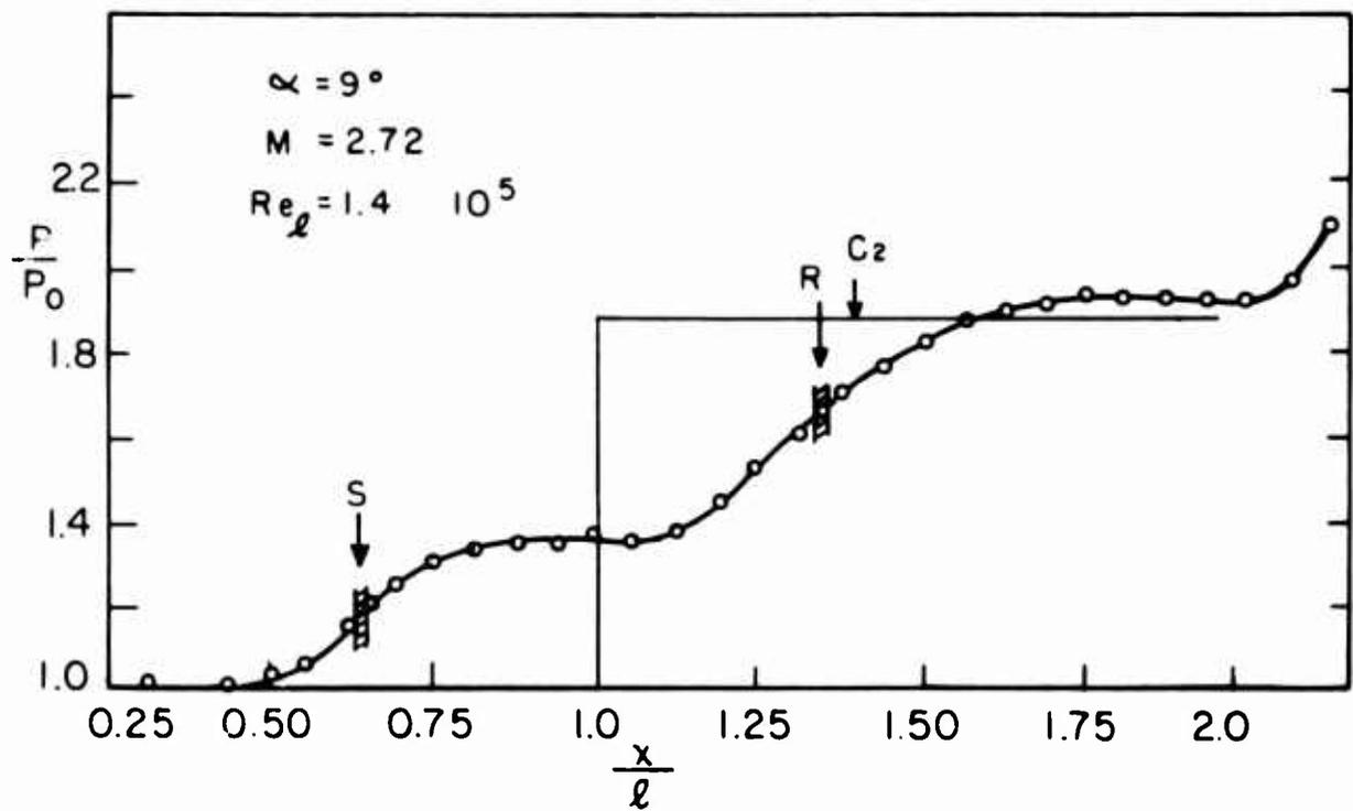
FIG. 25 PRESSURE DISTRIBUTION AND CRITICAL POINT
