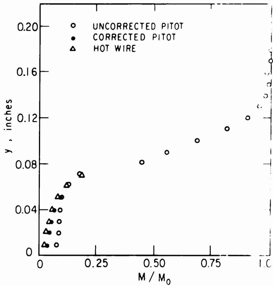
FIG. 8 UNCORRECTED AND CORRECTED PITOT DATA
