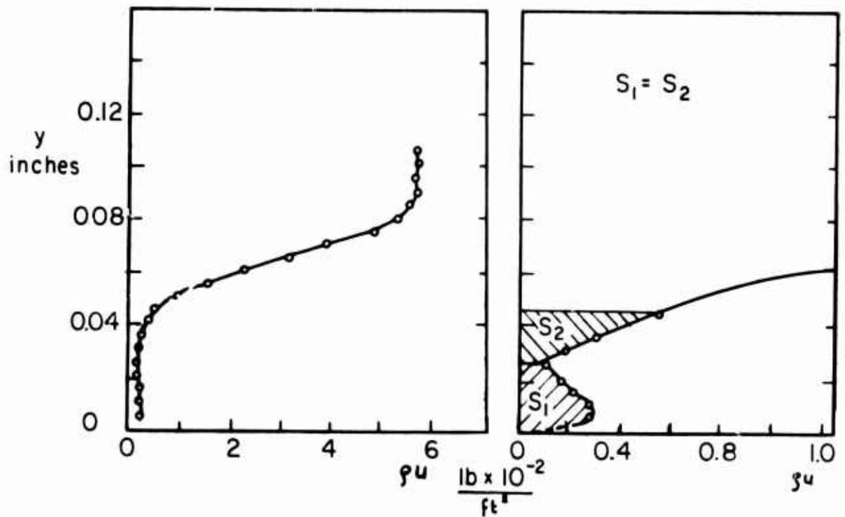
FIG. 22 GRAPHICAL DETERMINATION OF THE SEPARATING STREAMLINE
