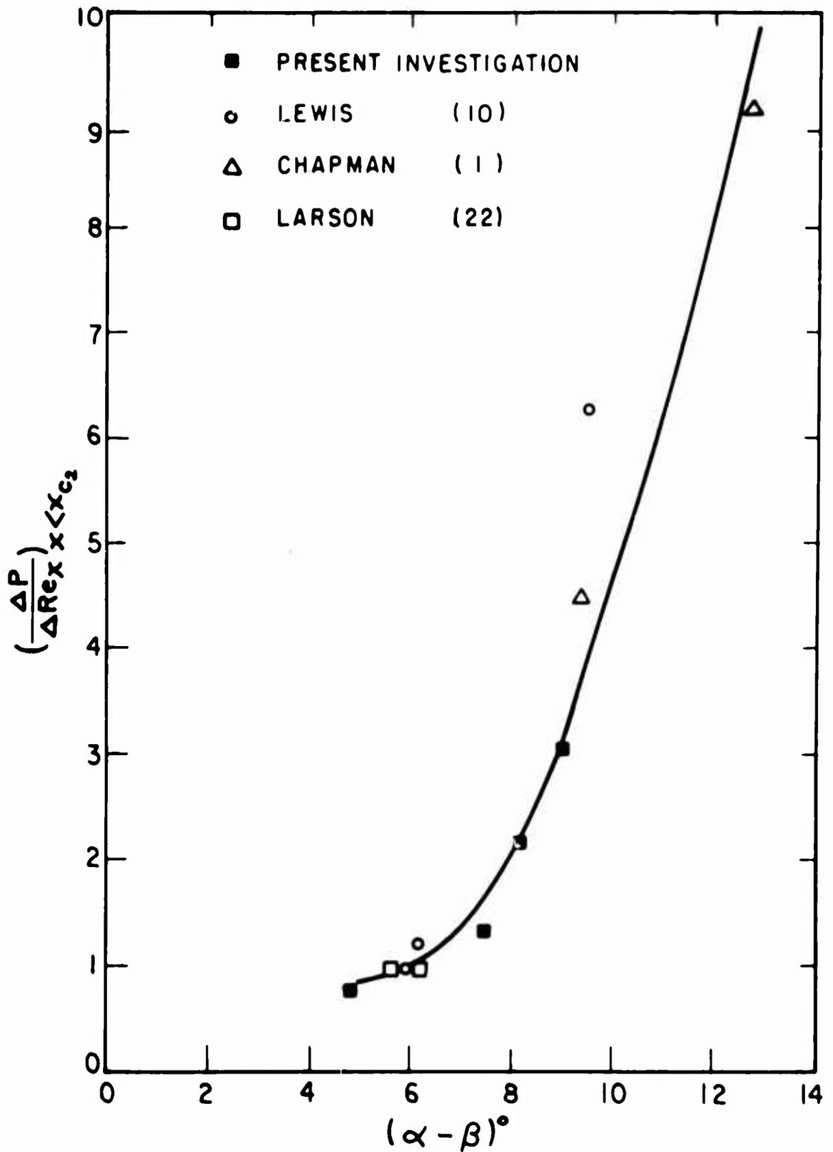
FIG. 32 VARIATION OF THE SLOPE OF THE PRESSURE DISTRIBUTION AHEAD OF THE CRITICAL POINT
