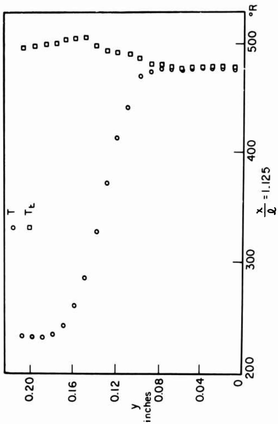
FIG. 13 TEMPERATURE PROFILES IN THE SEPARATED REGION
