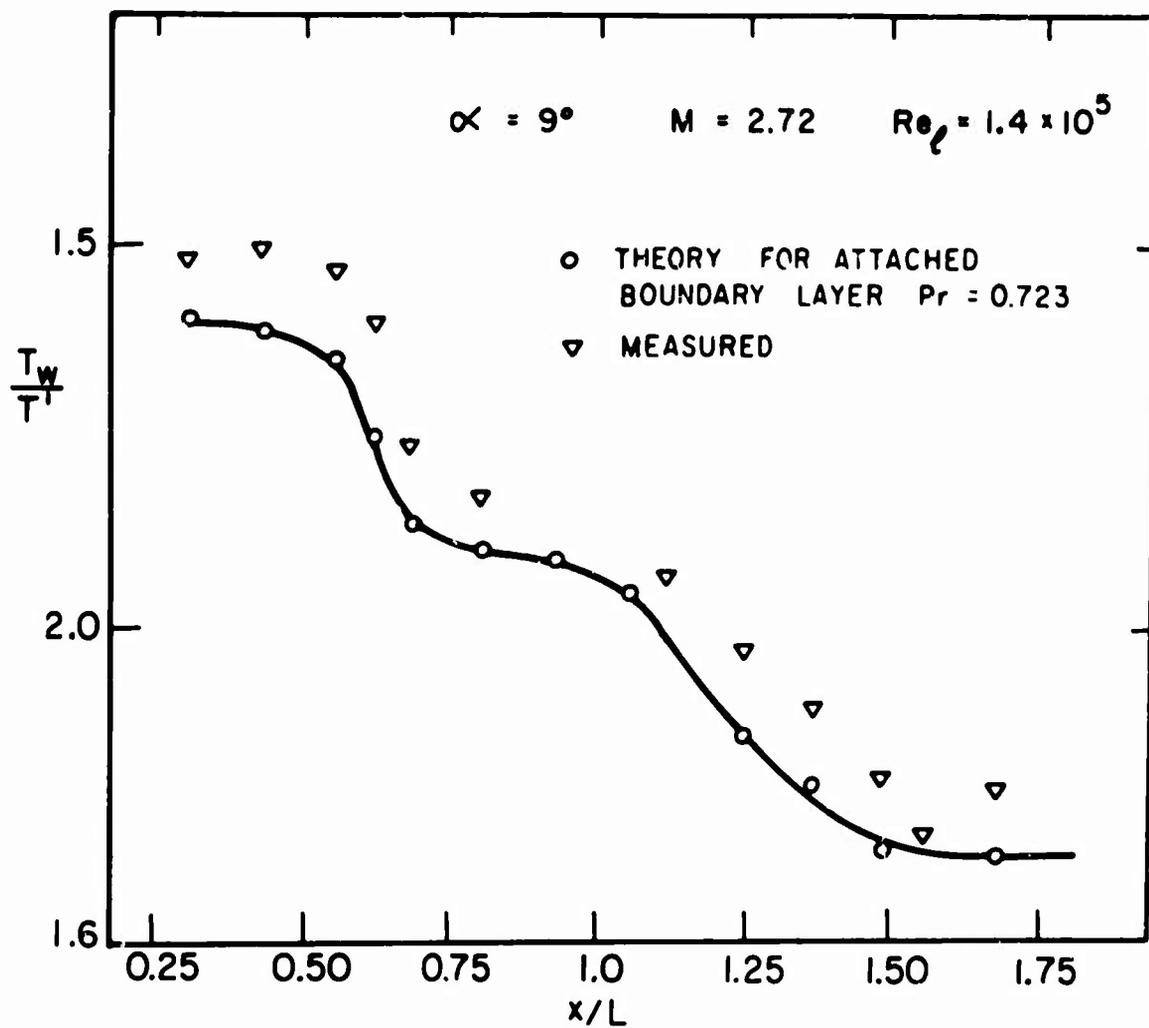
FIG. 18    COMPARISON OF  $\frac{T_w}{T_f}$  WITH THEORY
