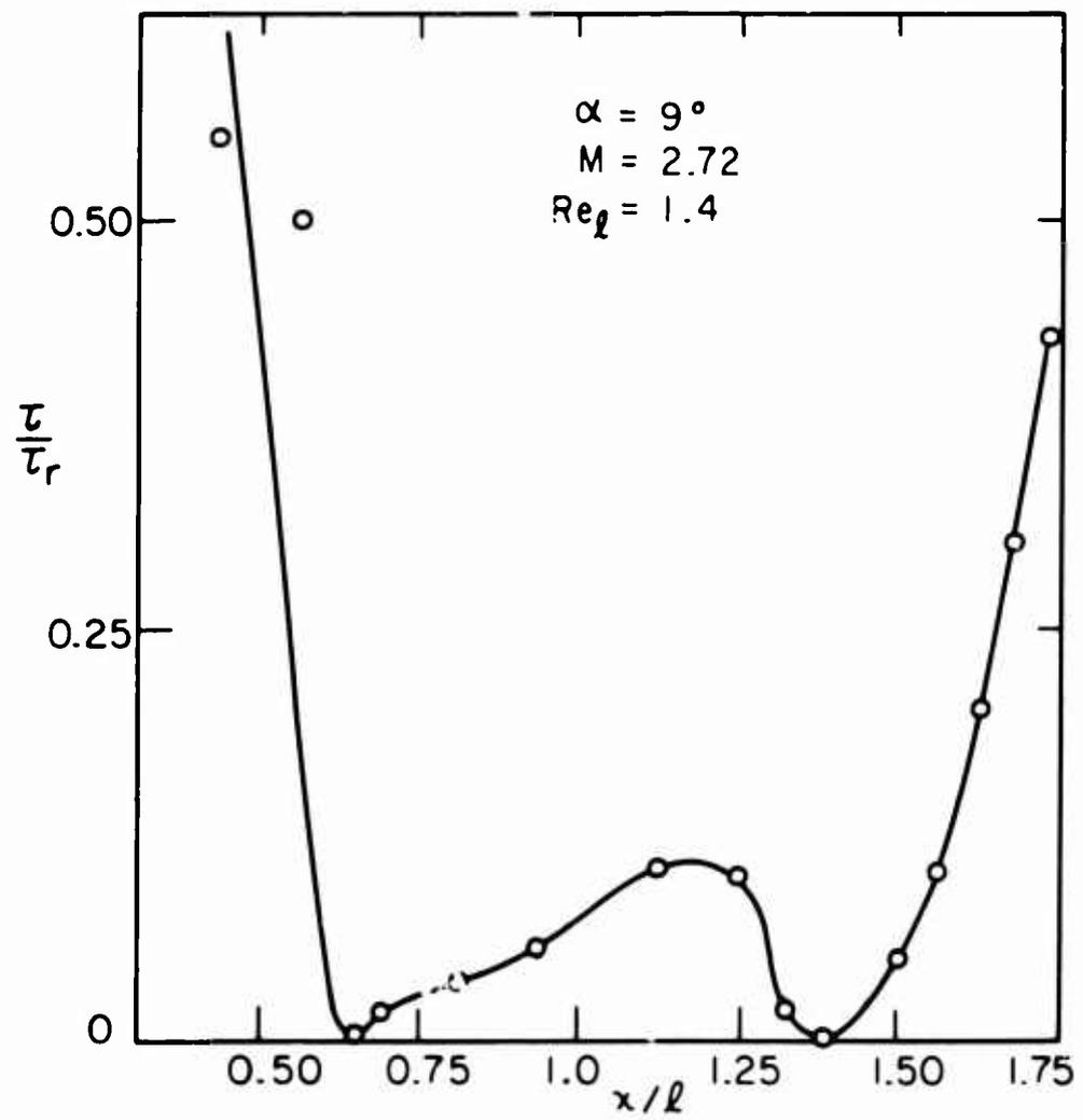
FIG. 20 SHEAR STRESS ALONG WALL AND  $u = 0$  LINE
