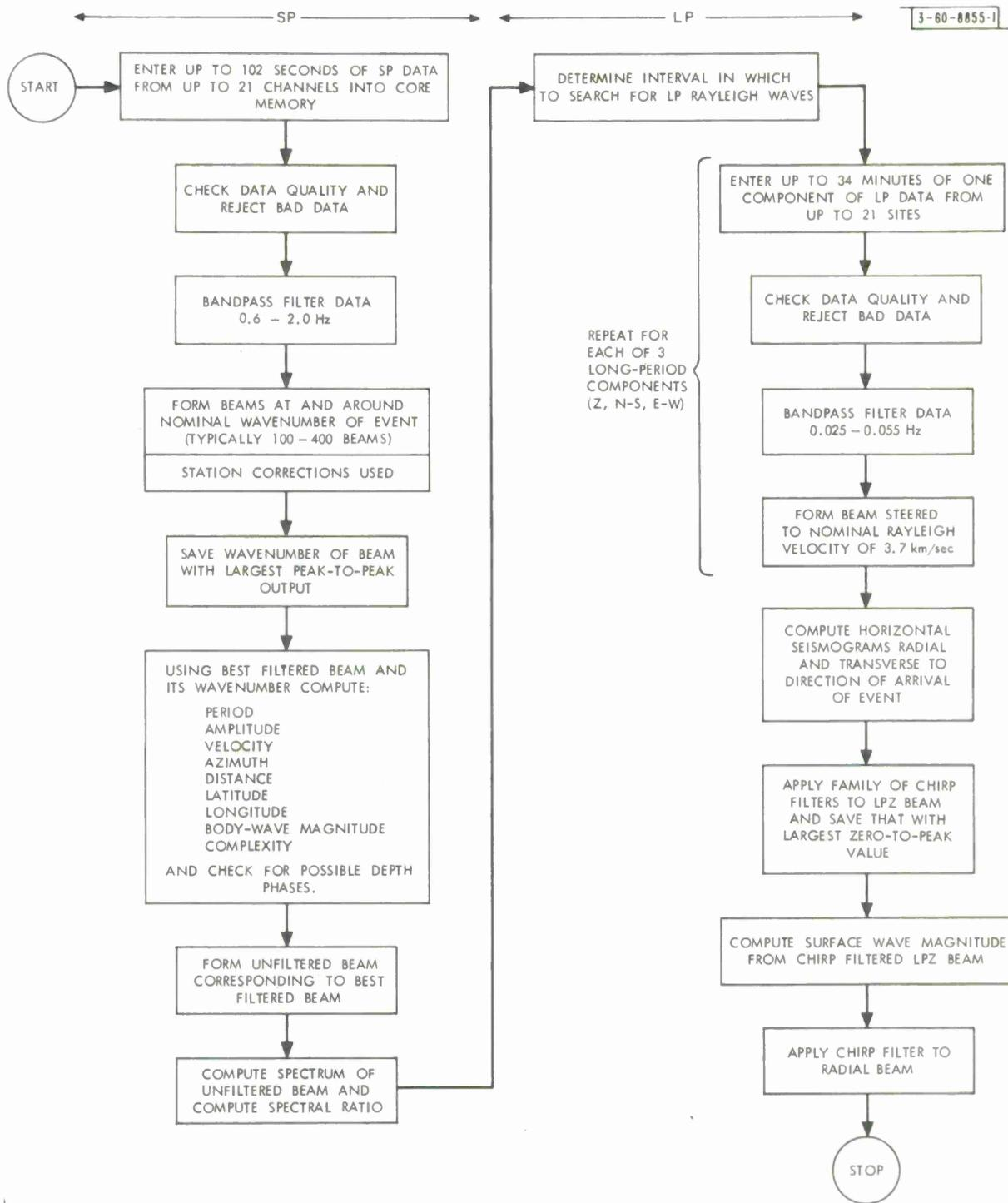
Fig. 3. Sequence of operations in SPLP program.
