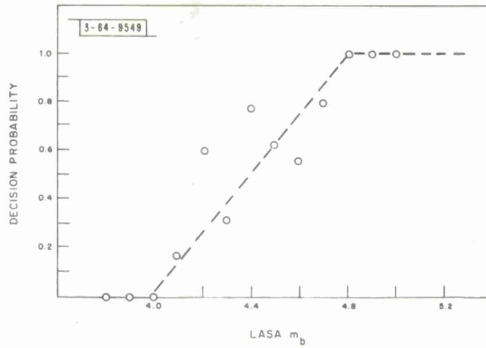
Fig. 21. Decision probability for modified spectral ratio test.
