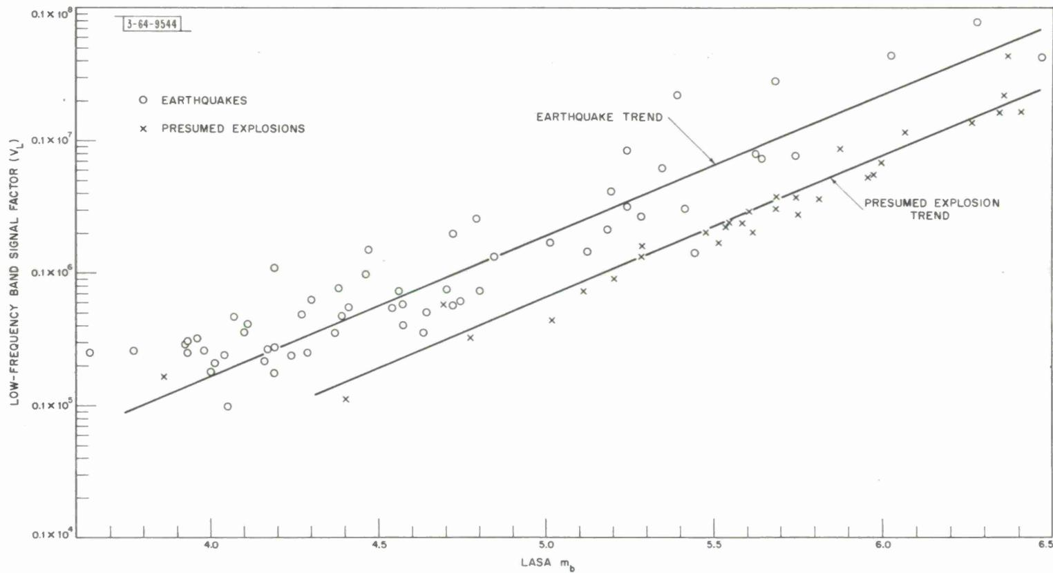
Fig. 14. Low-frequency band signal factor vs LASA  $m_b$ .
