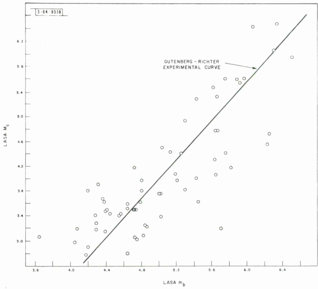
Fig. 4. LASA surface wave magnitude ( $M_s$ ) vs LASA body wave magnitude ( $m_b$ ) for earthquakes with detected surface waves (events with USCGS depth  $\geq 100$  km excluded).
