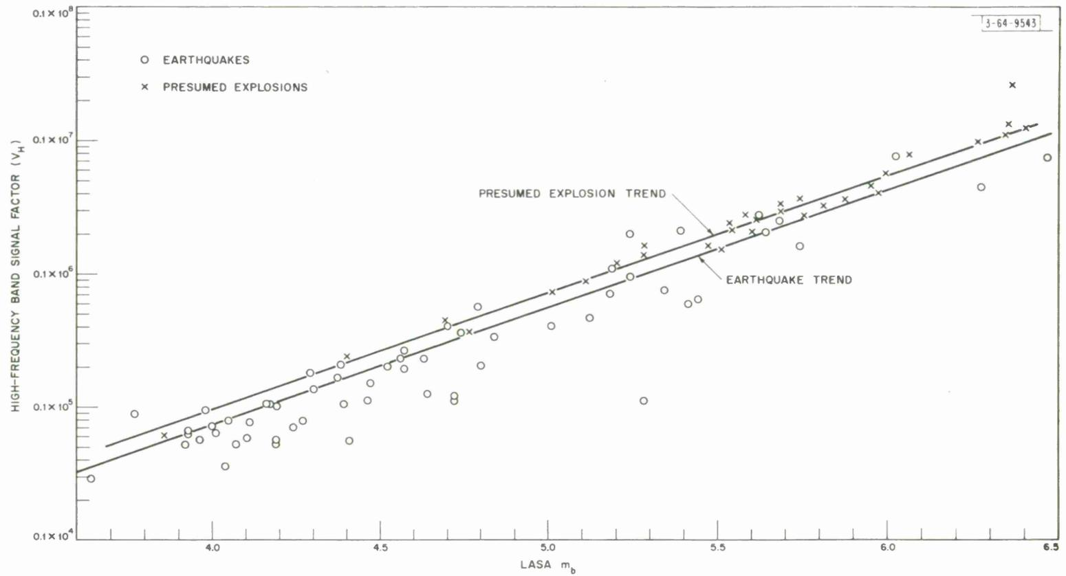
Fig. 13. High-frequency band signal factor vs LASA  $m_b$ .
