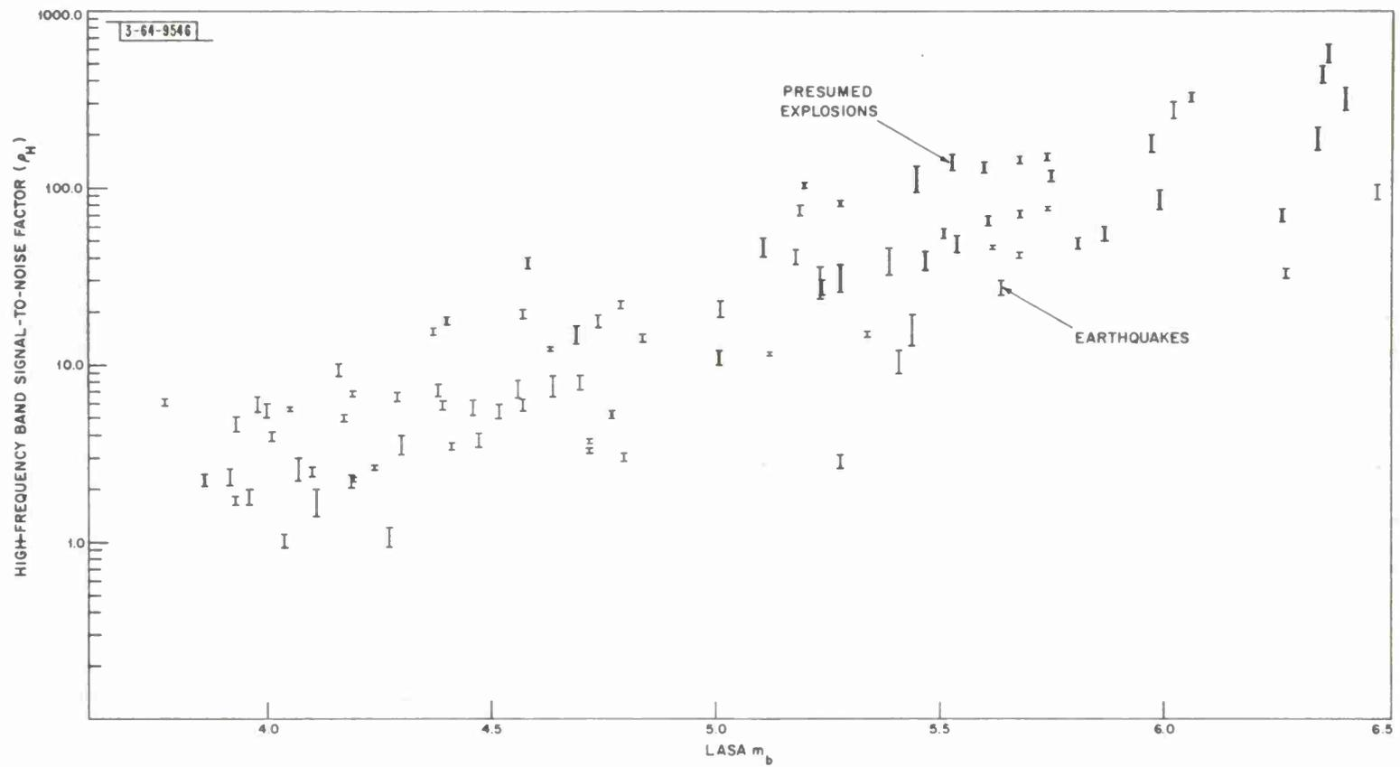
Fig. 16. High-frequency band signal-to-noise factor vs LASA  $m_b$ .
