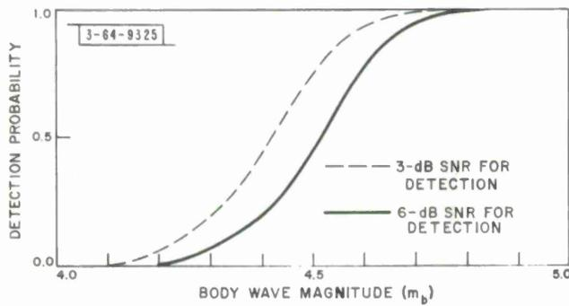
Fig. 8. Surface wave detection probability inferred from noise observations.
