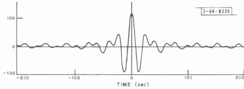
Fig. 27. Long period band-pass filter impulse response.
