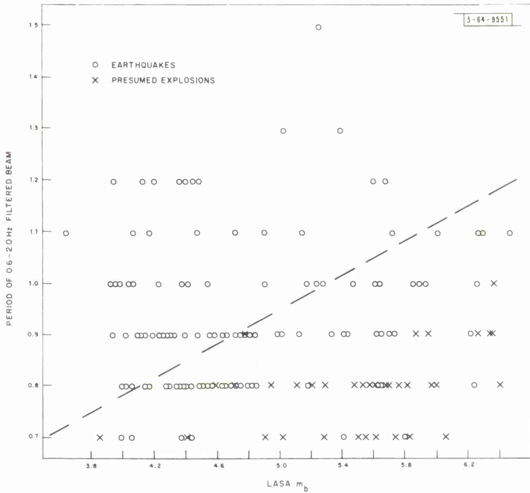
Fig. 23. Period of 0.6 - 2.0 Hz filtered beam vs LASA  $m_b$  (events with USCGS depth  $\geq 100$  km excluded).
