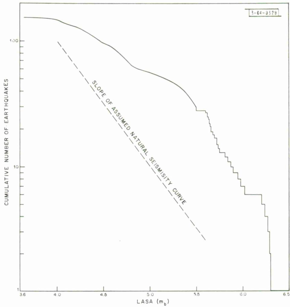
Fig. 1. Body wave magnitude distribution of earthquakes in experiment.
