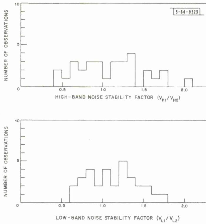
Fig. 18. Stability study for signal-to-noise factor test.
