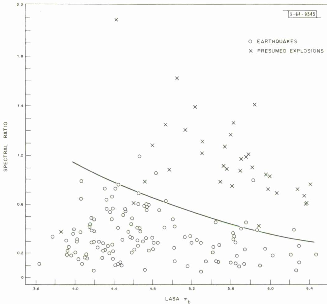
Fig. 15. Spectral ratio vs LASA  $m_b$  (events with USCGS depth  $\geq 100$  km excluded).
