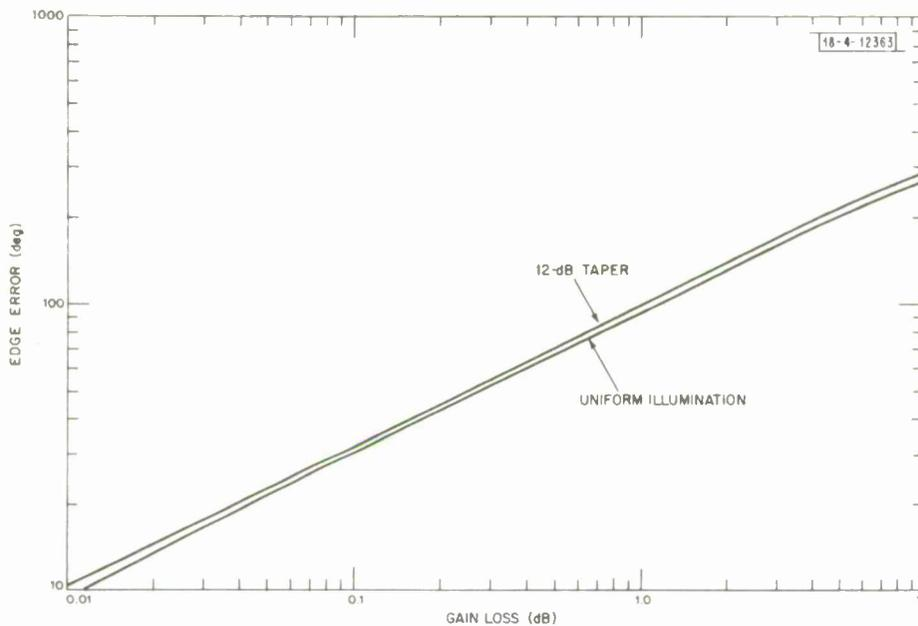
Fig. D-3. Loss in gain of circular aperture because of defocusing, for uniform and tapered illuminations. Assumed illumination varies as  $\exp[-\alpha y^2 - j\beta y^2]$ . (This figure was supplied by Dr. John Ruze).
