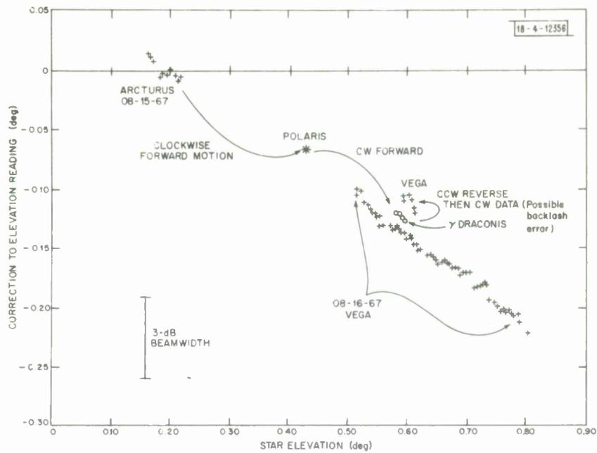
Fig. 8. Correction needed to make elevation encoder reading agree with calculated elevations of some stars, on two nights. Calculated elevations included no allowance for refraction.
