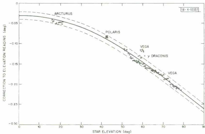
Fig. 9. Correction needed to make elevation encoder reading agree with calculated elevations of some stars, when calculations included allowance for refraction. Observations are same as those in Fig. 8. Of the correction at zero elevation, about 0.02 deg was caused by using traditional and incorrect value for elevation of Billerica transmitter used as reference. Solid curve is constructed analytically from  $-0.23 \cos E_l$ . Dashed lines are  $\pm 0.01$  deg from solid one.
