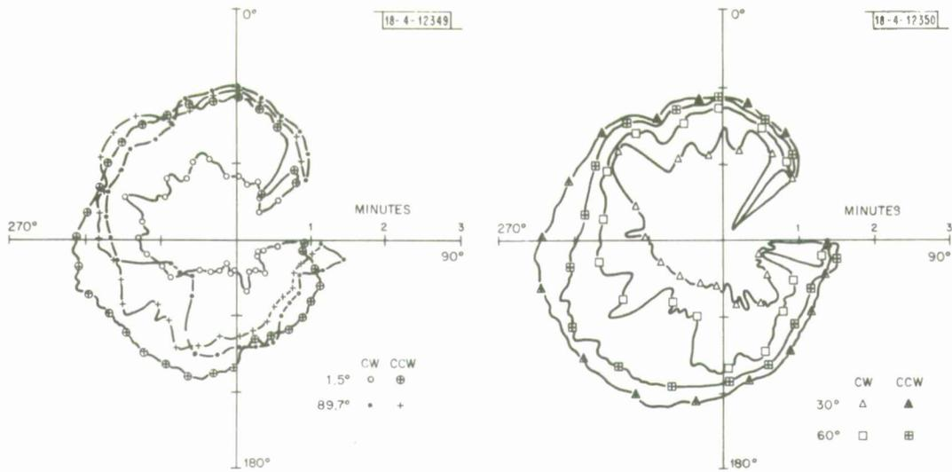
(a) Antenna elevations 1.5 and 89.9 deg.
