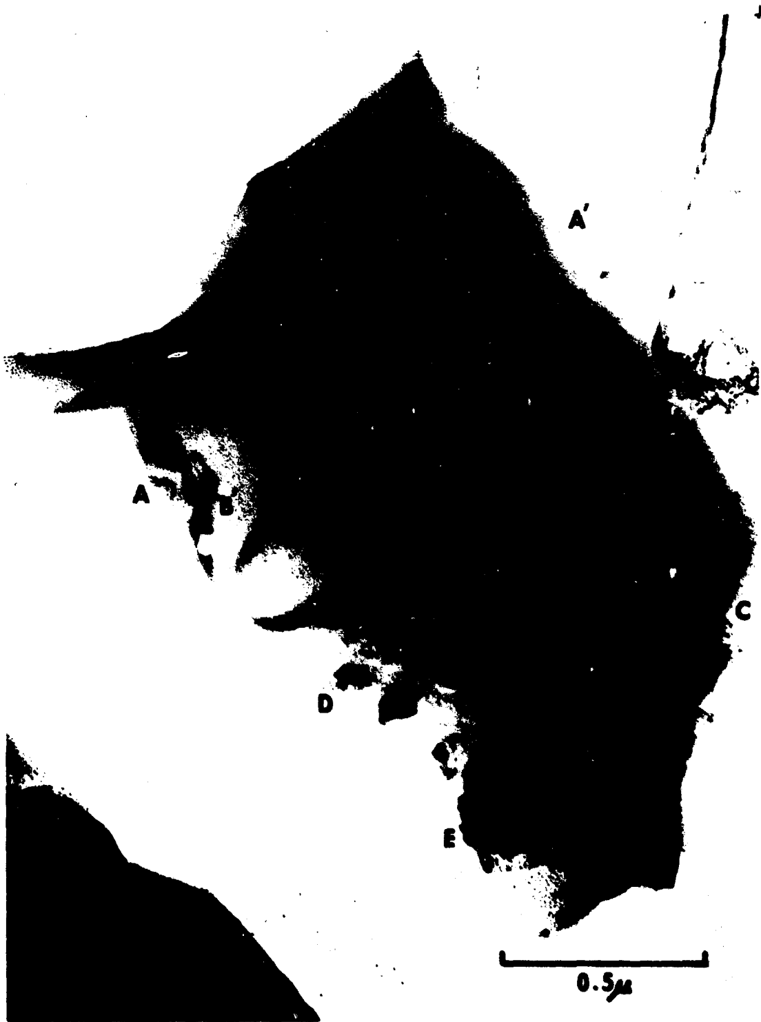
Figure 27. Additional tilting of the fragment (for two beam diffraction) reduces contrast for dislocations previously imaged, but brings a very densely populated region along C-E into strong contrast, X80,000. Extracted fragment on plastic-carbon replica [D1-1823].
