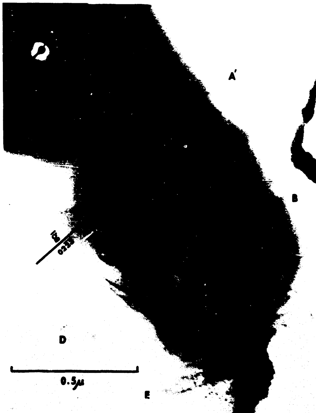
Figure 29. Additional information about dislocations is provided by different contrast conditions available from another orientation selected to yield two beam diffraction, X120,000. Extracted fragment on plastic-carbon replica [DI-1847; inset 1845]. The \bar{g} vector (arrow in inset diffraction pattern) describes crystallographic relationships between transmitted beam and the strong diffracted beam responsible for these dislocation contrast effects. Diffraction pattern also identifies this picture plane as the (2\bar{1}10) prism plane.
