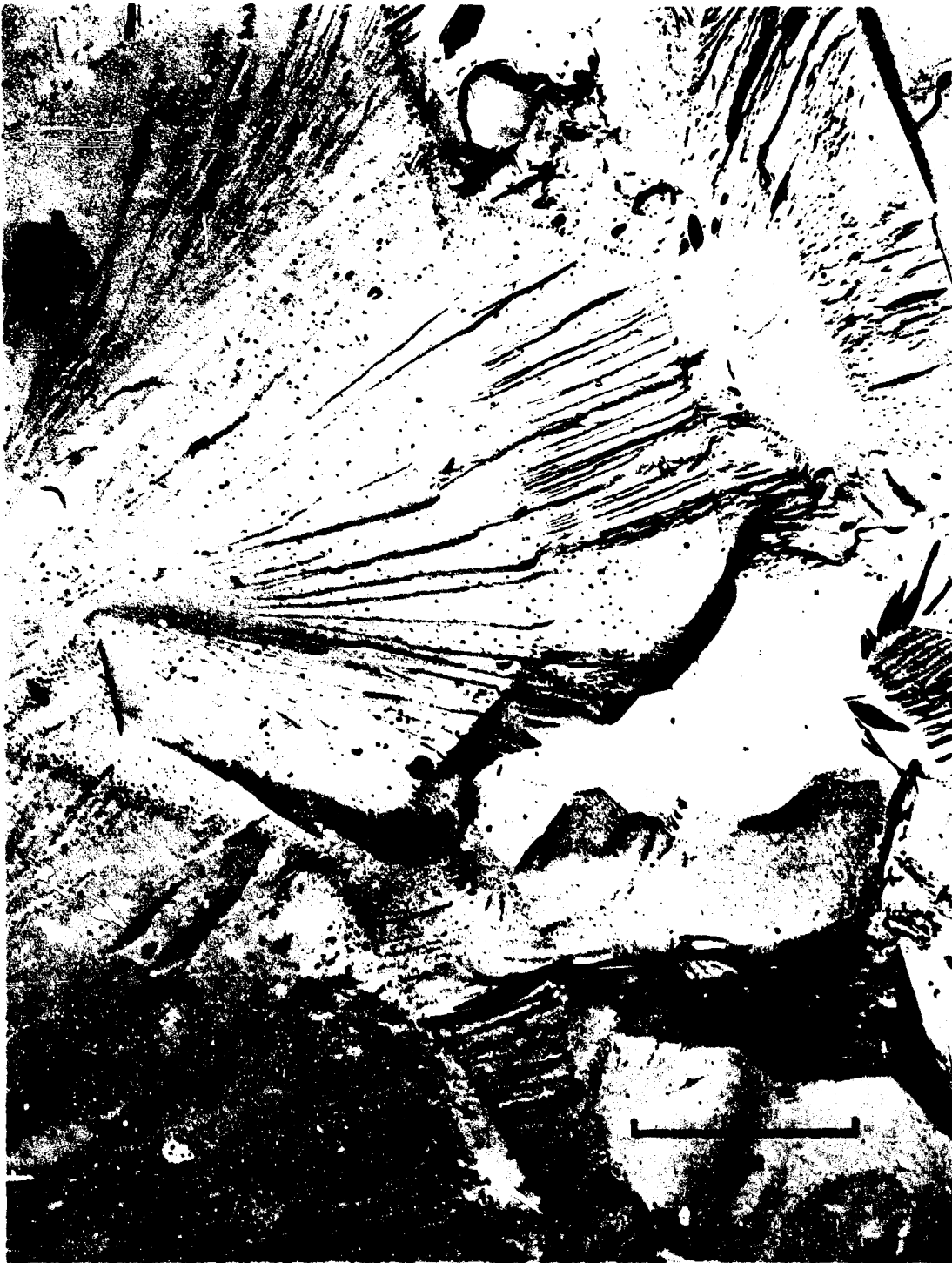
Figure 13. Complex fractography of conoid shear surface in ballistically damaged polycrystalline alumina tile, X6,900. Two-stage plastic-carbon replica, Pt-shadowed at 30° [D1-386].
