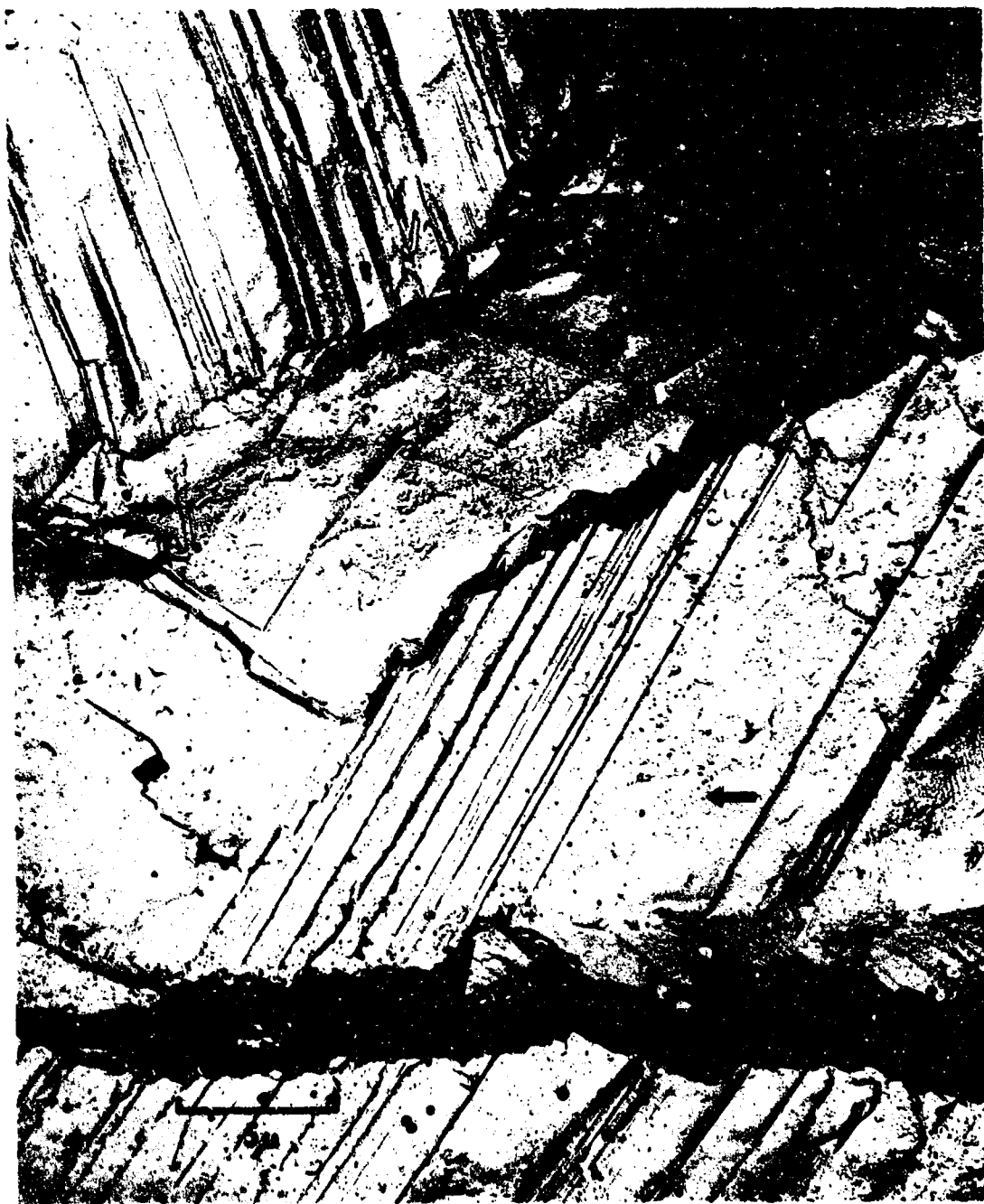
Figure 9. Fine textures associated with cleavage in ballistically damaged sapphire, X4,800.
