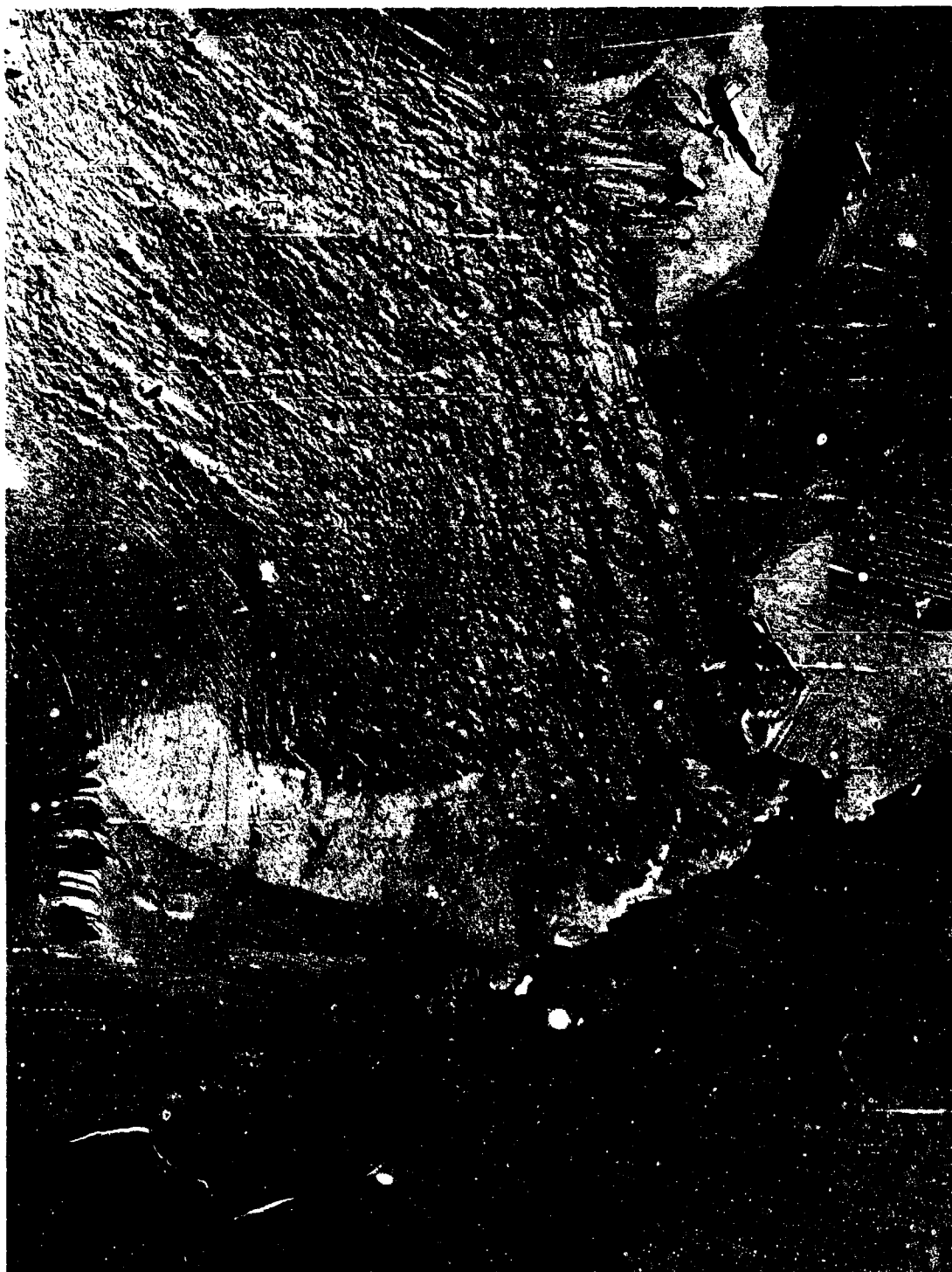
Figure 18. Fracture textures on transverse secondary crack in ballistically damaged polycrystalline alumina tile, X9,600. Two stage plastic-carbon replica, Pt-shadowed at 30° [SD5-402].
