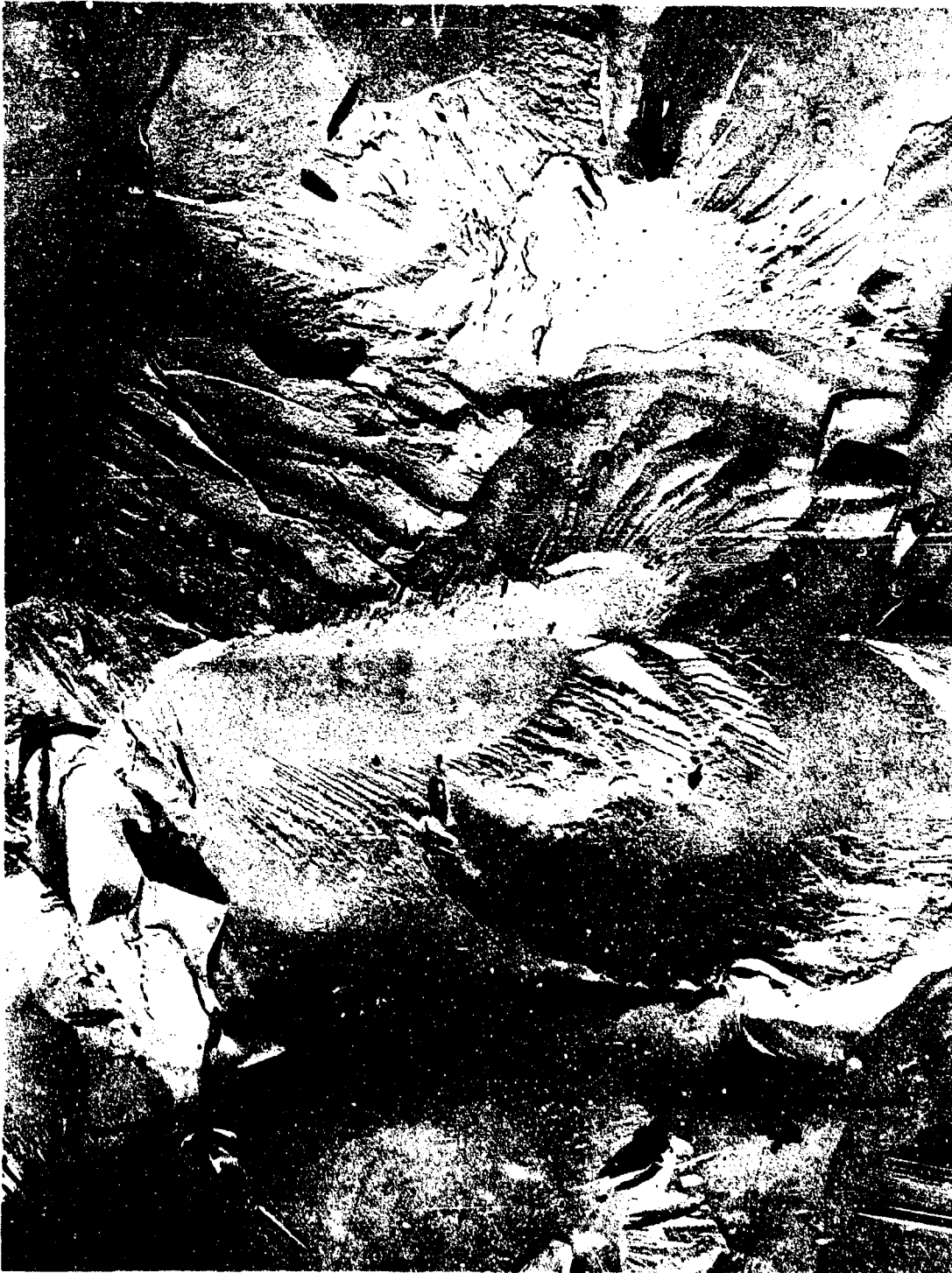
Figure 16. Fracture fragments and transition from intergranular separation to transgranular fracture on a smoothly textured portion of a radial crack in ballistically damaged polycrystalline alumina tile, X9,600. Two stage plastic-carbon replica, Pt-shadowed at 30° [SD4-378].
