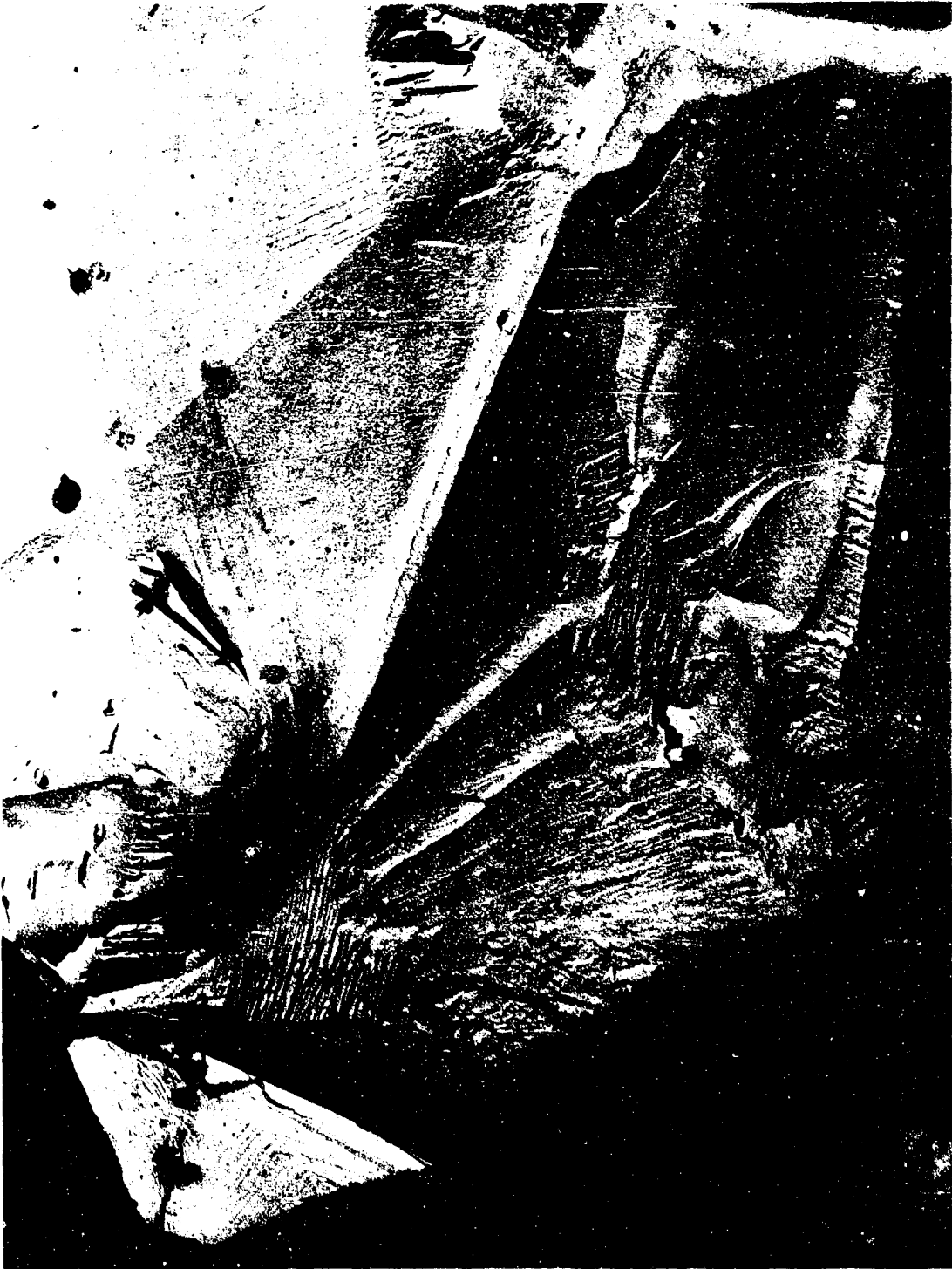
Figure 17. Transition from intergranular separation to transgranular fracture along grain edge junction on a radial crack surface in ballistically damaged polycrystalline alumina tile, X9,600. Two stage plastic-carbon replica, Pt-shadowed at 30° [SD4-379].
