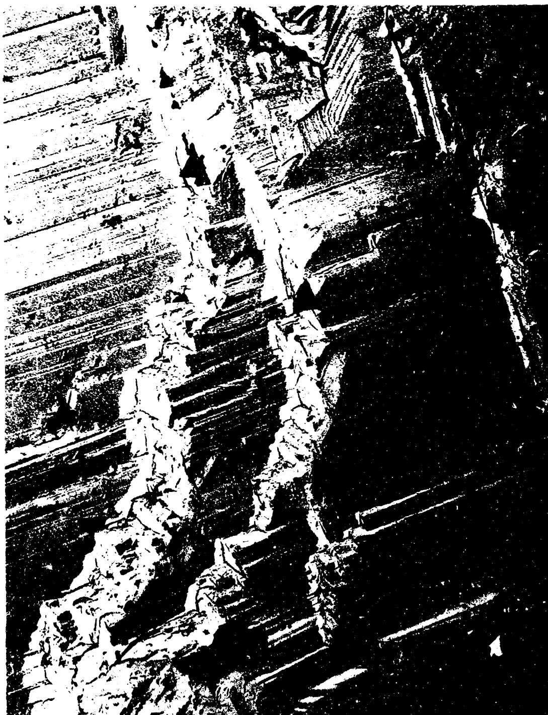
Figure 10. Cleavage fracture across previously sheared regions in ballistically damaged sapphire, X23,300.
