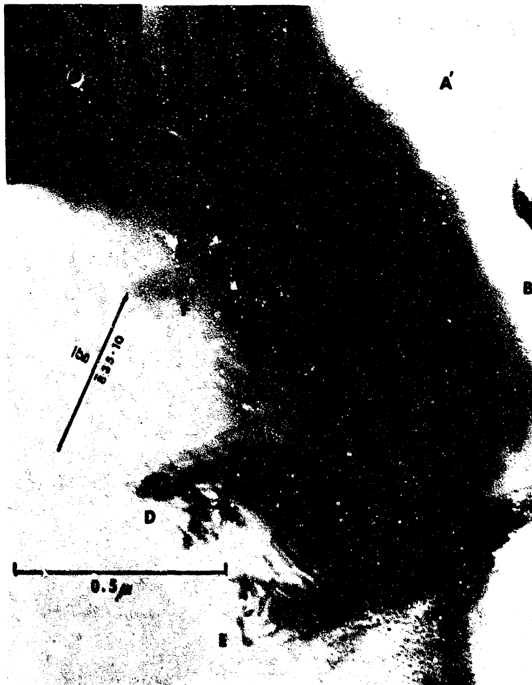
Figure 30. Bright field image with two beam diffraction for (03\bar{3}3) orientation in fragment from conoid shear surface in ballistically damaged polycrystalline alumina tile, X120,000. Extracted fragment on plastic-carbon replica [D1-1836; inset 1834]. Compare with different contrast conditions in Figs. 28 and 29.
