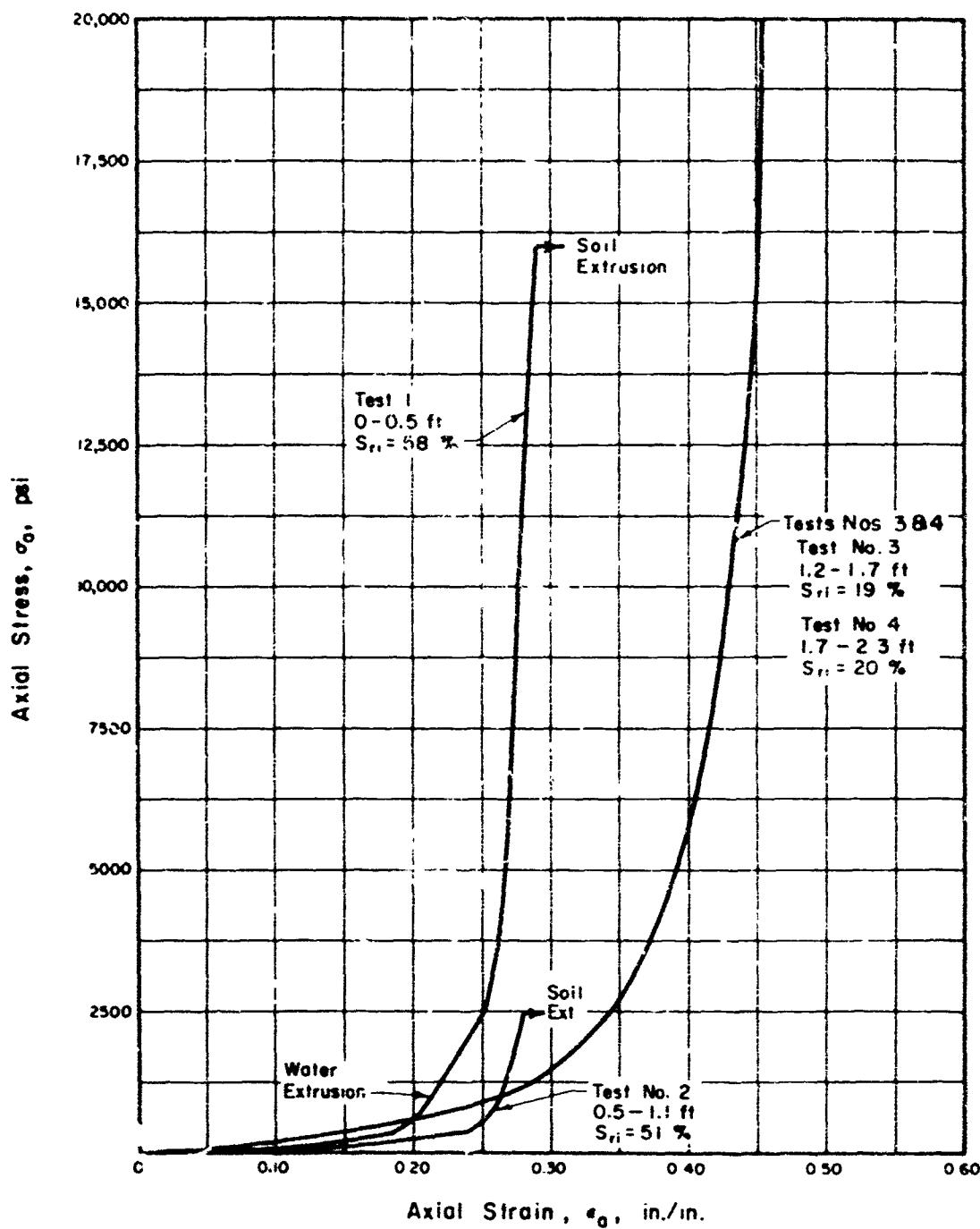
Fig. 5. Summary of stress-strain curves for the undisturbed samples of silty clay
