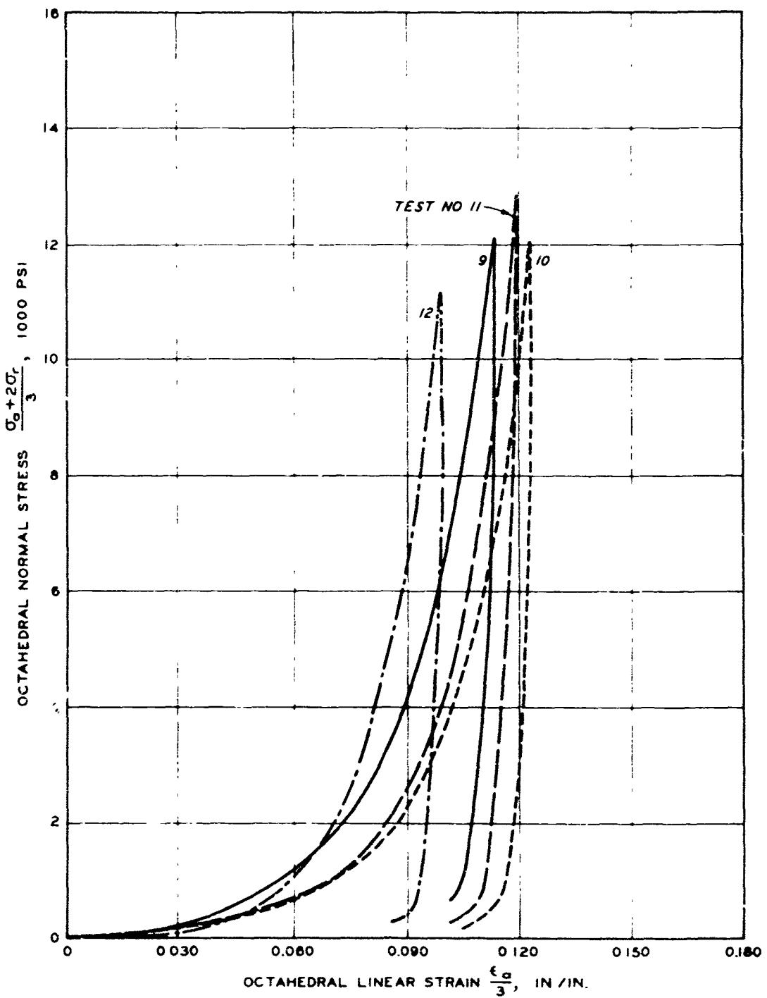
Fig. F3 Octahedral normal stress versus octahedral linear strain
