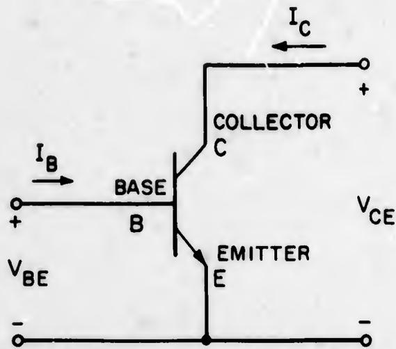
FIG.3.29 SCHEMATIC SYMBOL OF A TRANSISTOR
