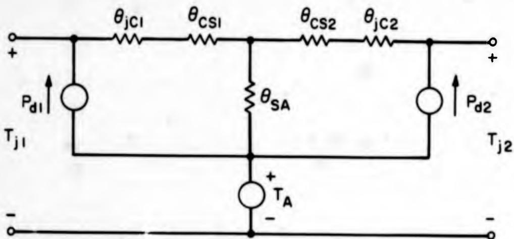
FIG. 3.25 TWO DEVICE CONVECTION COOLED STATIC THERMAL CIRCUIT MODEL
