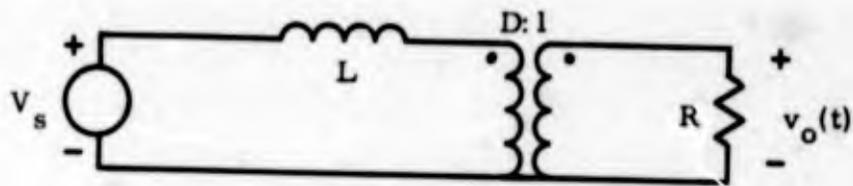
a. Proposed Model of Step-Up Circuit
