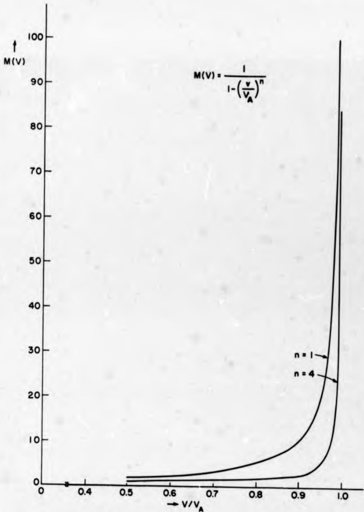
FIG. 3.22 AVALANCHE MULTIPLICATION FACTOR VERSUS NORMALIZED VOLTAGE.
