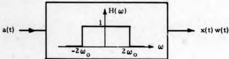
b. Isolation of Low-Frequency Components of  $a(t)$
