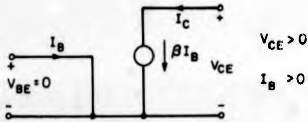
a. CURRENT CONTROLLED CURRENT SOURCE MODEL OF A TRANSISTOR
