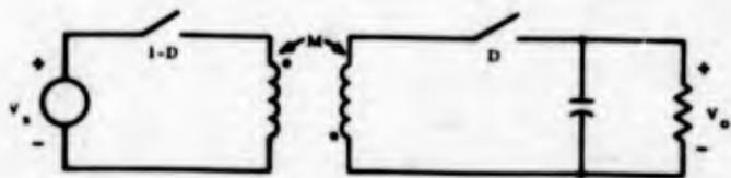
d. Modeling the transformer and inductor as two unity-coupled inductors.
