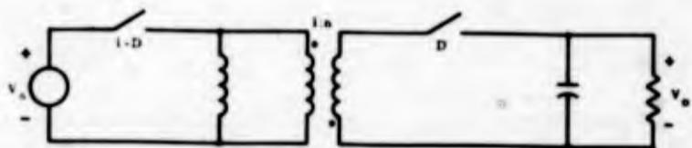
c. Reflecting the switch and the capacitor to the secondary.
