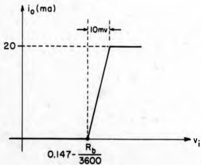
FIGURE 12.44 TRANSFER CHARACTERISTIC OF ERROR AMPLIFIER
