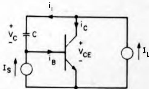
FIG. 3.48b CIRCUIT FOR INVESTIGATING EFFECTS OF COLLECTOR CAPACITY
