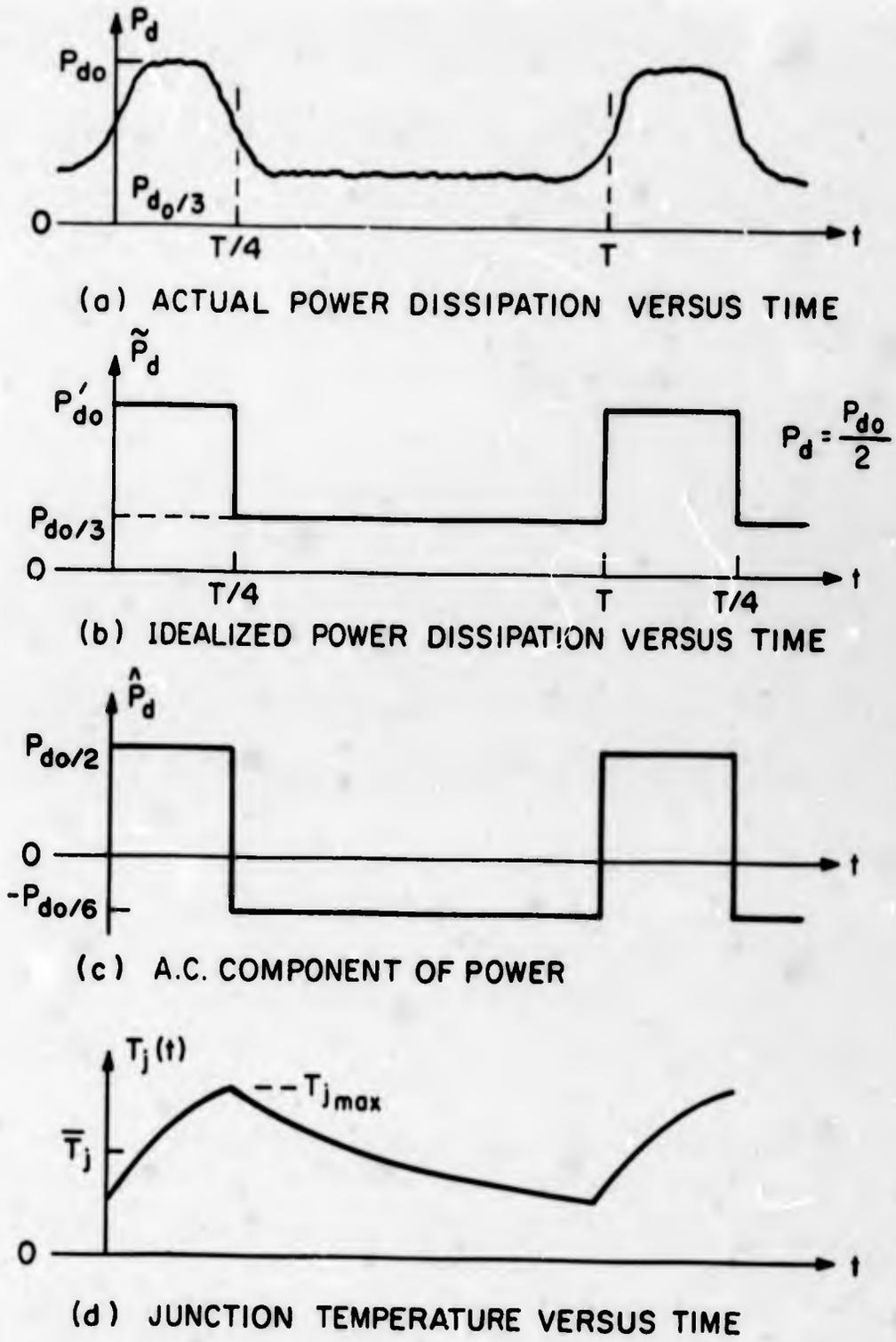
FIG. 3.27 CALCULATION OF MAXIMUM JUNCTION TEMPERATURE
