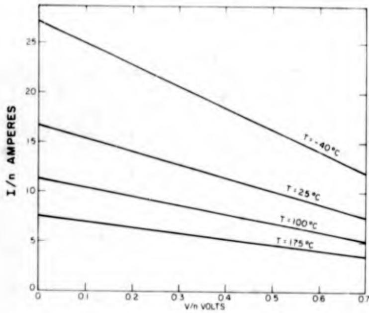
FIG. 3.10. NORMALIZED FORWARD CURRENT TEMPERATURE COEFFICIENT VERSUS  $\frac{V}{n}$  WITH TEMPERATURE AS A PARAMETER
