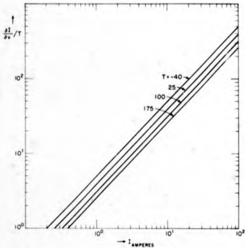
FIG. 3.11. DIODE FORWARD INCREMENTAL CONDUCTANCE VERSUS CURRENT WITH TEMPERATURE AS A PARAMETER
