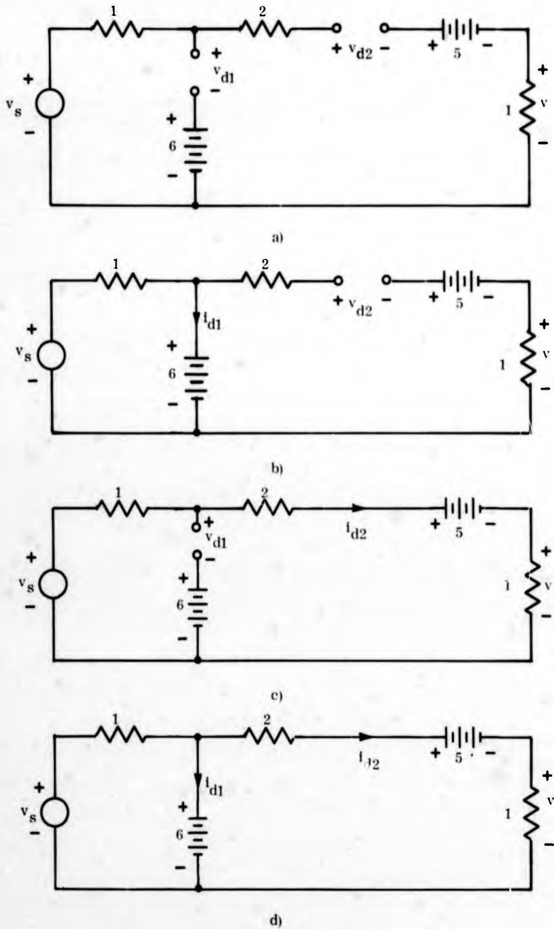
FIG. 10.19 NONLINEAR NETWORK WITH ASSUMED DIODE STATES
