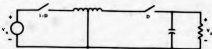
e. Modeling the coupled inductors as a tapped inductor if there is a common ground.
