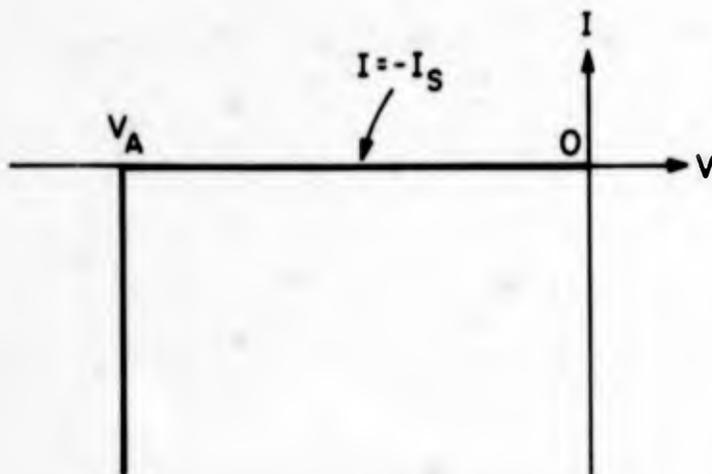
FIG. 3.23 THRESHOLD BREAKDOWN V-I
