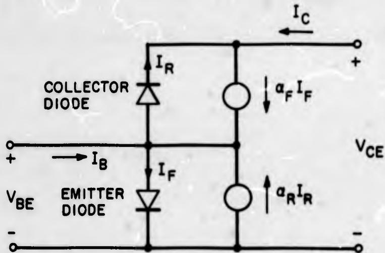
FIG.3.30 EBERS - MOLL TRANSISTOR MODEL
