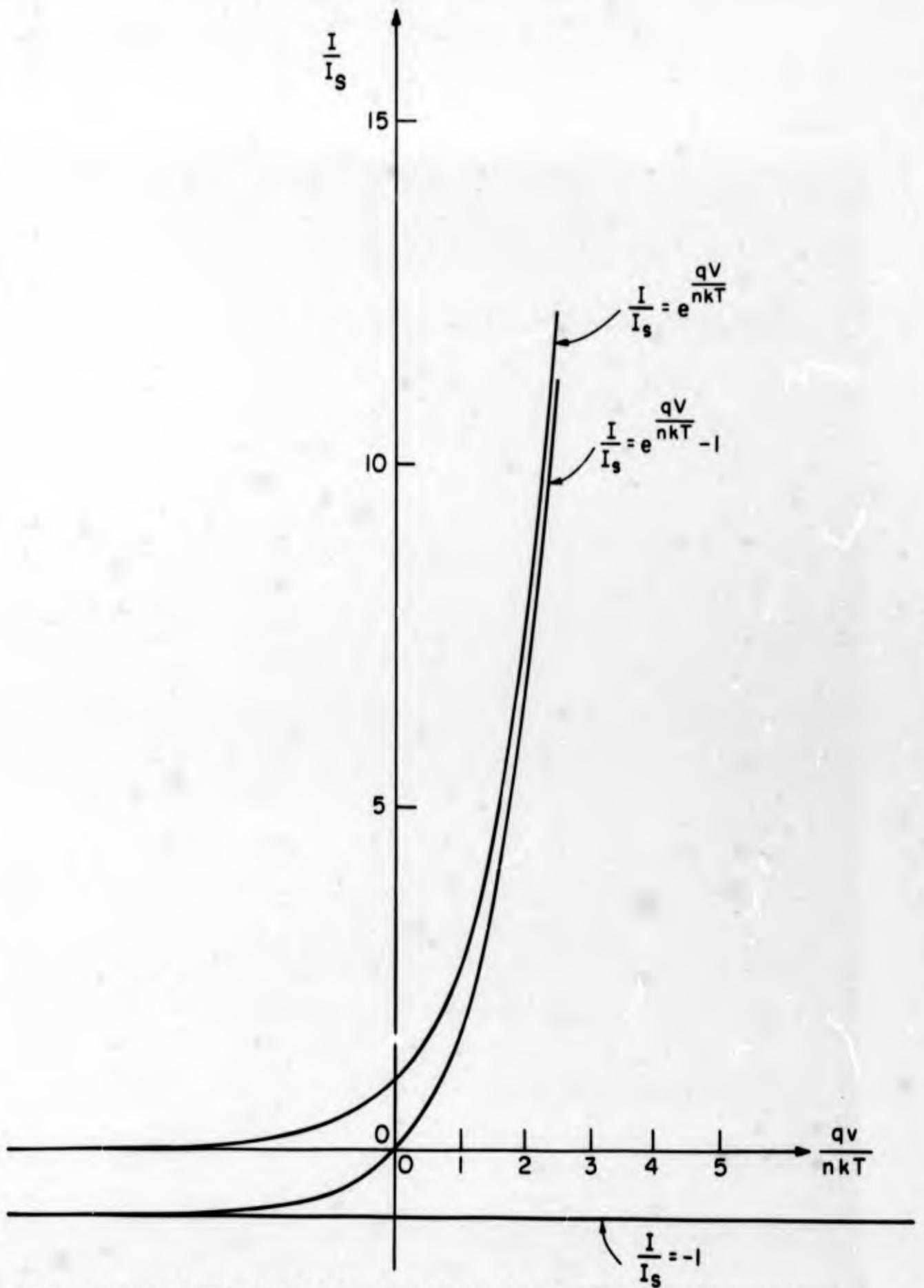
FIG. 3.4 EXPANDED NORMALIZED IDEAL DIODE CURRENT VERSUS EXPONENT AND APPROXIMATIONS
