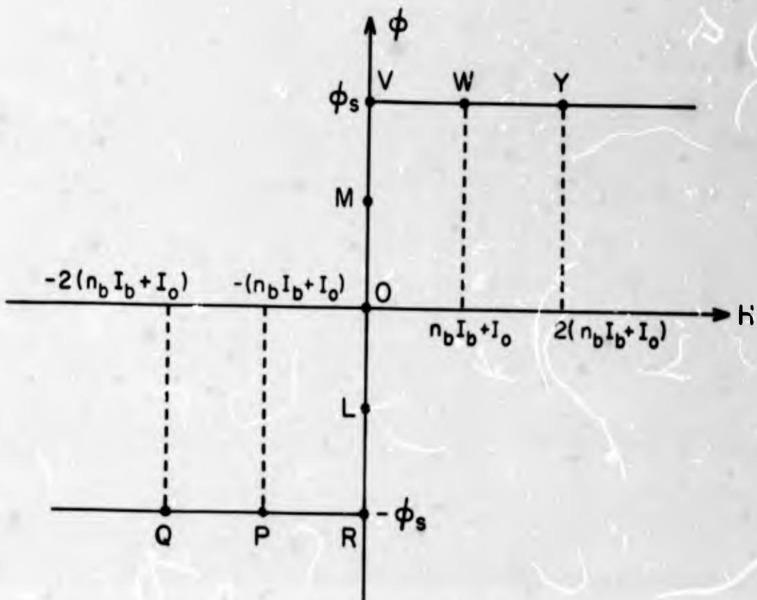
FIGURE 12.26 CURRENT SENSING TRANSFORMER
