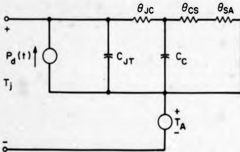
FIG. 3.26 DYNAMIC THERMAL CIRCUIT MODEL FOR A SINGLE DEVICE
