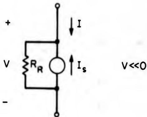
FIG. 3.9 DIODE MODEL FOR NON-CONDUCTING
