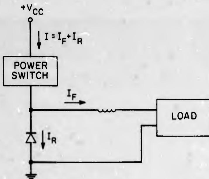
FIG. 3.20 POWER OUTPUT STAGE DURING THE SWITCH TURN - ON INTERVAL
