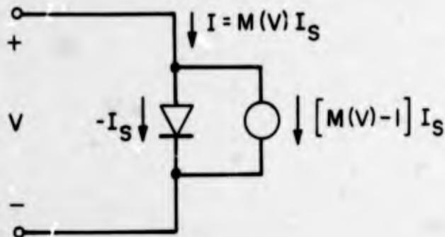
FIG.3.21 DIODE MODEL ILLUSTRATING AVALANCHE MULTIPLICATION
