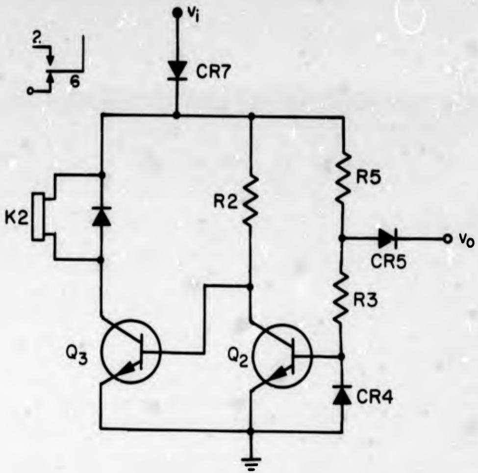
FIGURE 12.14 SCHEMATIC OF POLARITY SENSING CIRCUIT
