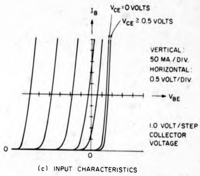
FIG. 3.35 MEASURED TRANSISTOR CHARACTERISTICS
