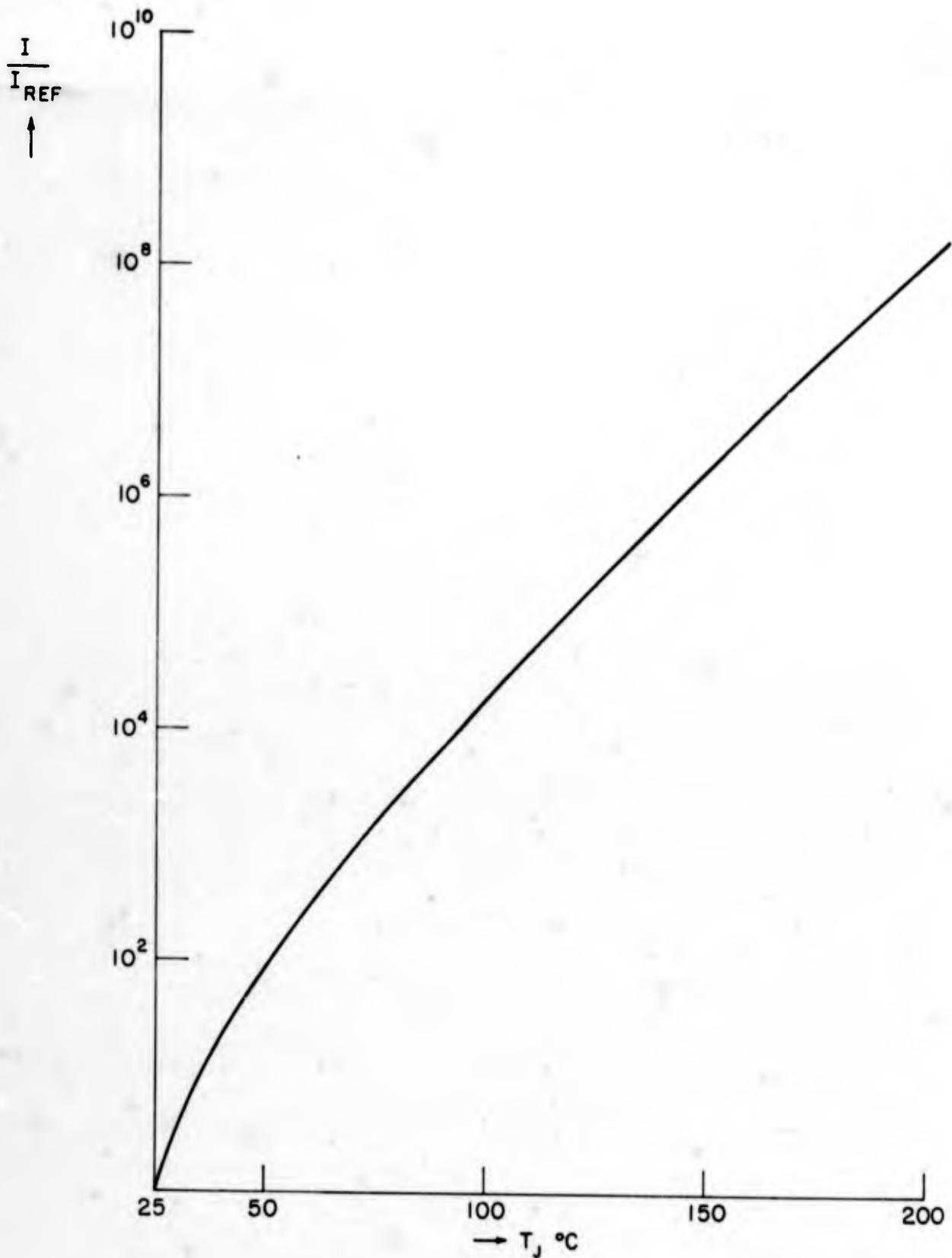
FIG.3.13 NORMALIZED REVERSE CURRENT CHANGE VERSUS TEMPERATURE RELATIVE TO 25 °C.
