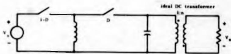
b. Addition of an ideal transformer to obtain a sign inversion.
