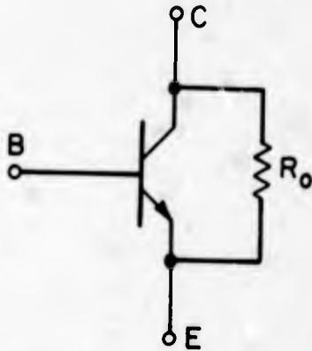
FIG.3.36 TRANSISTOR MODEL WITH RESISTOR TO ACCOUNT FOR BASE WIDTH MODULATION
