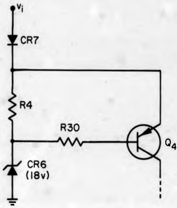
FIGURE 12.15 SCHEMATIC OF INPUT VOLTAGE SENSING CIRCUIT
