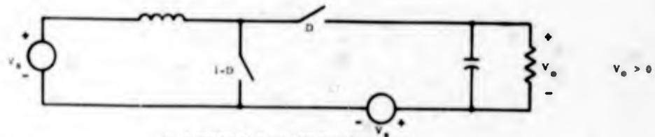
b. Flyback with  $V_s$  subtracted from output.
