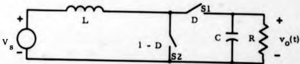
b. Output Circuit with Switches Reinserted
