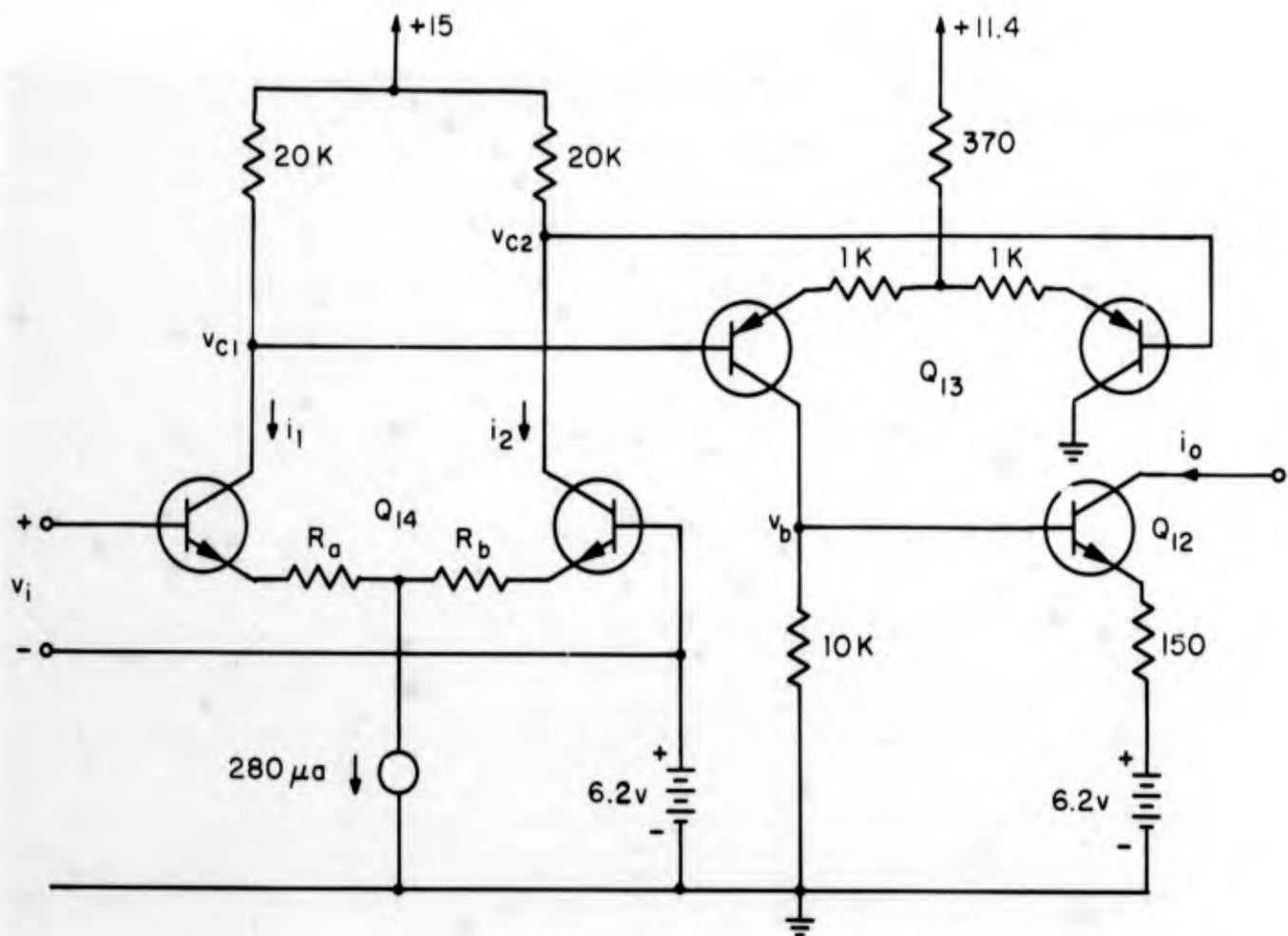
FIGURE 12.43 SIMPLIFIED MODEL OF ERROR AMPLIFIER
