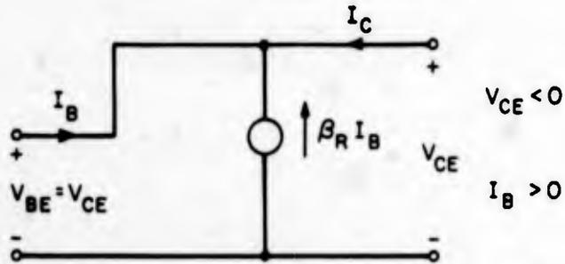
b. CURRENT SOURCE MODEL OF A TRANSISTOR IN THE REVERSE-ACTIVE REGION.
