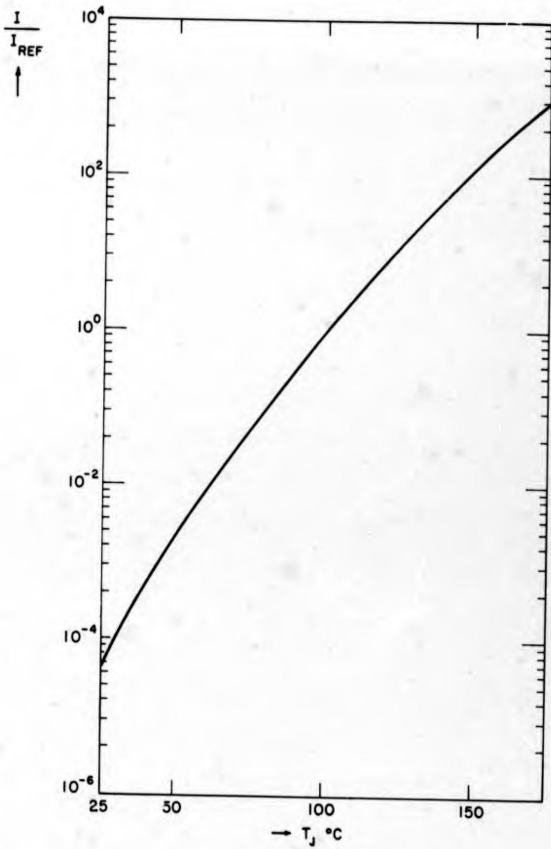
FIG. 3.14 NORMALIZED REVERSE CURRENT CHANGE VERSUS TEMPERATURE RELATIVE TO 100°C.
