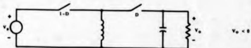
f. Circuit in e) with source polarity reversed. Note the change in the polarity of allowed output voltages.
