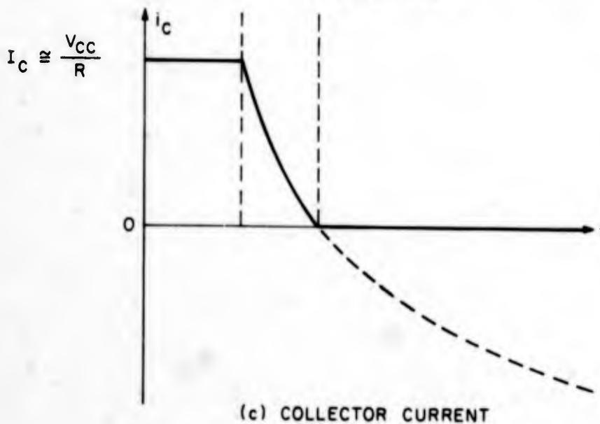
FIG. 3.46 TRANSISTOR SATURATION
