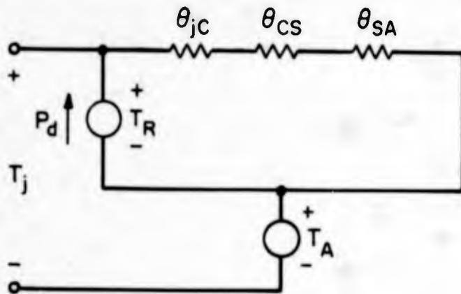
FIG. 3.24 STATIC THERMAL CIRCUIT MODEL FOR SINGLE CONVECTION COOLED DIODE
