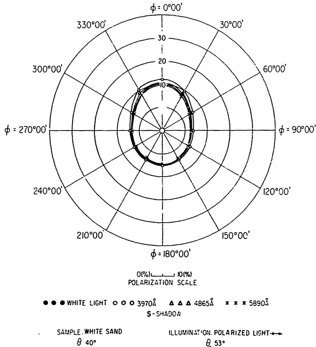
FIG 13I POLAR DIAGRAM SHOWING AZIMUTHAL VARIATION OF THE POLARIZATION OF REFLECTED LIGHT
