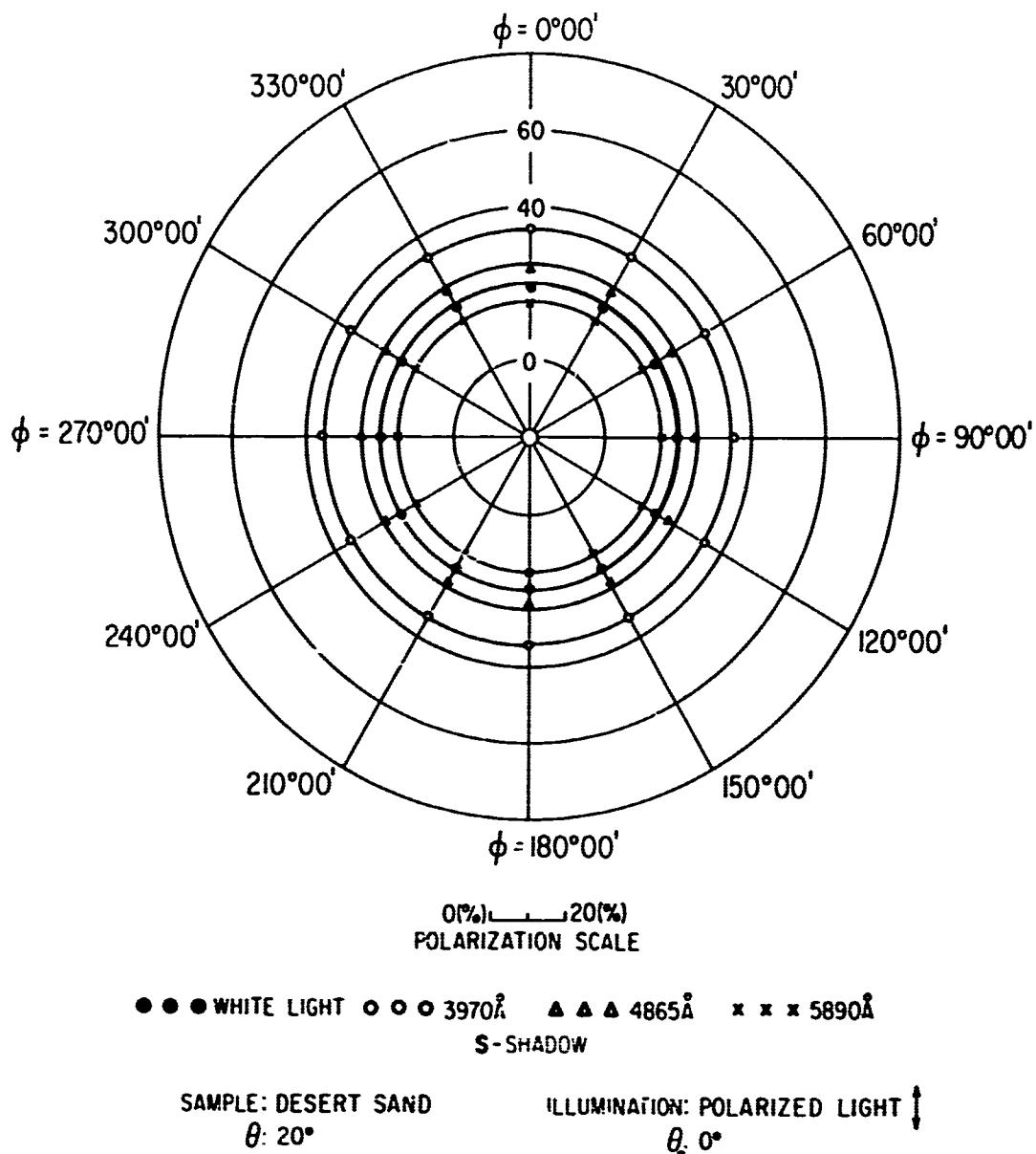
FIG 6I. POLAR DIAGRAM SHOWING AZIMUTHAL VARIATION OF THE POLARIZATION OF REFLECTED LIGHT
