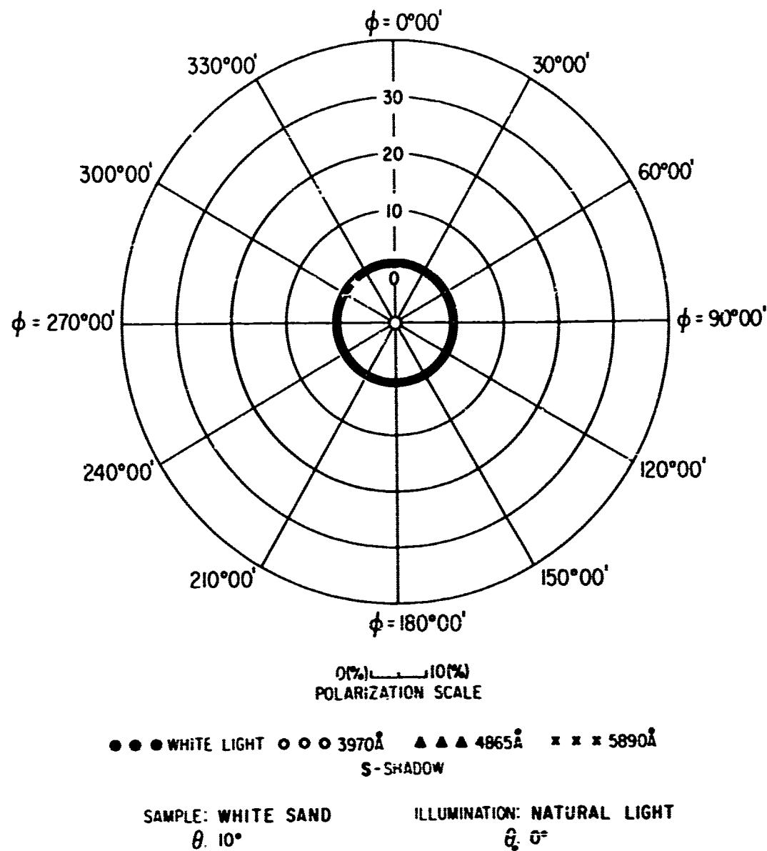
FIG 89. POLAR DIAGRAM SHOWING AZIMUTHAL VARIATION OF THE POLARIZATION OF REFLECTED LIGHT
