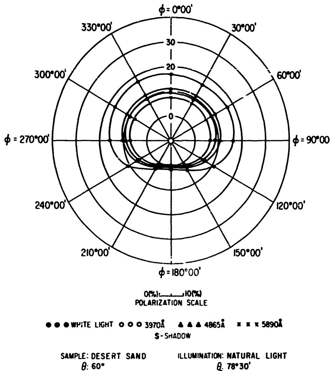
FIG 27. POLAR DIAGRAM SHOWING AZIMUTHAL VARIATION OF THE POLARIZATION OF REFLECTED LIGHT
