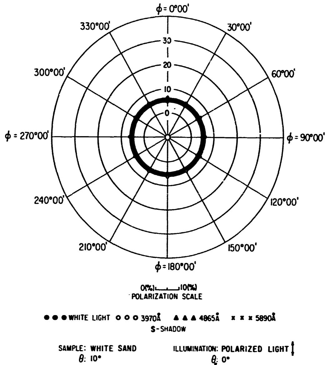
FIG 147 POLAR DIAGRAM SHOWING AZIMUTHAL VARIATION
