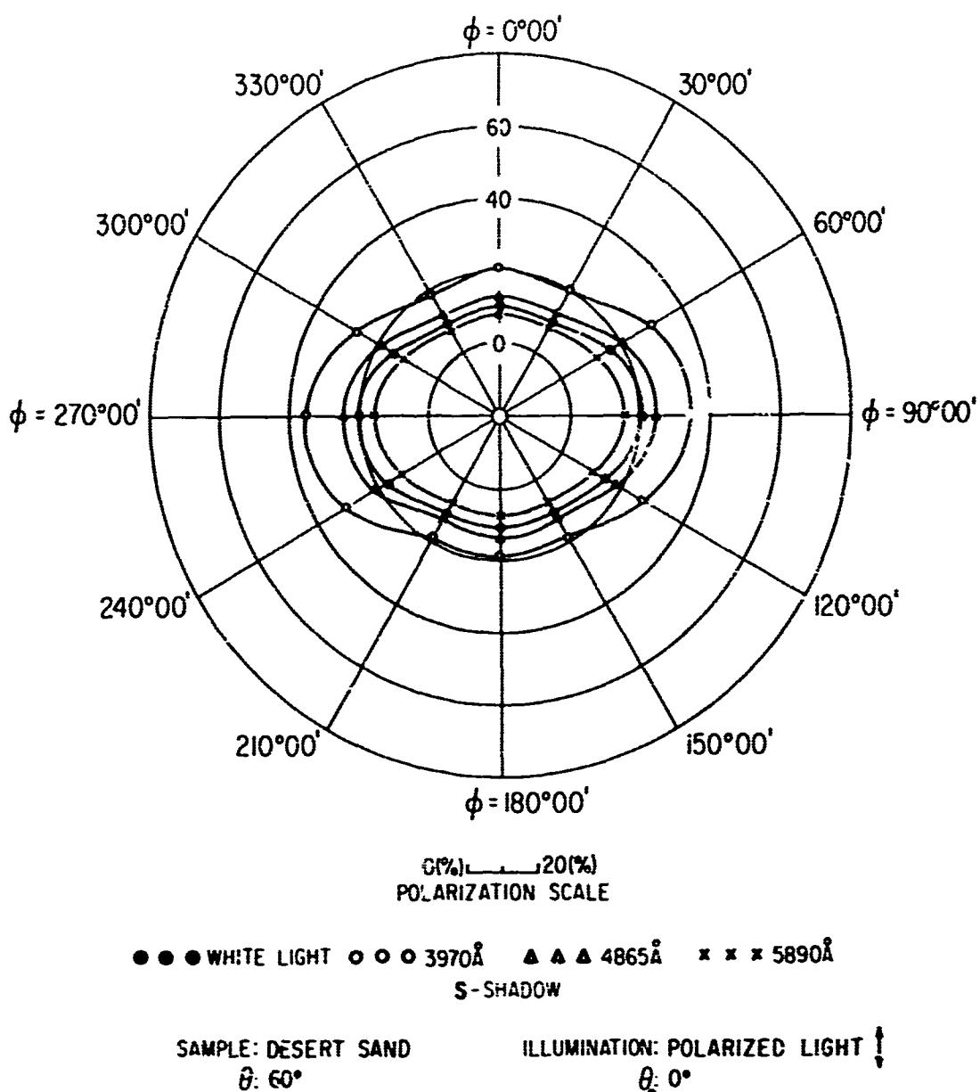
FIG. 65. POLAR DIAGRAM SHOWING AZIMUTHAL VARIATION OF THE POLARIZATION OF REFLECTED LIGHT
