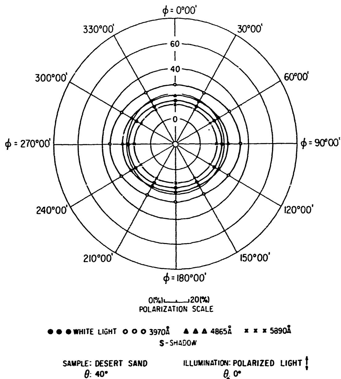
FIG 63. POLAR DIAGRAM SHOWING AZIMUTHAL VARIATION OF THE POLARIZATION OF REFLECTED LIGHT
