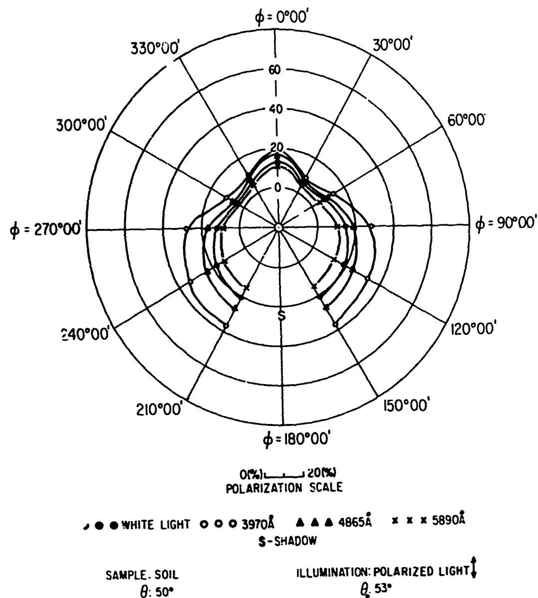
FIG. 248 POLAR DIAGRAM SHOWING AZIMUTHAL VARIATION
