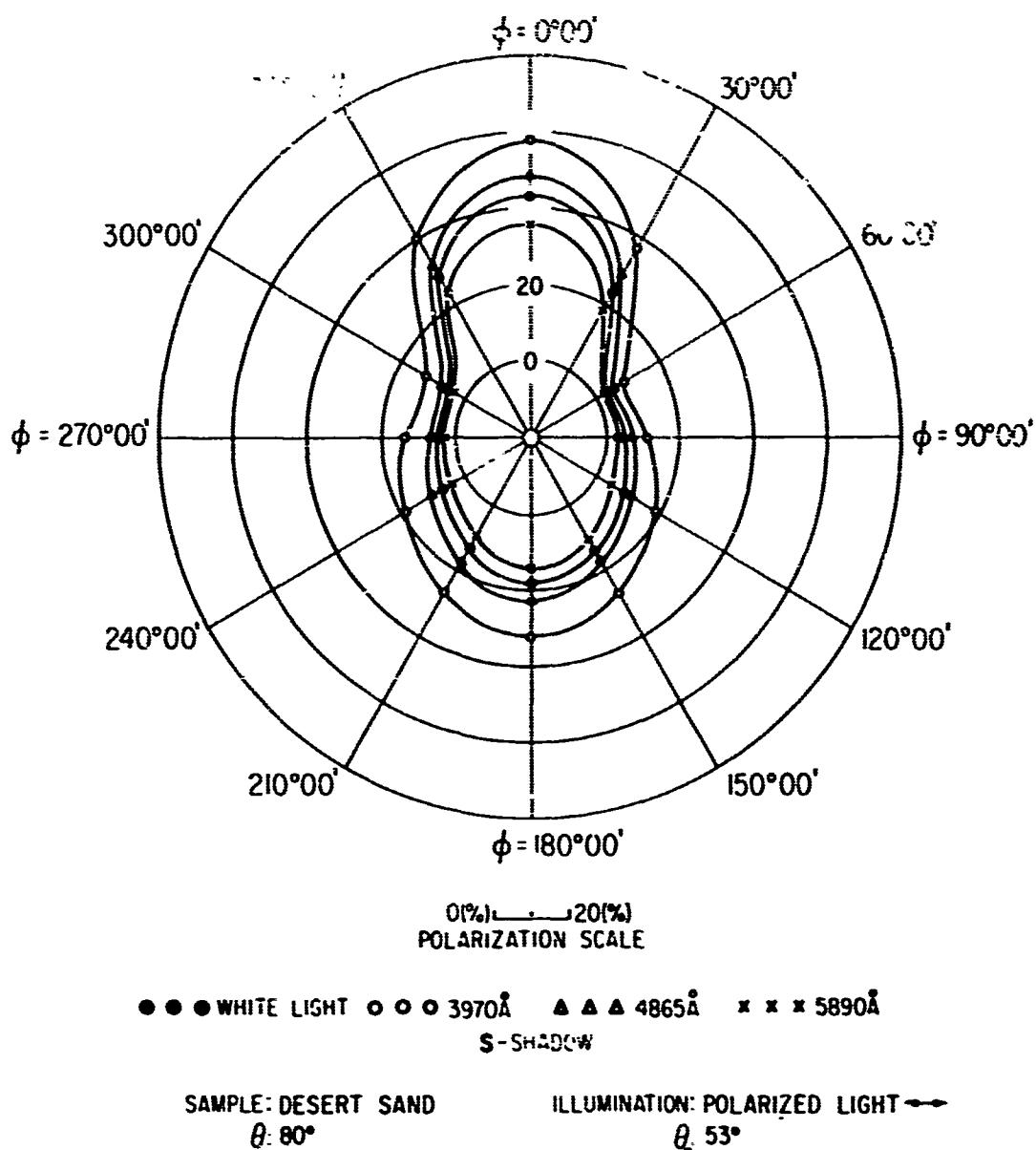
FIG 49. POLAR DIAGRAM SHOWING AZIMUTHAL VARIATION OF THE POLARIZATION OF REFLECTED LIGHT
