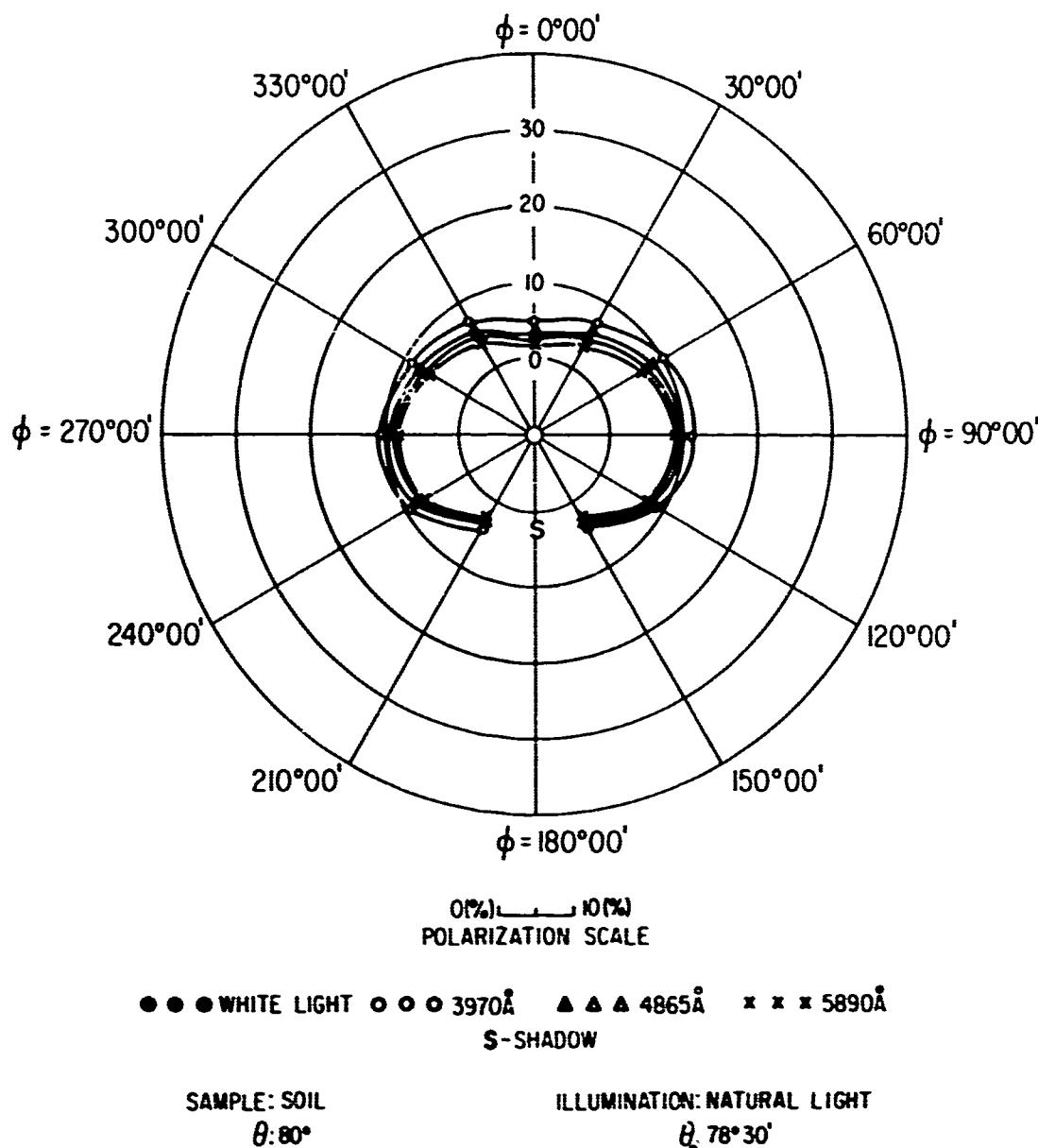
FIG.204 POLAR DIAGRAM SHOWING AZIMUTHAL VARIATION
