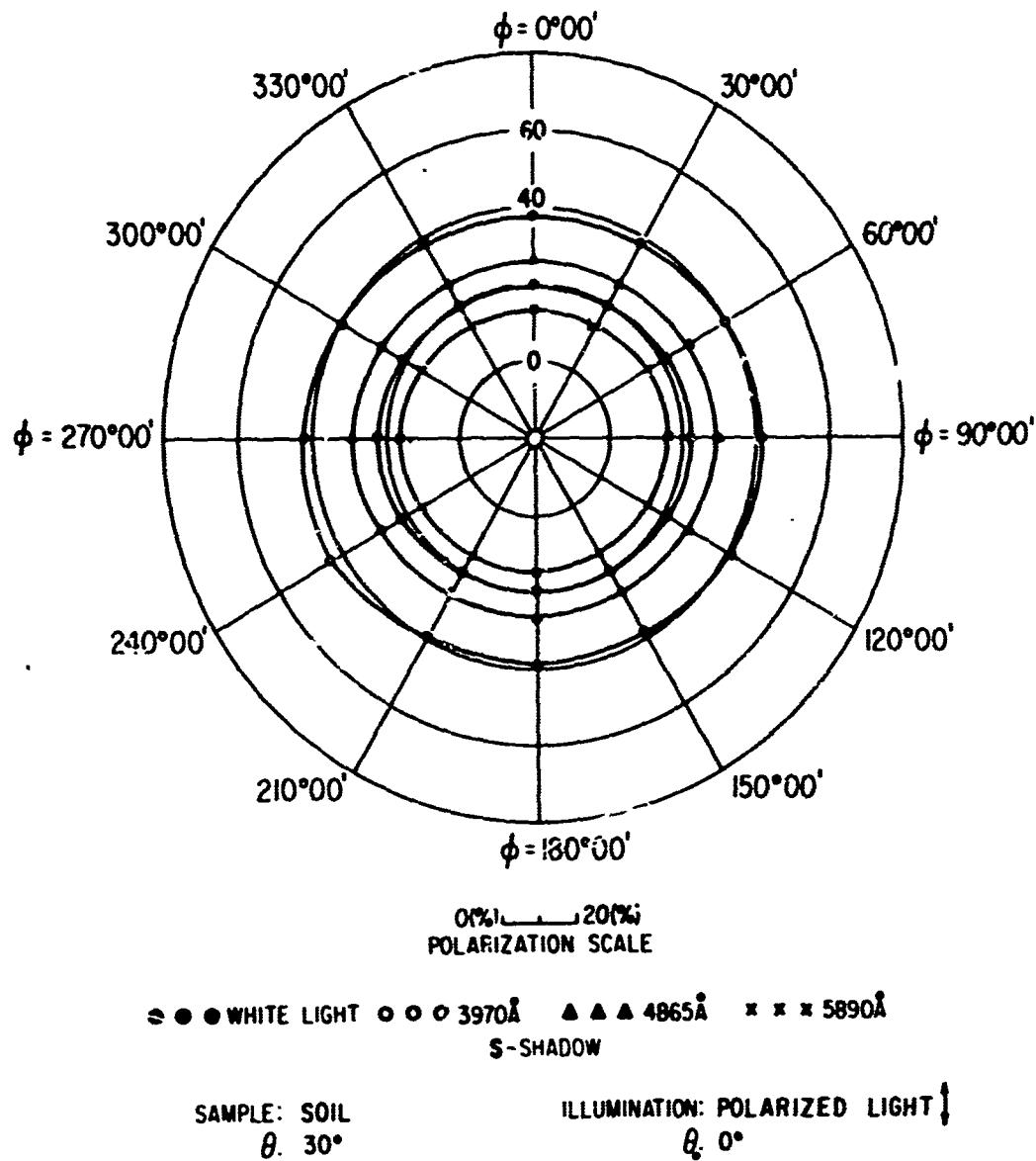
FIG. 236. POLAR DIAGRAM SHOWING AZIMUTHAL VARIATION
