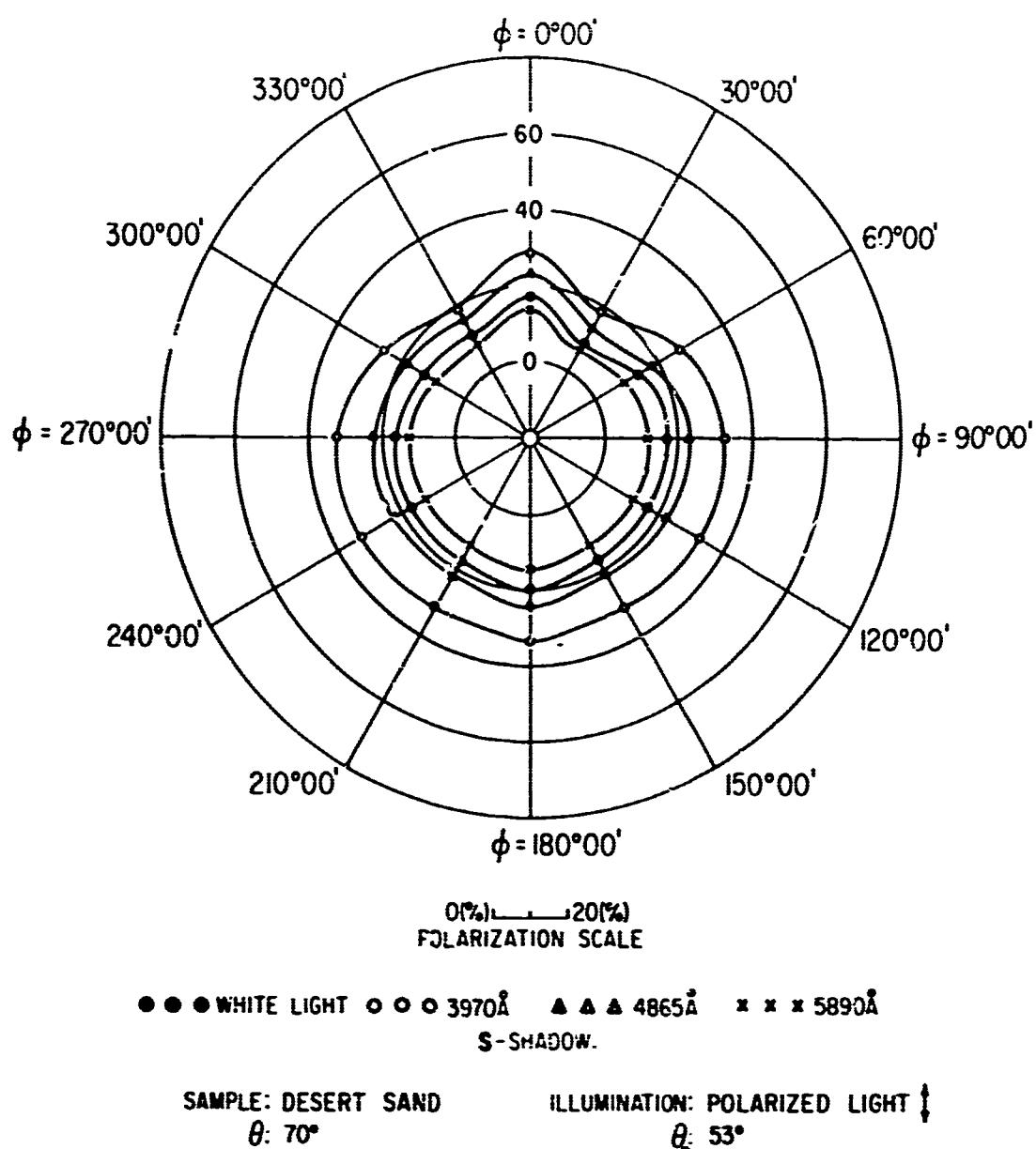
FIG. 76. POLAR DIAGRAM SHOWING AZIMUTHAL VARIATION OF THE POLARIZATION OF REFLECTED LIGHT
