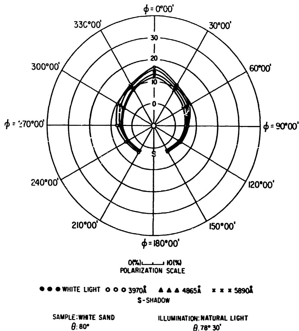
FIG. II7 POLAR DIAGRAM SHOWING AZIMUTHAL VARIATION OF THE POLARIZATION OF REFLECTED LIGHT
