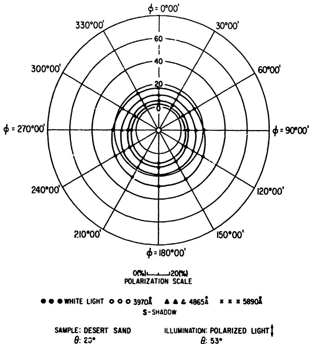
FIG. 71. POLAR DIAGRAM SHOWING AZIMUTHAL VARIATION OF THE POLARIZATION OF REFLECTED LIGHT
