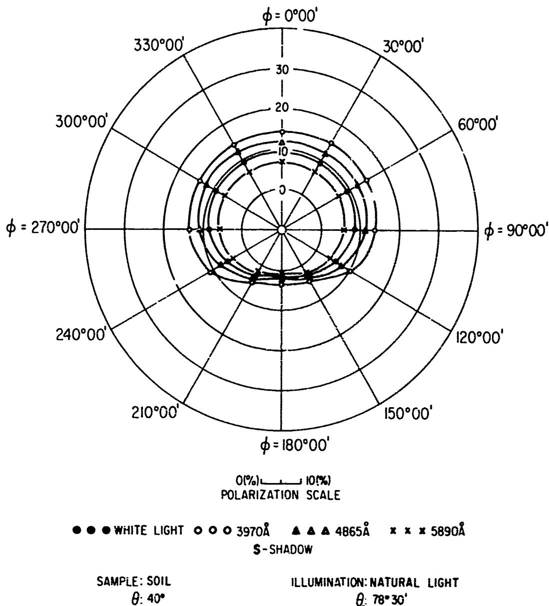
FIG. 199 POLAR DIAGRAM SHOWING AZIMUTHAL VARIATION
