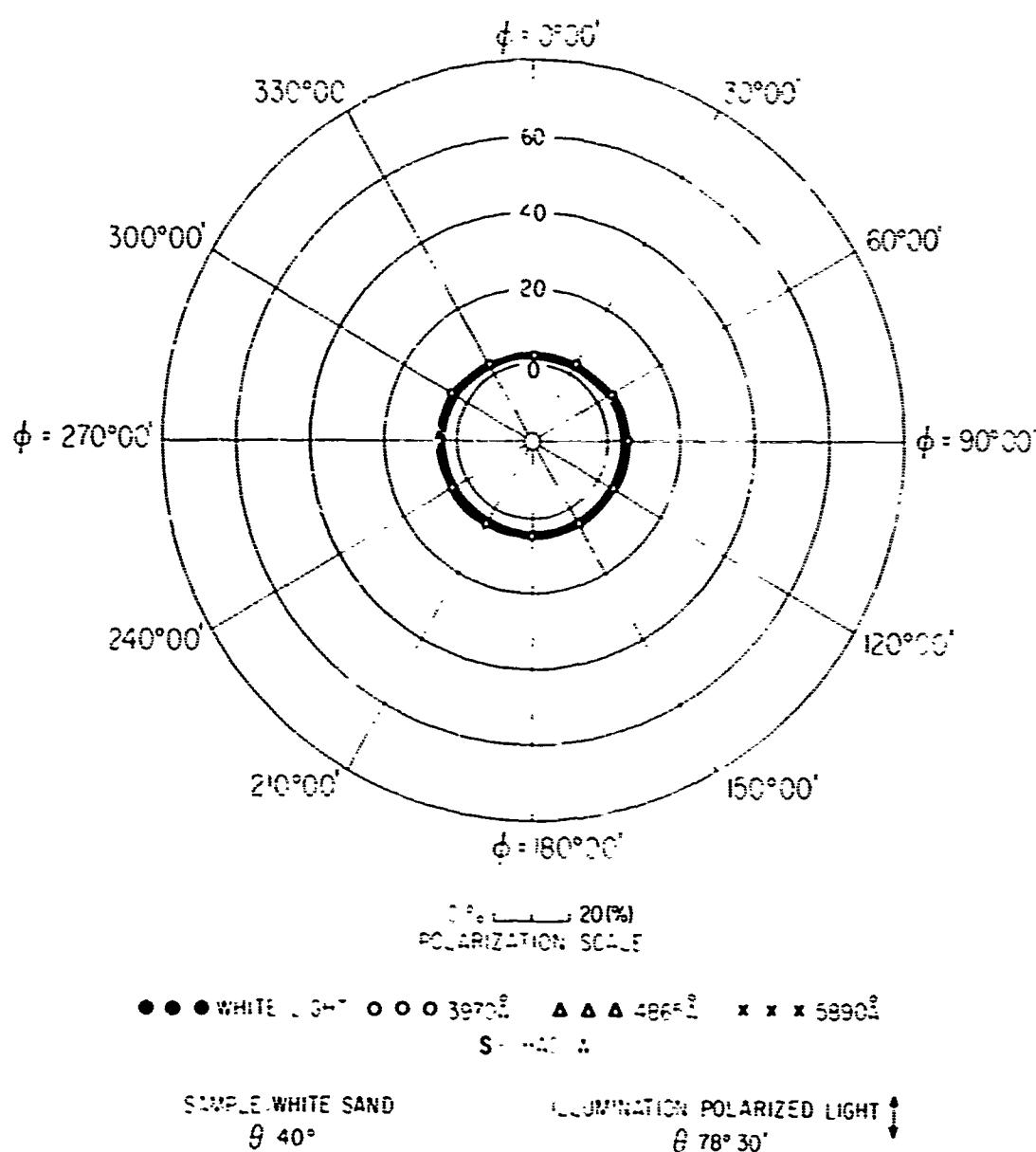
FIG 170 POLAR DIAGRAM SHOWING AZIMUTHAL VARIATION
