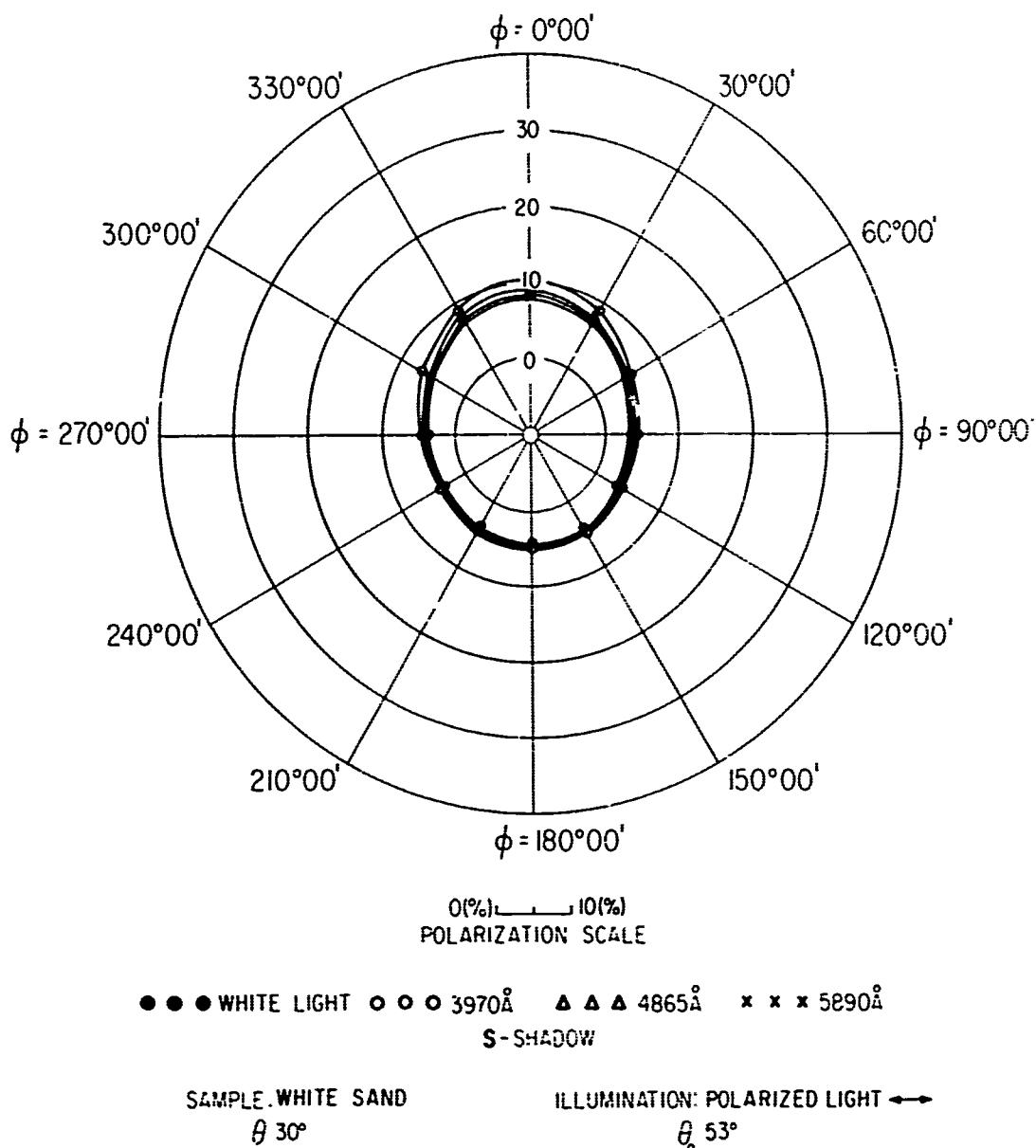
FIG 130 POLAR DIAGRAM SHOWING AZIMUTHAL VARIATION
