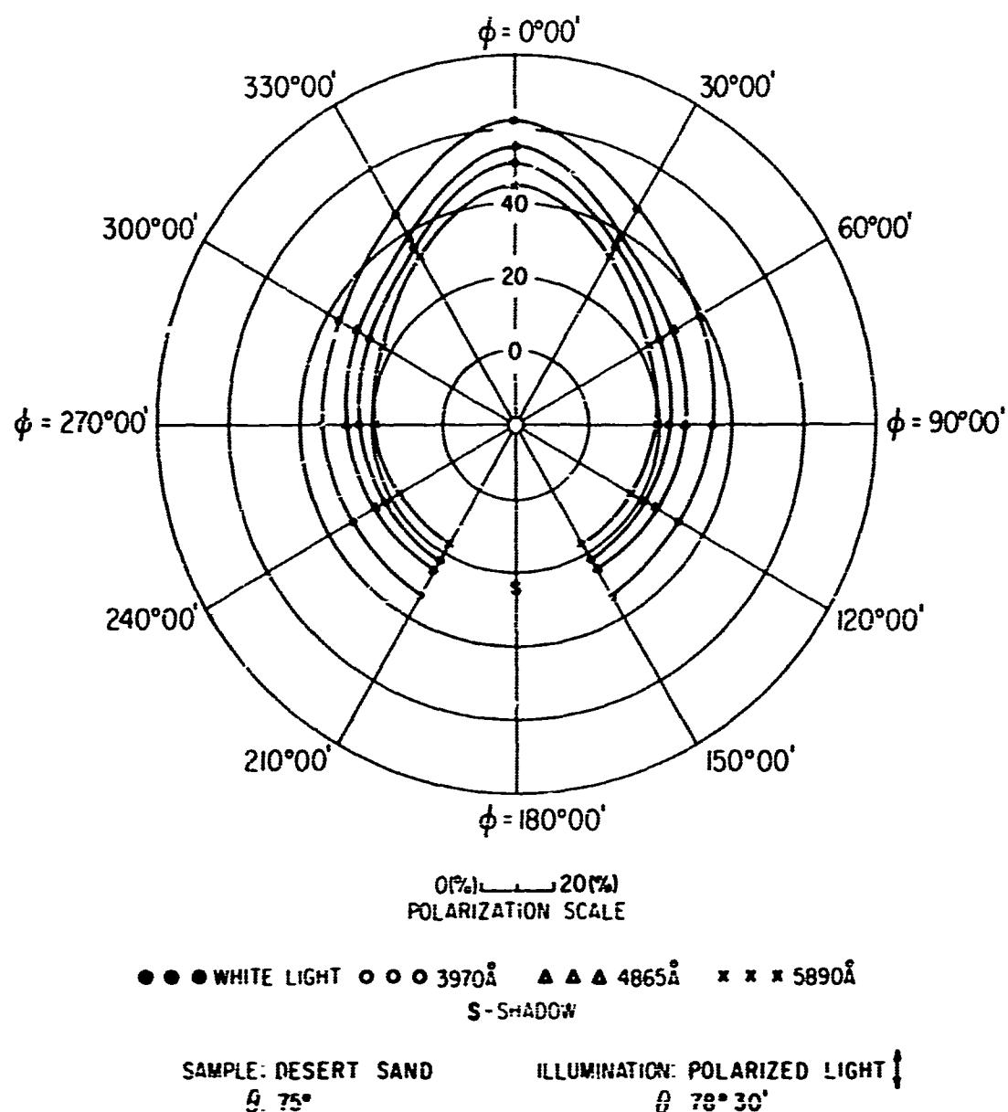
FIG 87. POLAR DIAGRAM SHOWING AZIMUTHAL VARIATION OF THE POLARIZATION OF REFLECTED LIGHT
