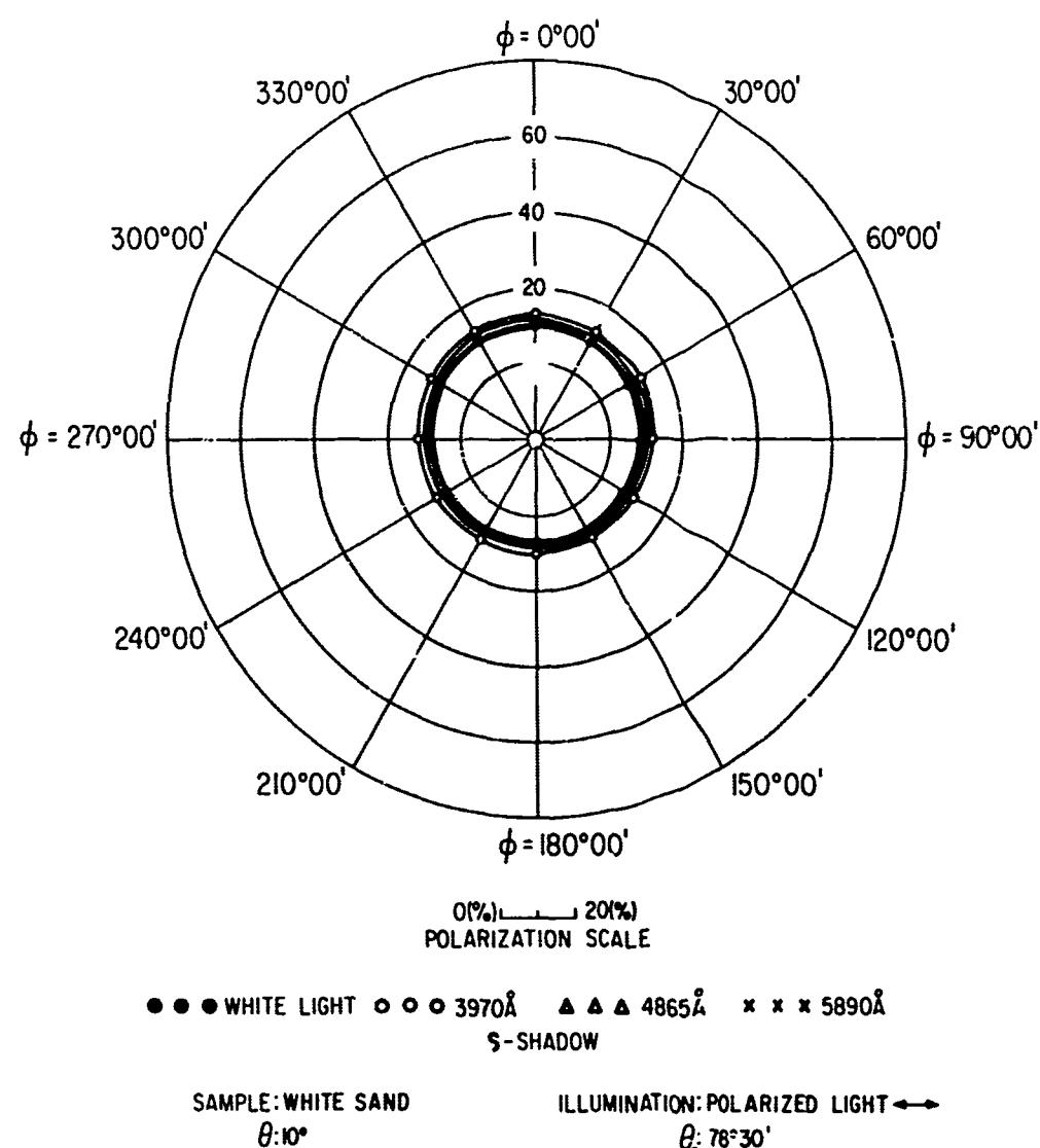
FIG.138 POLAR DIAGRAM SHOWING AZIMUTHAL VARIATION OF THE POLARIZATION OF REFLECTED LIGHT
