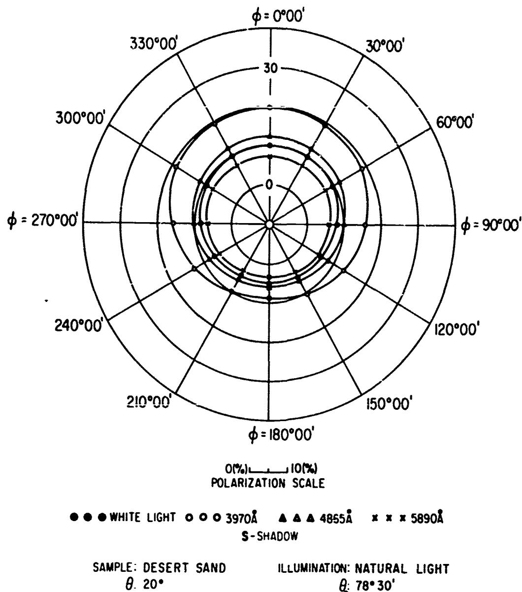
FIG 23. POLAR DIAGRAM SHOWING AZIMUTHAL VARIATION OF THE POLARIZATION OF REFLECTED LIGHT
