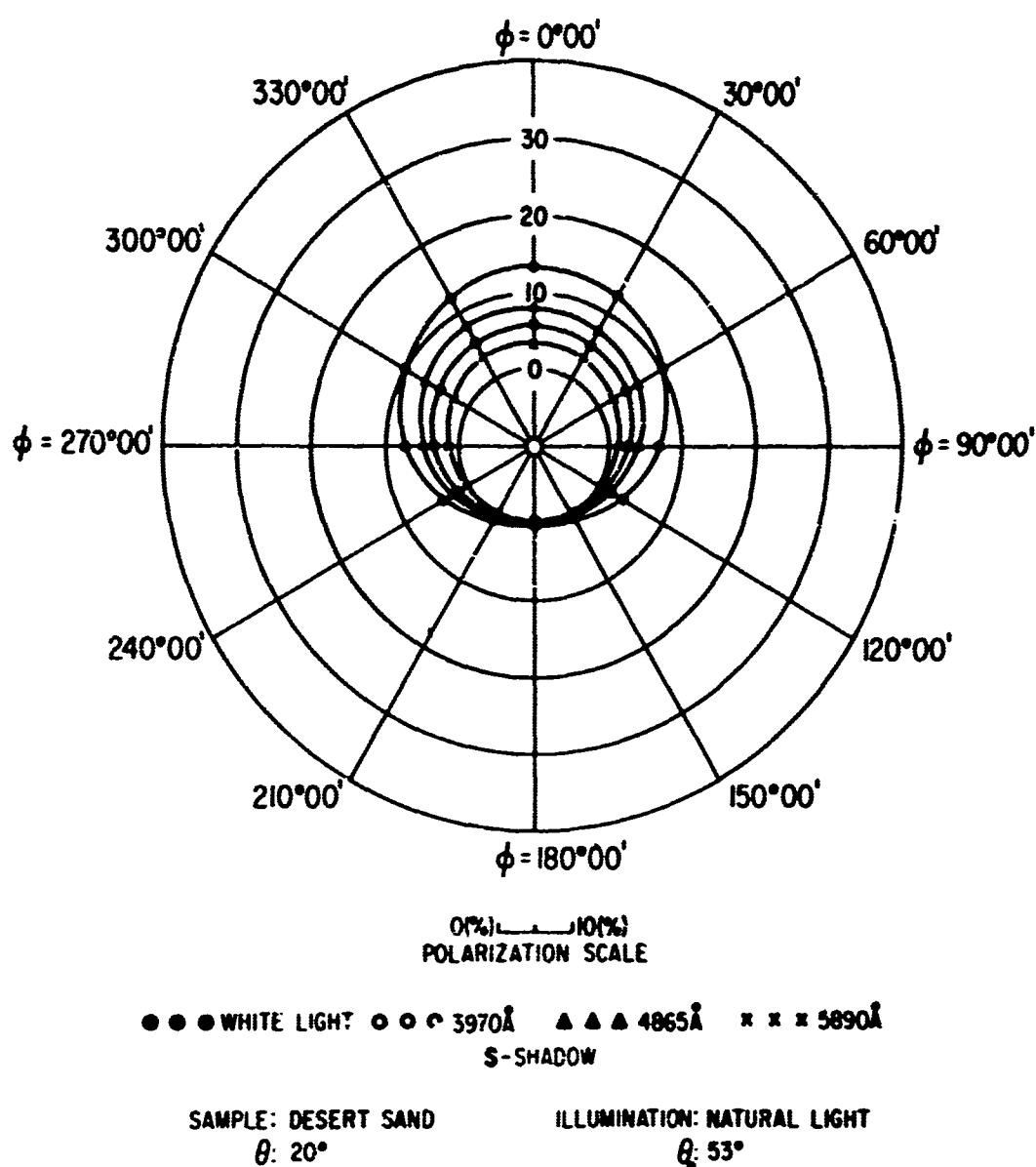
FIG 13. POLAR DIAGRAM SHOWING AZIMUTHAL VARIATION OF THE POLARIZATION OF REFLECTED LIGHT
