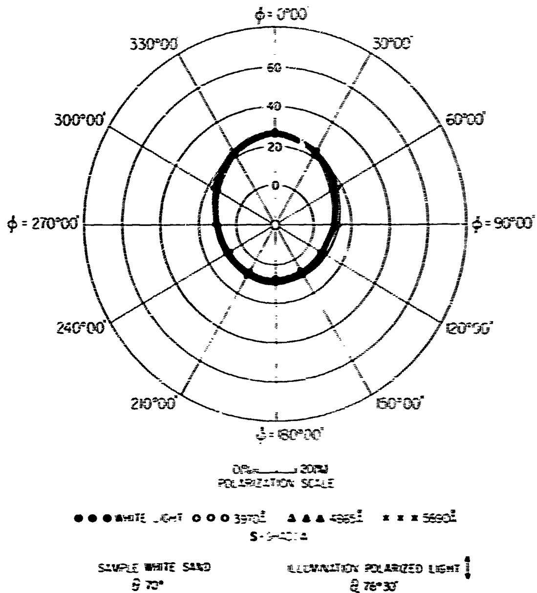
FIG. 173 POLAR DIAGRAM SHOWING AZIMUTHAL VARIATION
