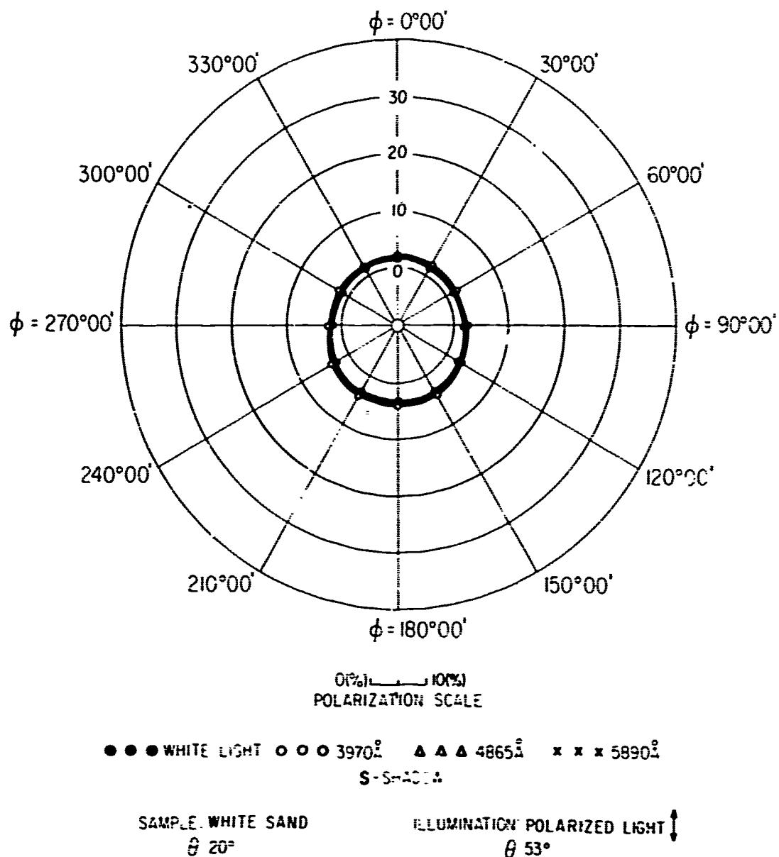
FIG 158 POLAR DIAGRAM SHOWING AZIMUTHAL VARIATION
