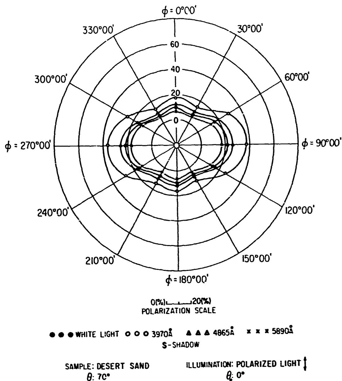
FIG 66. POLAR DIAGRAM SHOWING AZIMUTHAL VARIATION
