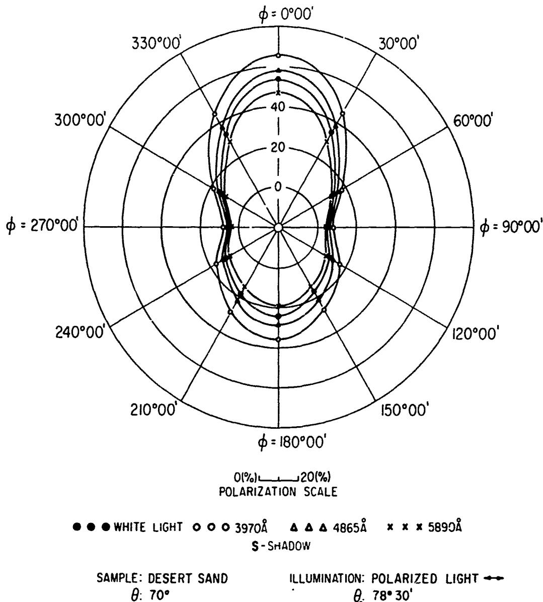
FIG 57. POLAR DIAGRAM SHOWING AZIMUTHAL VARIATION OF THE POLARIZATION OF REFLECTED LIGHT
