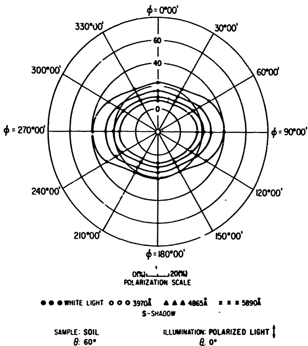
FIG. 239. POLAR DIAGRAM SHOWING AZIMUTHAL VARIATION
