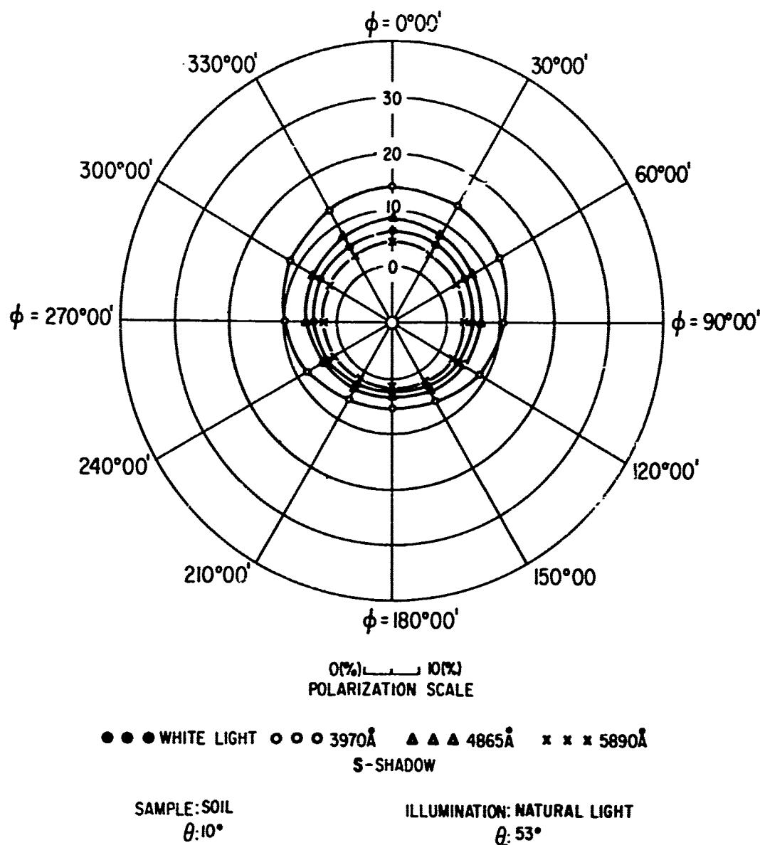
FIG. 186 POLAR DIAGRAM SHOWING AZIMUTHAL VARIATION
