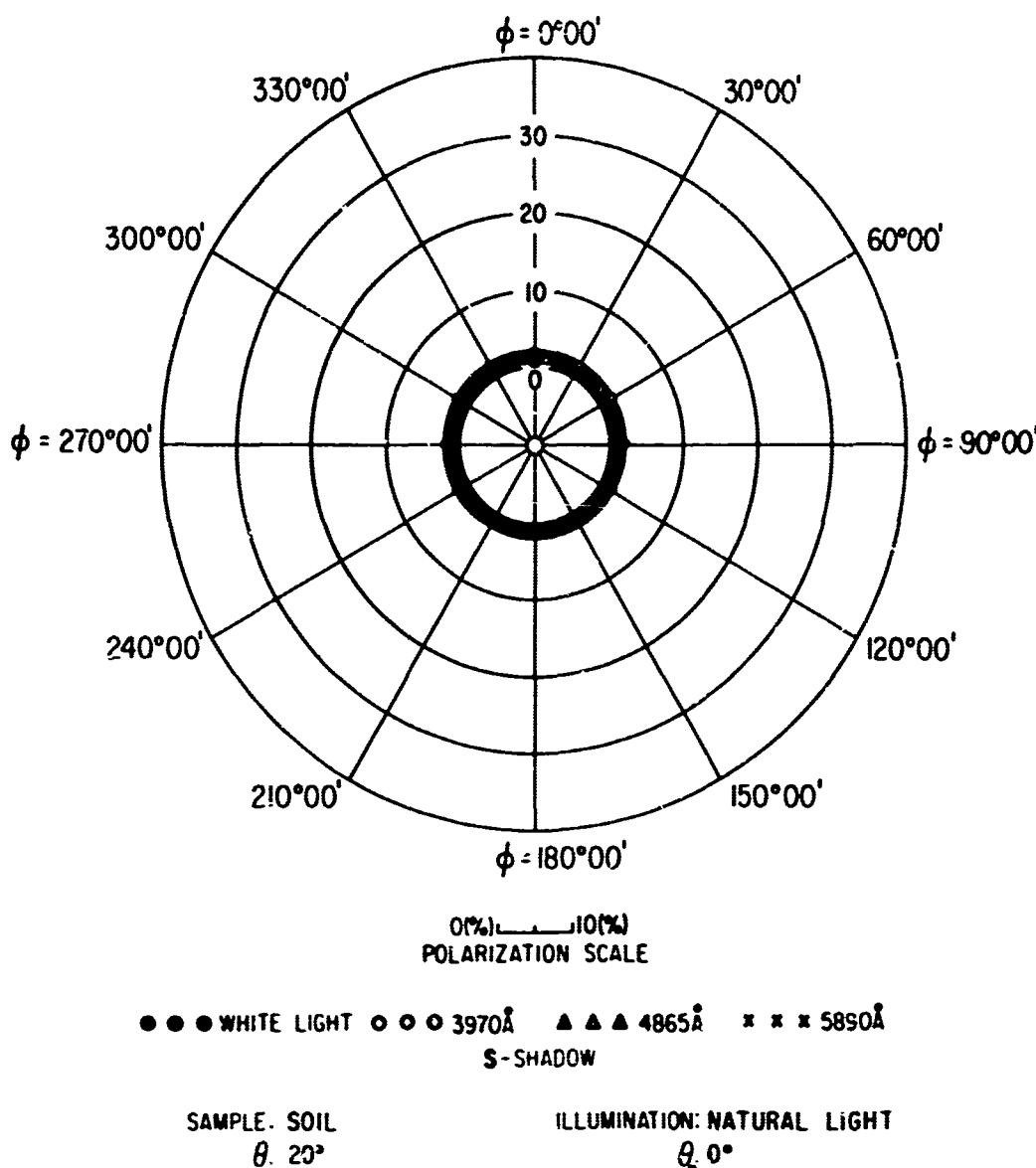
FIG. 177. POLAR DIAGRAM SHOWING AZIMUTHAL VARIATION OF THE POLARIZATION OF REFLECTED LIGHT
