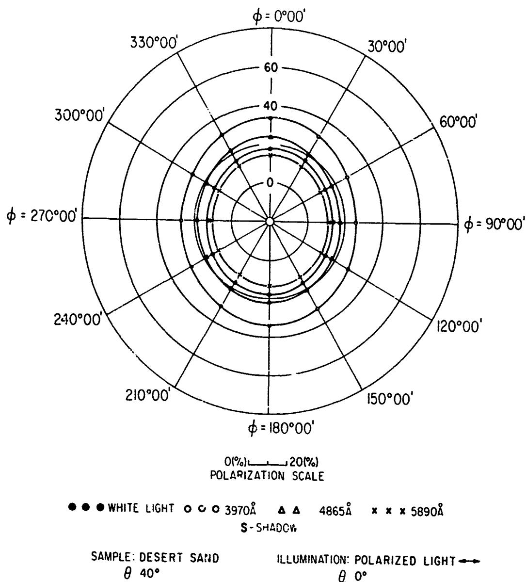
FIG 34. POLAR DIAGRAM SHOWING AZIMUTHAL VARIATION
