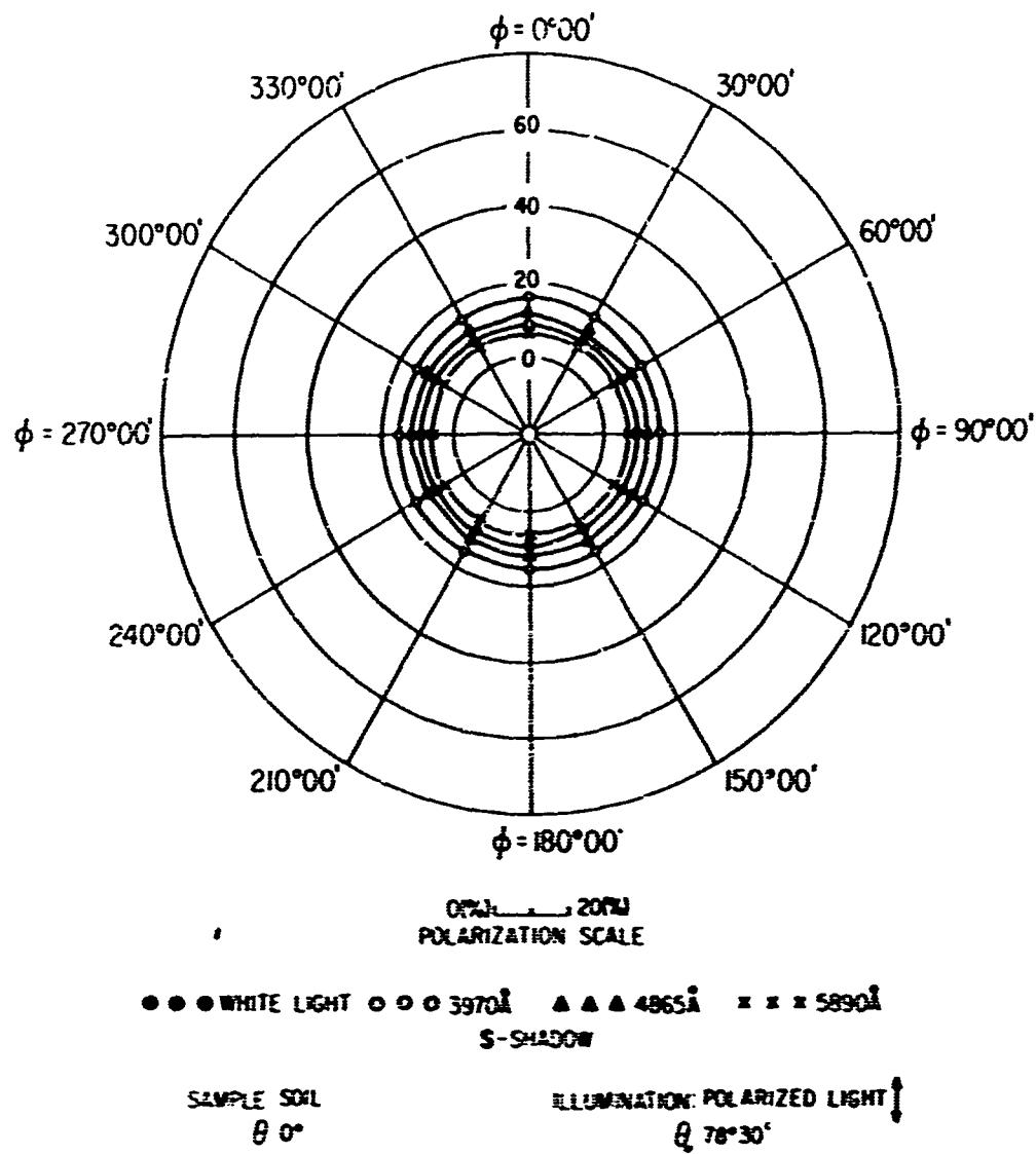
FIG 253 POLAR DIAGRAM SHOWING AZIMUTHAL VARIATION
