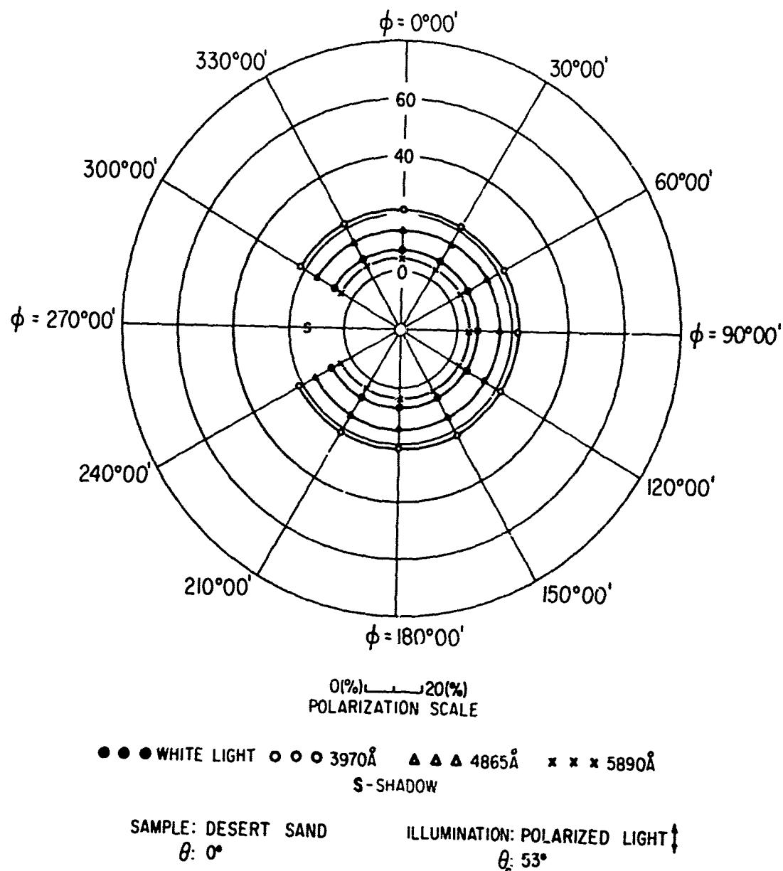
FIG 69. POLAR DIAGRAM SHOWING AZIMUTHAL VARIATION OF THE POLARIZATION OF REFLECTED LIGHT
