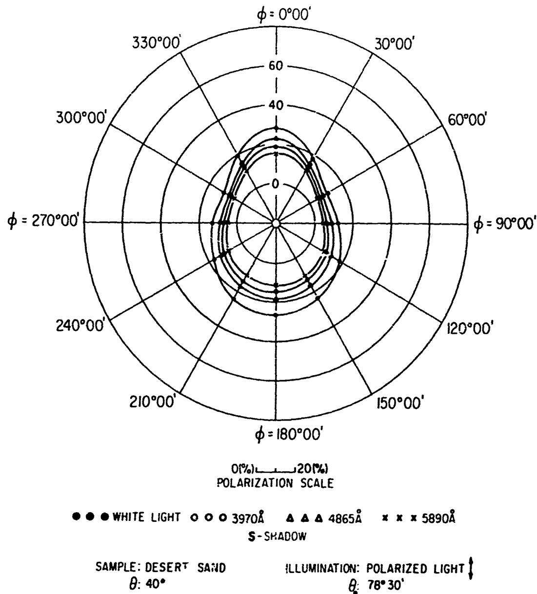
FIG 83. POLAR DIAGRAM SHOWING AZIMUTHAL VARIATION
