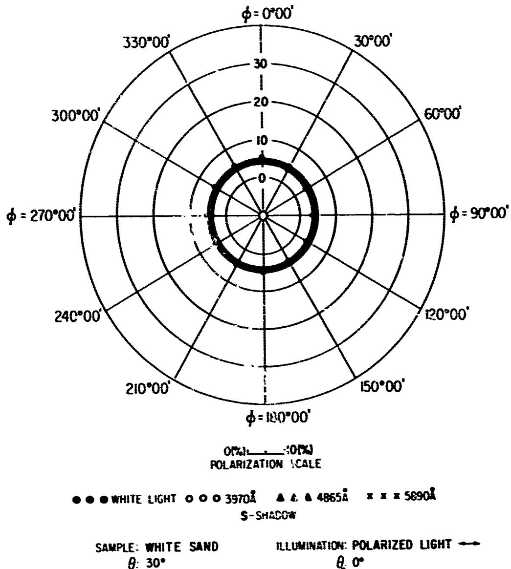
FIG 120. POLAR DIAGRAM SHOWING AZIMUTHAL VARIATION
