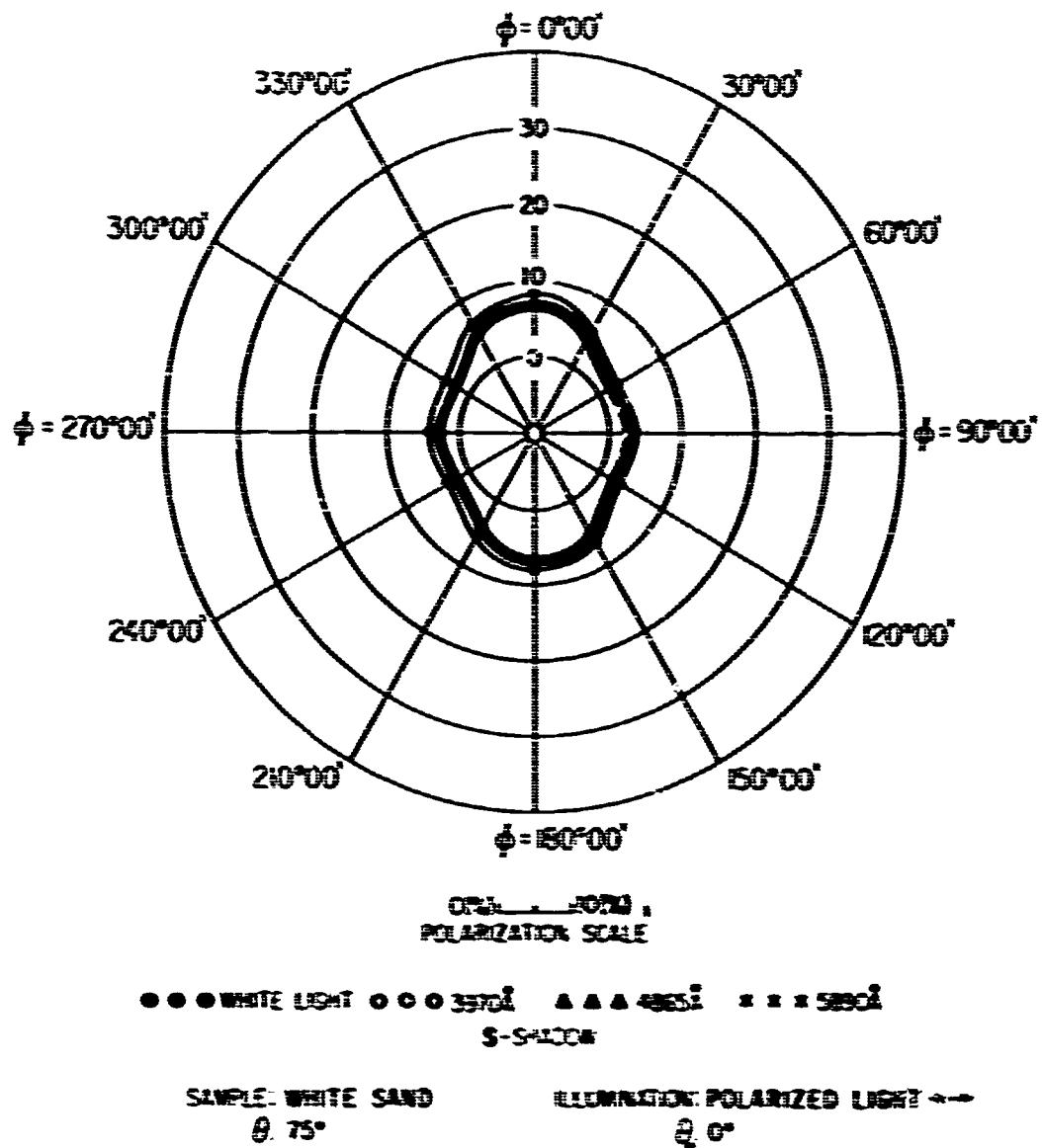
FIG 125. POLAR DIAGRAM SHOWING AZIMUTHAL VARIATION
