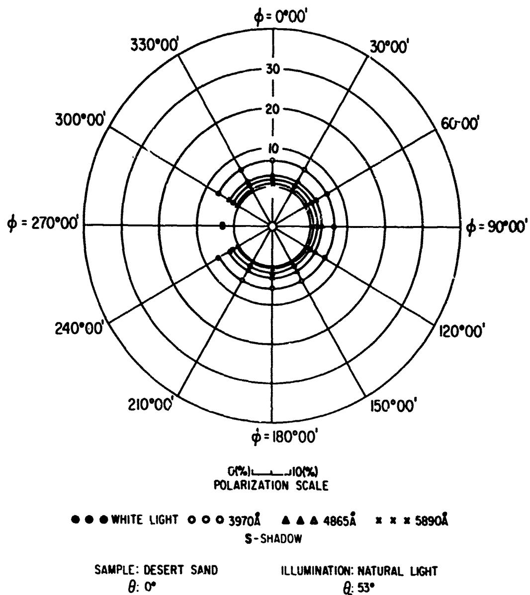
FIG 11. POLAR DIAGRAM SHOWING AZIMUTHAL VARIATION OF THE POLARIZATION OF REFLECTED LIGHT
