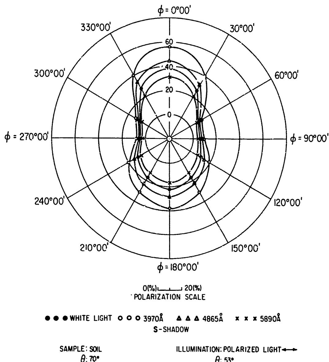
FIG.221 POLAR DIAGRAM SHOWING AZIMUTHAL VARIATION OF THE POLARIZATION OF REFLECTED LIGHT
