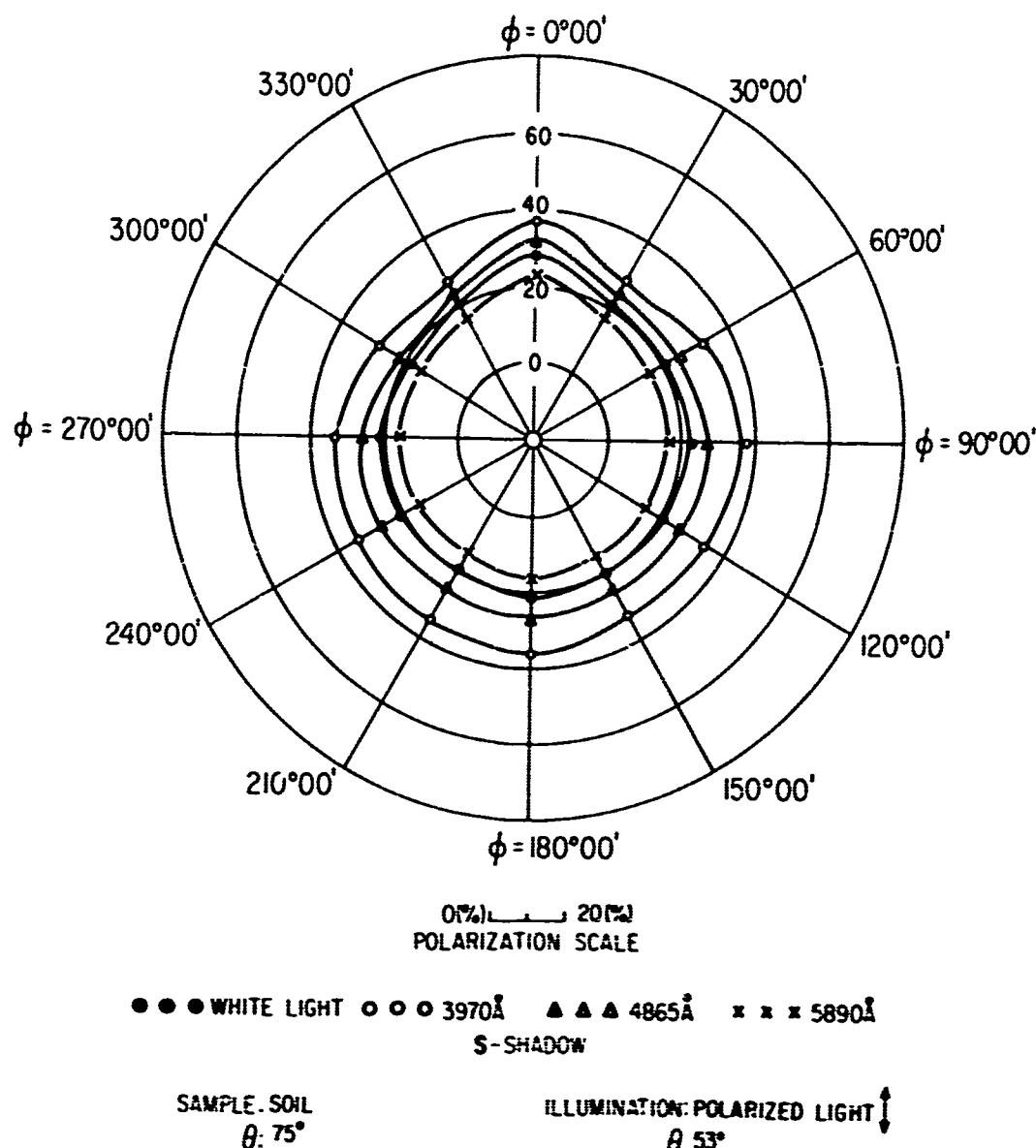
FIG. 251 POLAR DIAGRAM SHOWING AZIMUTHAL VARIATION OF THE POLARIZATION OF REFLECTED LIGHT
