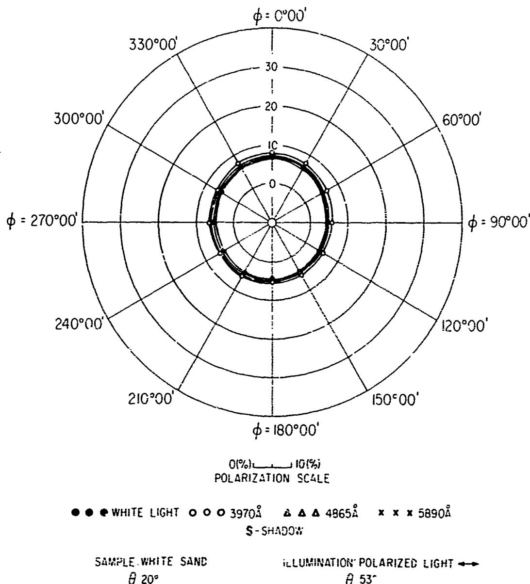
FIG 129 POLAR DIAGRAM SHOWING AZIMUTHAL VARIATION OF THE POLARIZATION OF REFLECTED LIGHT
