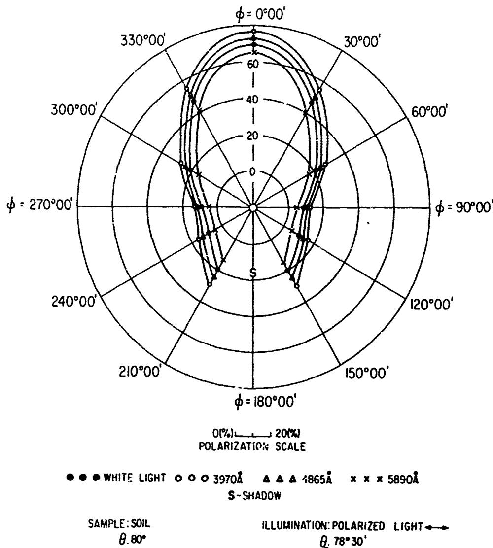
FIG.233 POLAR DIAGRAM SHOWING AZIMUTHAL VARIATION
