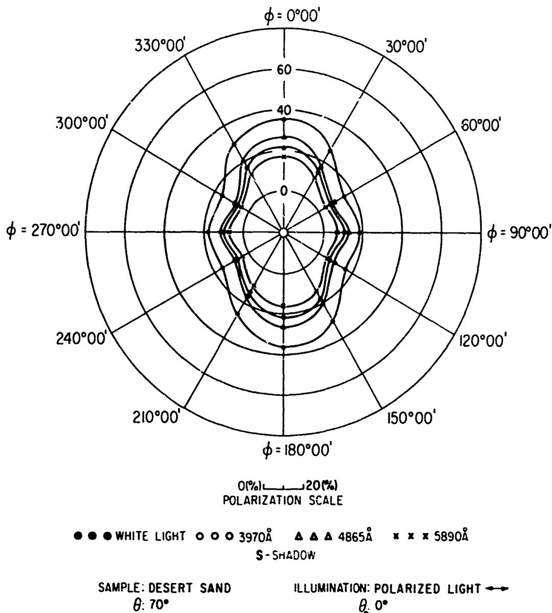
FIG 37. POLAR DIAGRAM SHOWING AZIMUTHAL VARIATION OF THE POLARIZATION OF REFLECTED LIGHT
