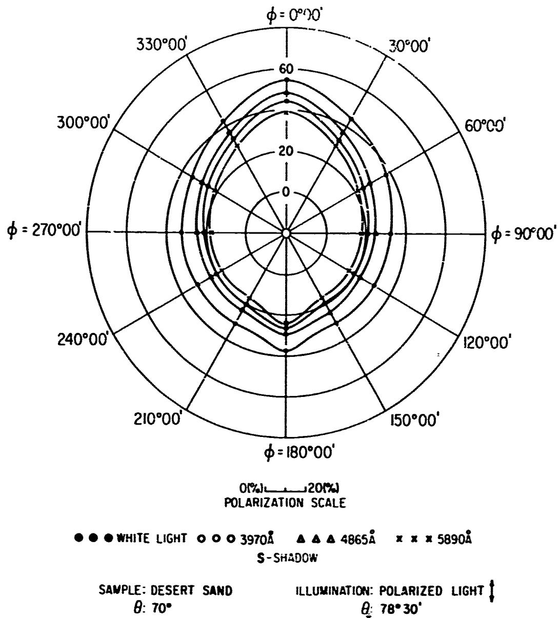
FIG 86. POLAR DIAGRAM SHOWING AZIMUTHAL VARIATION OF THE POLARIZATION OF REFLECTED LIGHT
