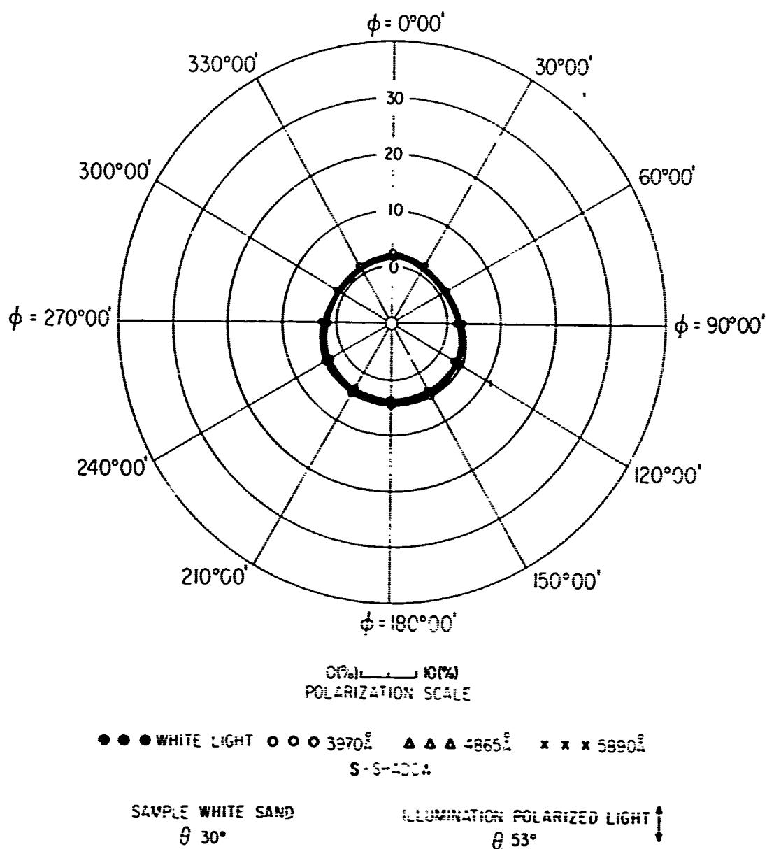
FIG 159 POLAR DIAGRAM SHOWING AZIMUTHAL VARIATION
