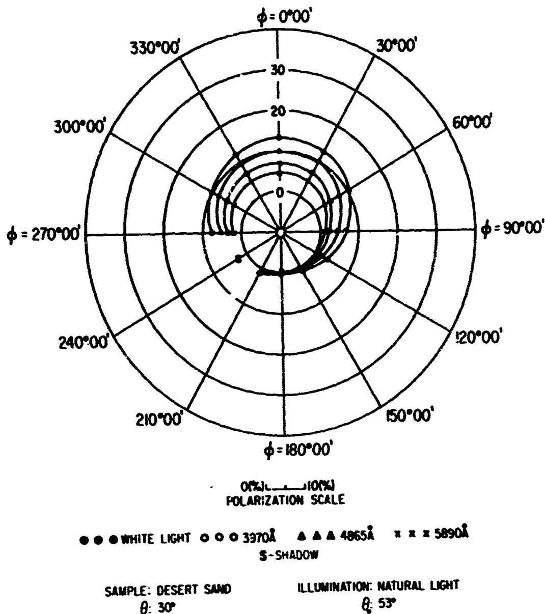
FIG. 14. POLAR DIAGRAM SHOWING AZIMUTHAL VARIATION OF THE POLARIZATION OF REFLECTED LIGHT
