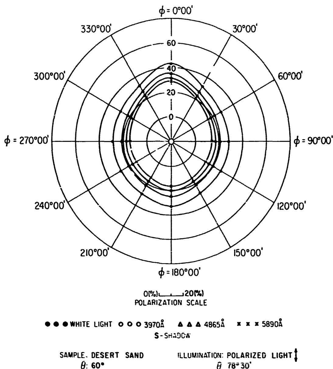
FIG 85. POLAR DIAGRAM SHOWING AZIMUTHAL VARIATION OF THE POLARIZATION OF REFLECTED LIGHT
