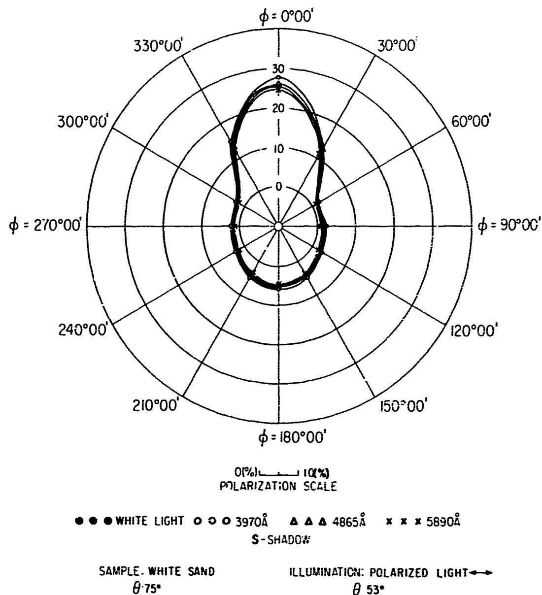
FIG. 135 POLAR DIAGRAM SHOWING AZIMUTHAL VARIATION
