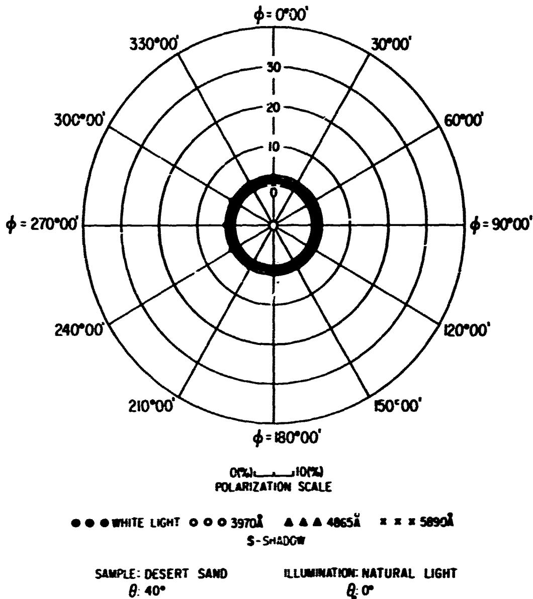
FIG 5. POLAR DIAGRAM SHOWING AZIMUTHAL VARIATION OF THE POLARIZATION OF REFLECTED LIGHT
