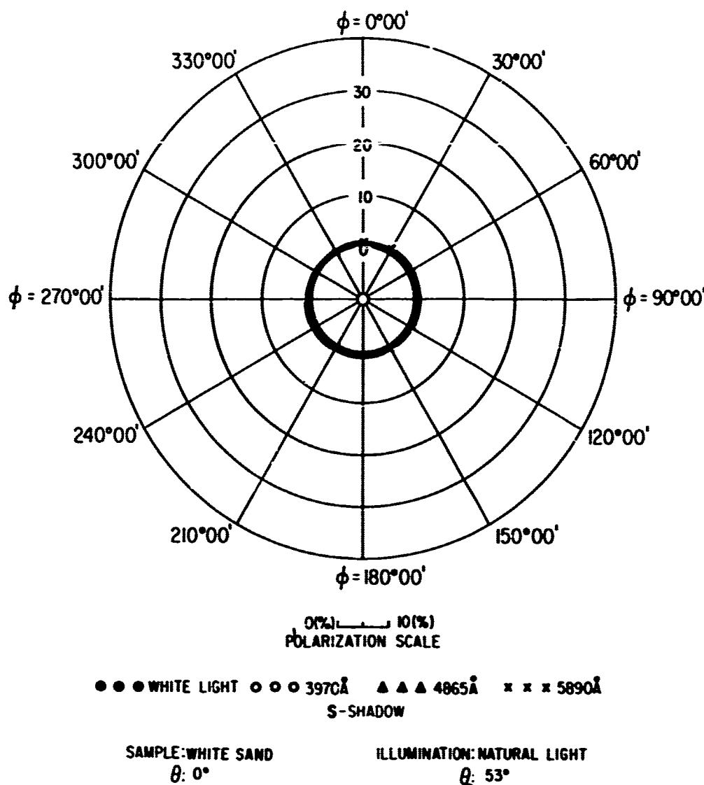
FIG. 98 POLAR DIAGRAM SHOWING AZIMUTHAL VARIATION
