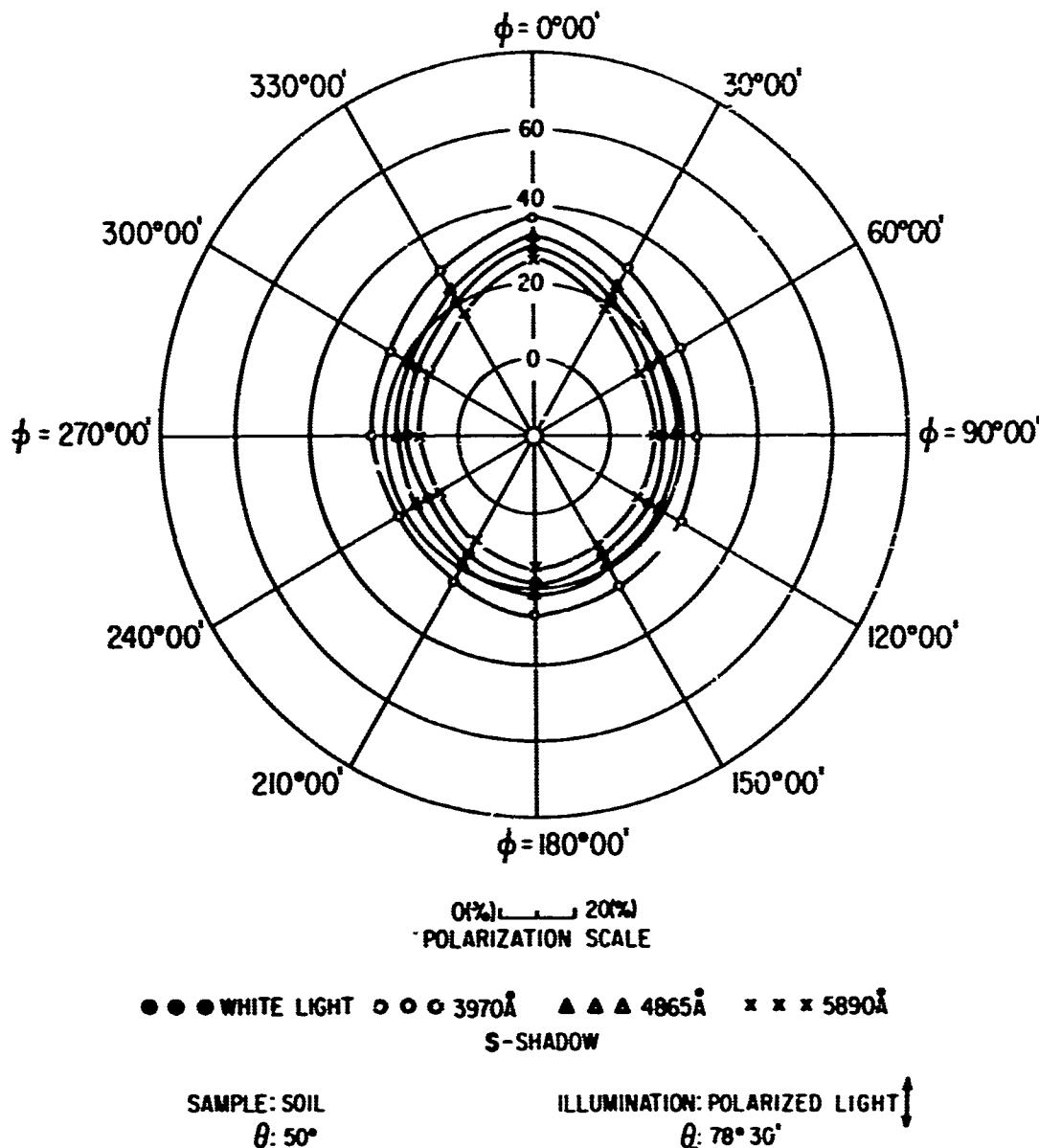
FIG.258 POLAR DIAGRAM SHOWING AZIMUTHAL VARIATION OF THE POLARIZATION OF REFLECTED LIGHT
