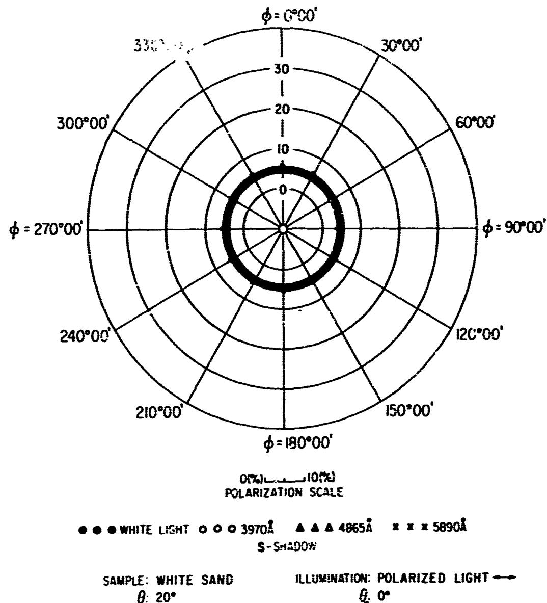
FIG 119. POLAR DIAGRAM SHOWING AZIMUTHAL VARIATION OF THE POLARIZATION OF REFLECTED LIGHT
