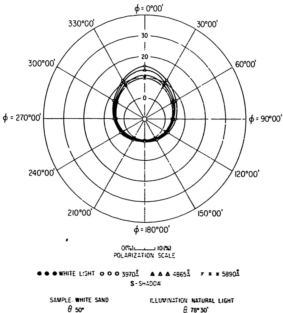
FIG II3 POLAR DIAGRAM SHOWING AZIMUTHAL VARIATION OF THE POLARIZATION OF REFLECTED LIGHT
