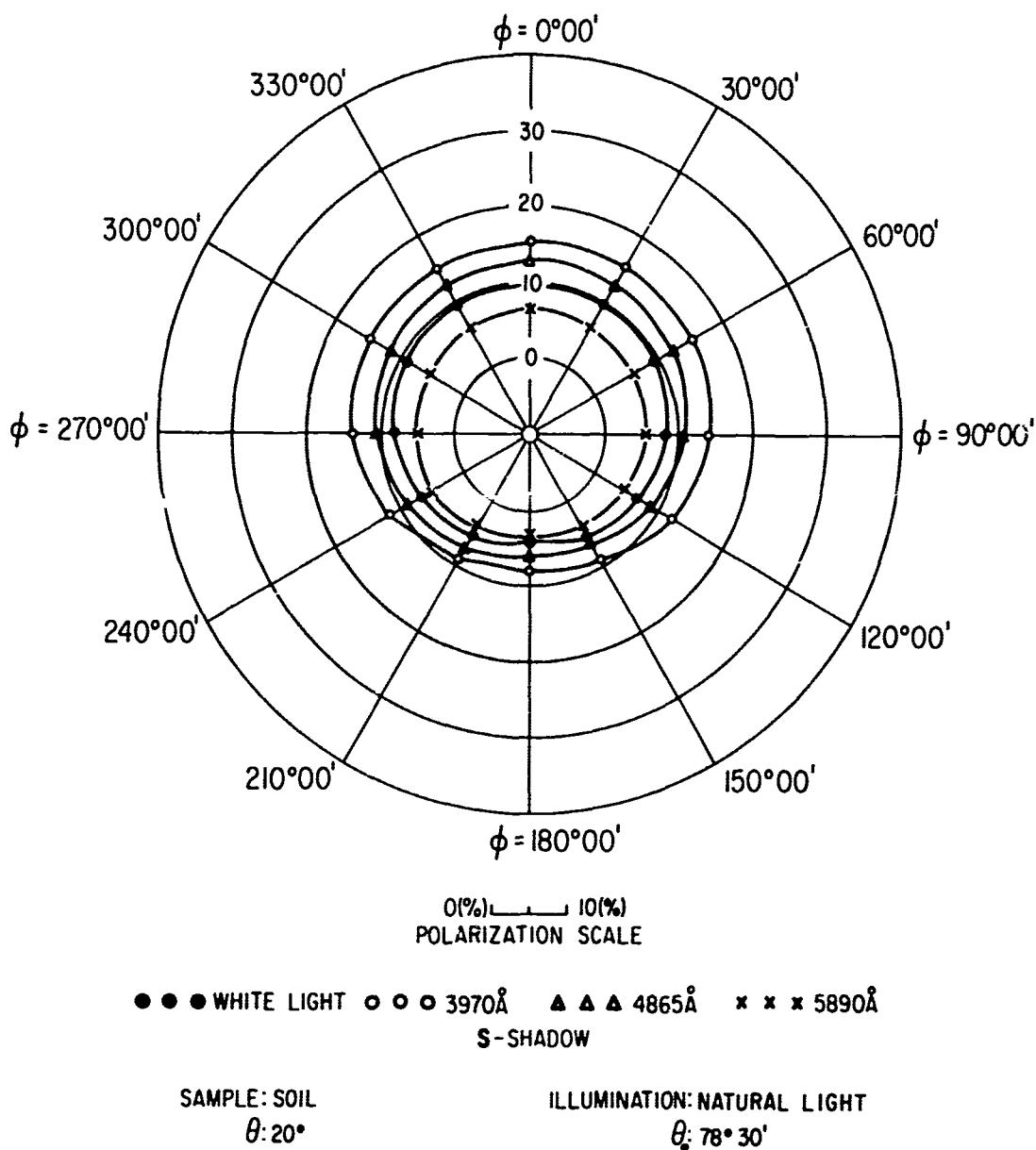
FIG. 197 POLAR DIAGRAM SHOWING AZIMUTHAL VARIATION OF THE POLARIZATION OF REFLECTED LIGHT
