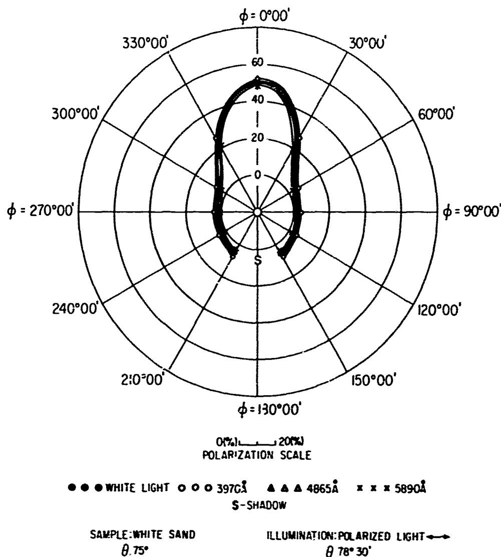
FIG. 145 POLAR DIAGRAM SHOWING AZIMUTHAL VARIATION OF THE POLARIZATION OF REFLECTED LIGHT
