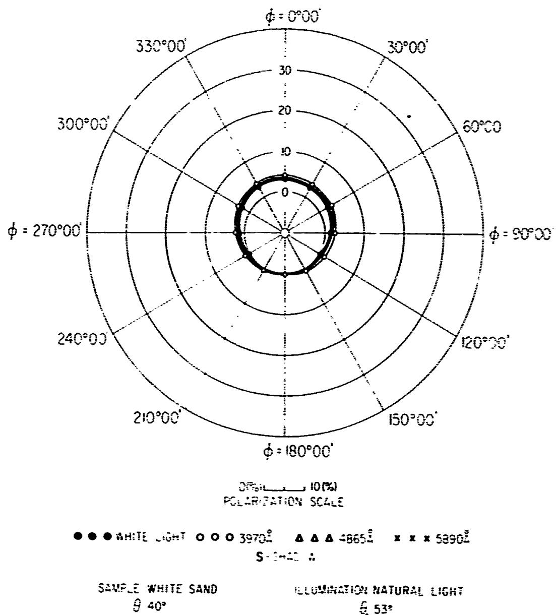
FIG 102 POLAR DIAGRAM SHOWING AZIMUTHAL VARIATION
