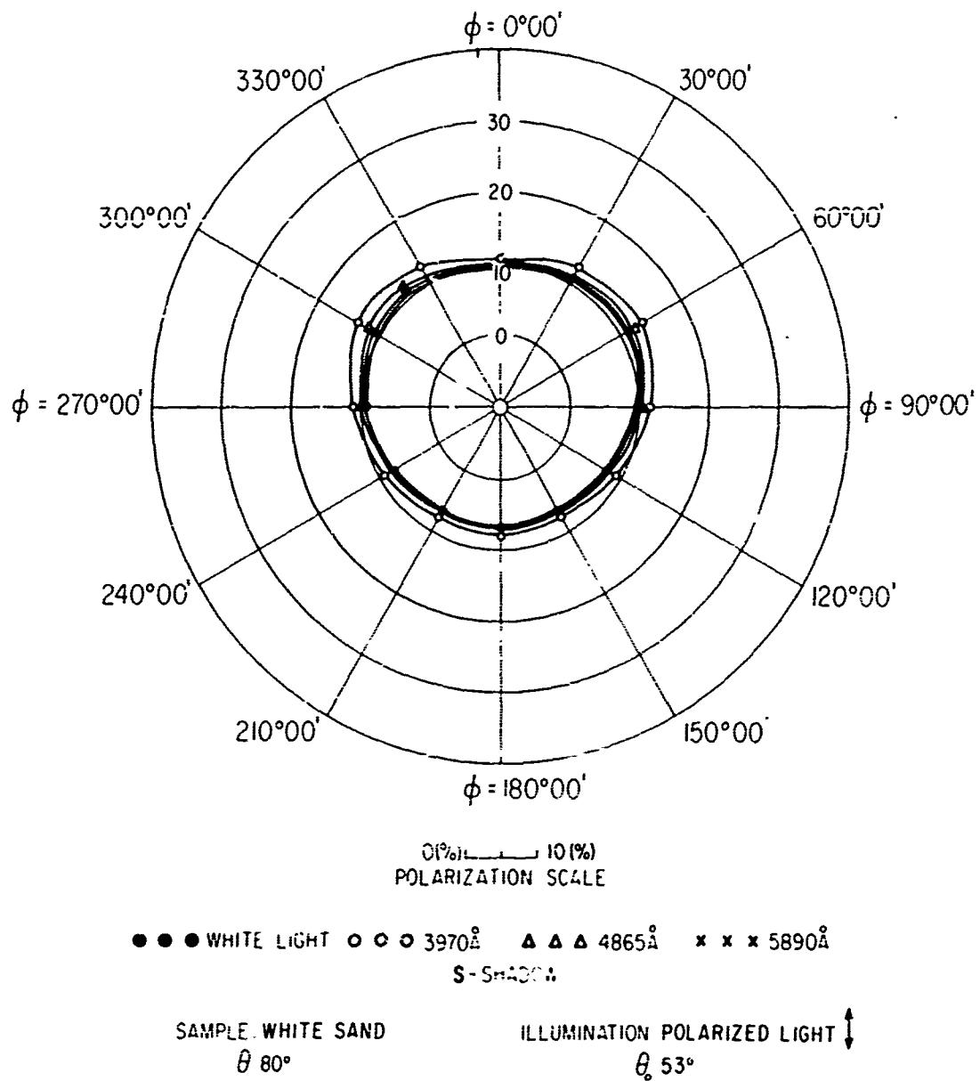
FIG 165 POLAR DIAGRAM SHOWING AZIMUTHAL VARIATION OF THE POLARIZATION OF REFLECTED LIGHT
