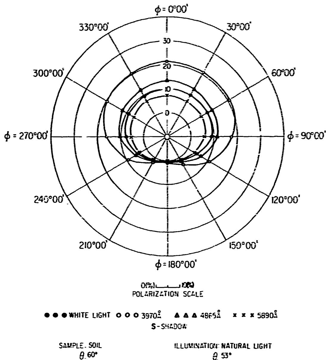
FIG. 191 POLAR DIAGRAM SHOWING AZIMUTHAL VARIATION
