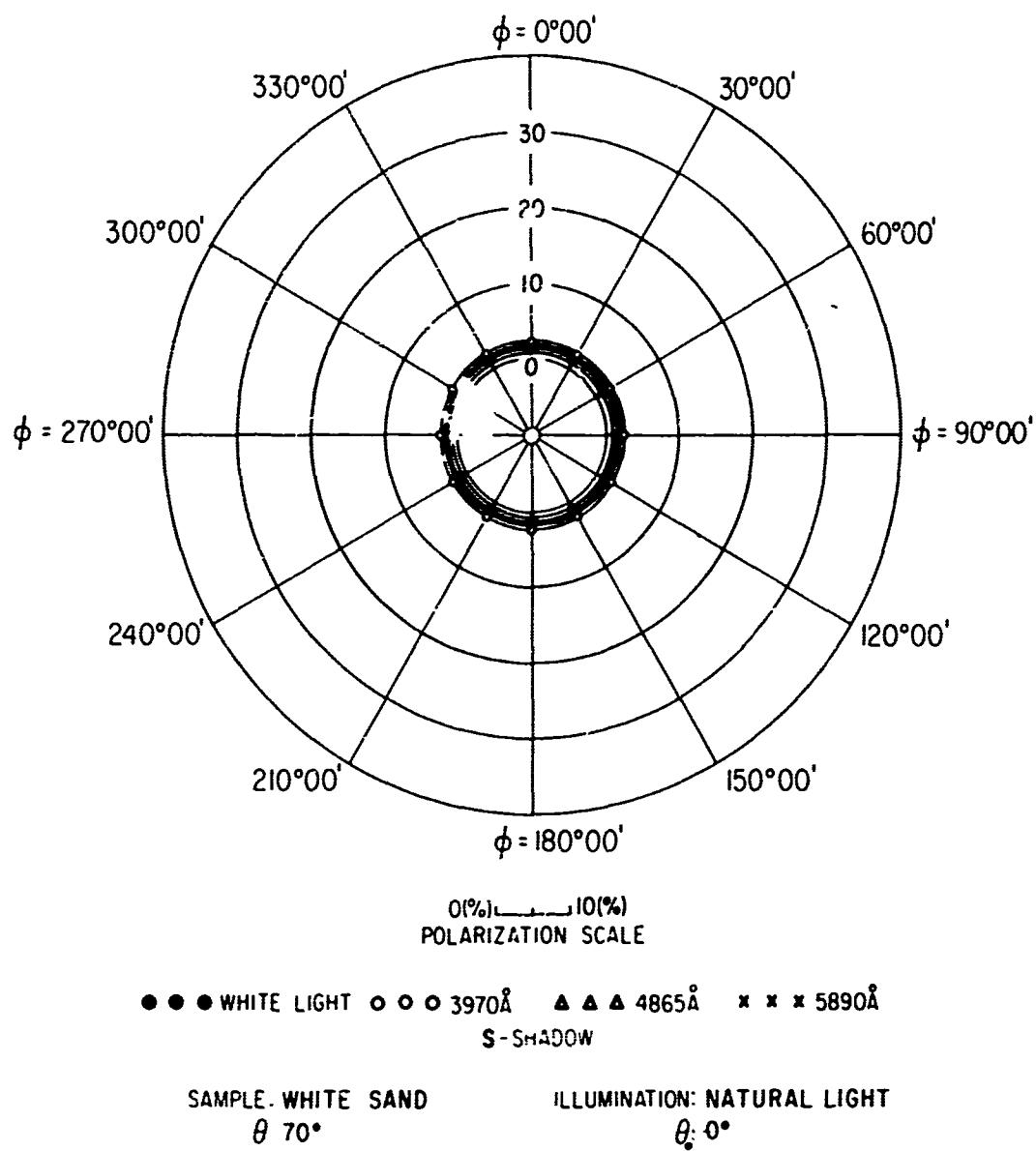
FIG 95. POLAR DIAGRAM SHOWING AZIMUTHAL VARIATION
