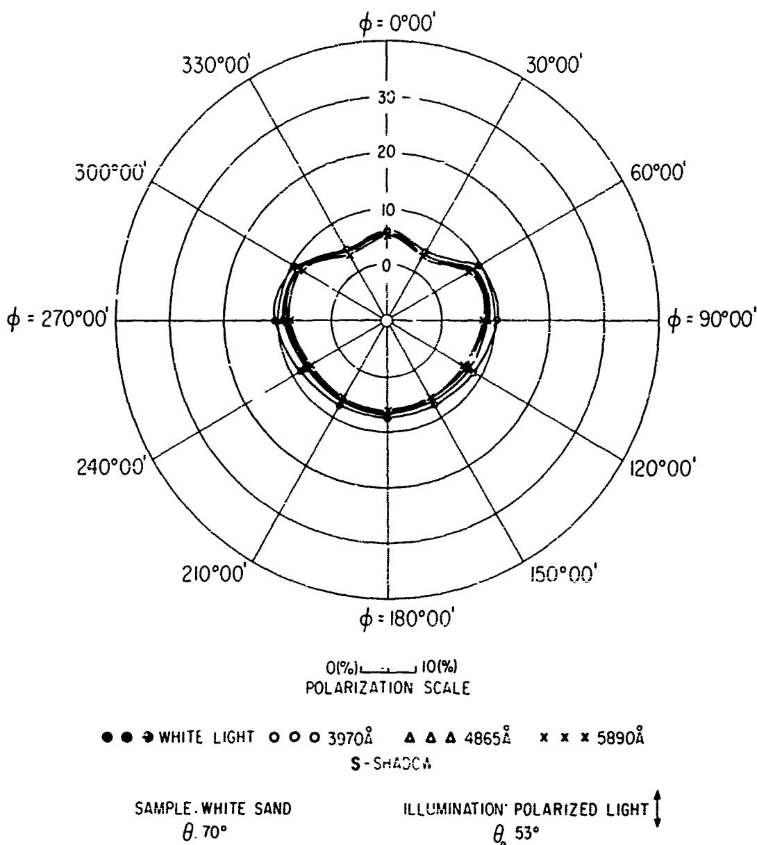
FIG 163 POLAR DIAGRAM SHOWING AZIMUTHAL VARIATION OF THE POLARIZATION OF REFLECTED LIGHT
