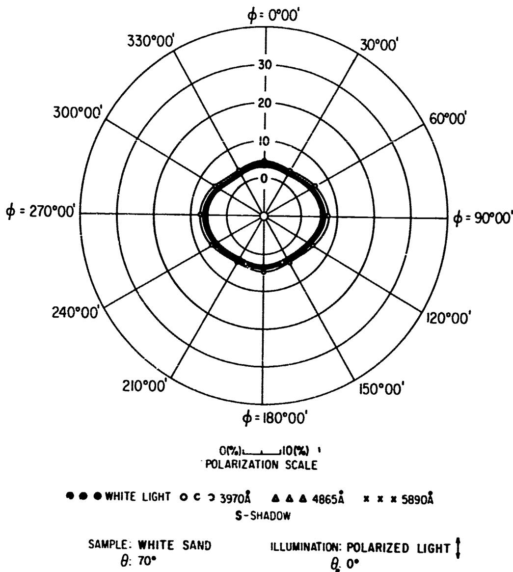
FIG 153 POLAR DIAGRAM SHOWING AZIMUTHAL VARIATION
