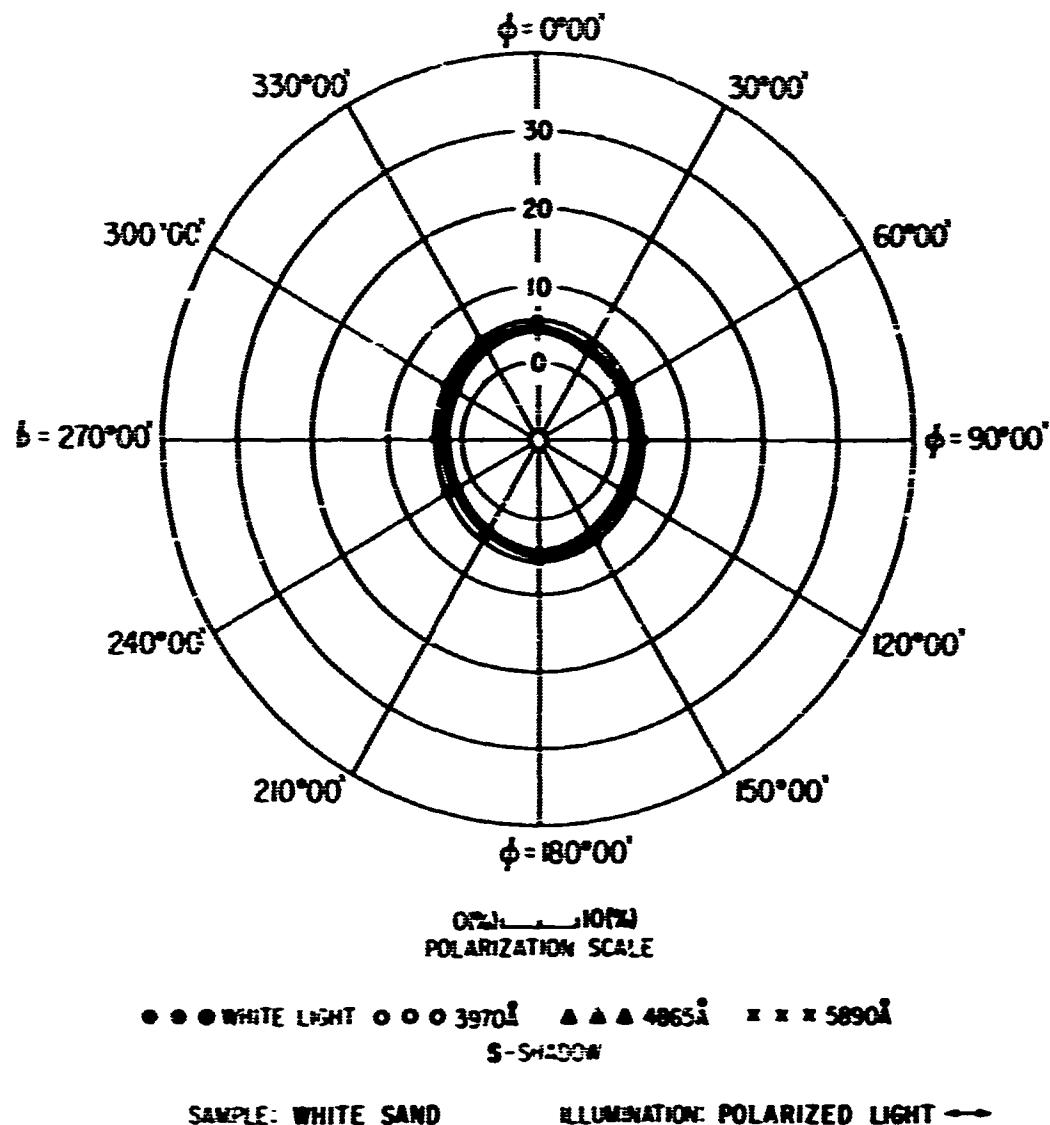
FIG 123. POLAR DIAGRAM SHOWING AZIMUTHAL VARIATION OF THE POLARIZATION OF REFLECTED LIGHT
