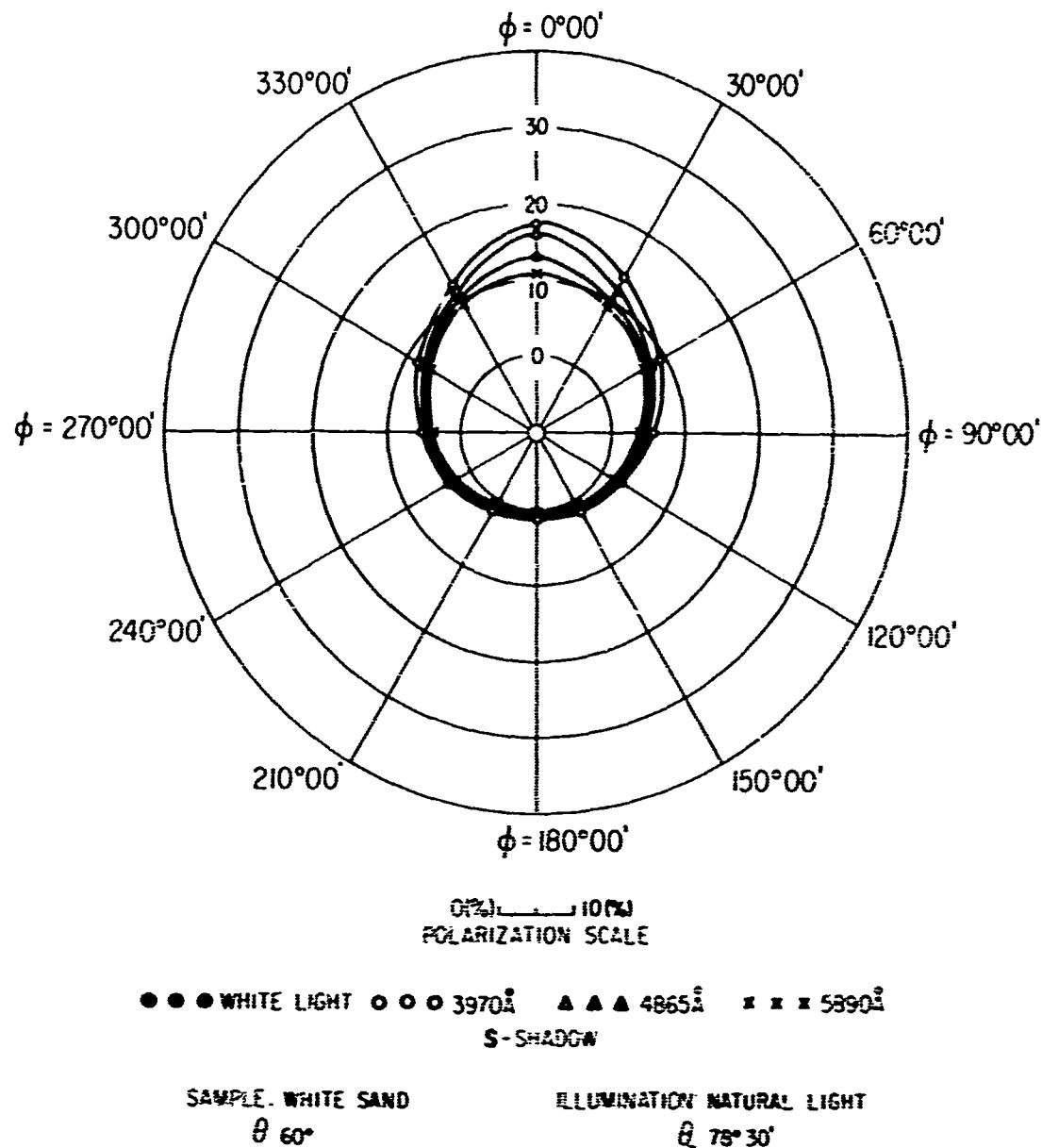
FIG III4 POLAR DIAGRAM SHOWING AZIMUTHAL VARIATION
