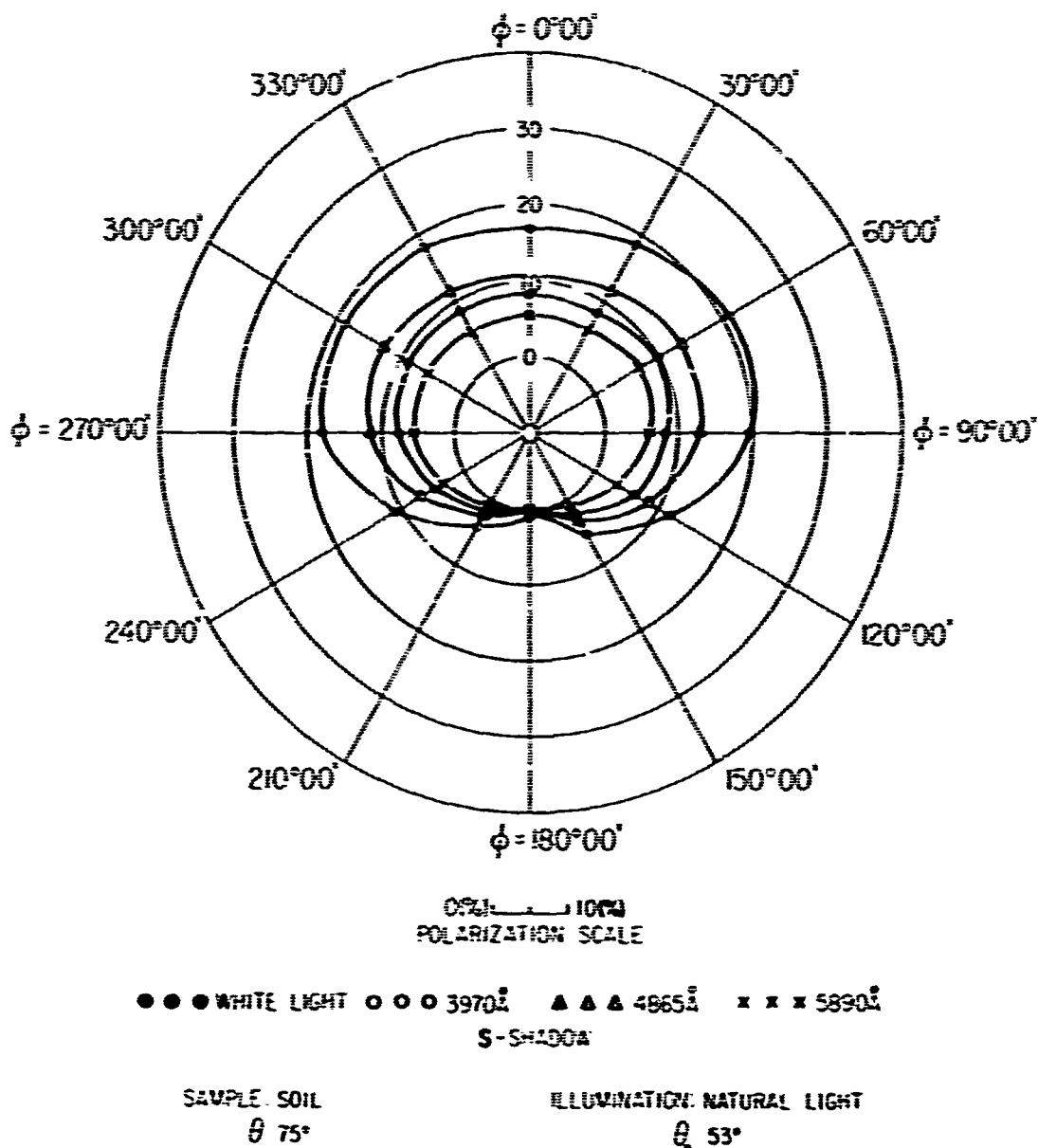
FIG 193 POLAR DIAGRAM SHOWING AZIMUTHAL VARIATION OF THE POLARIZATION OF REFLECTED LIGHT
