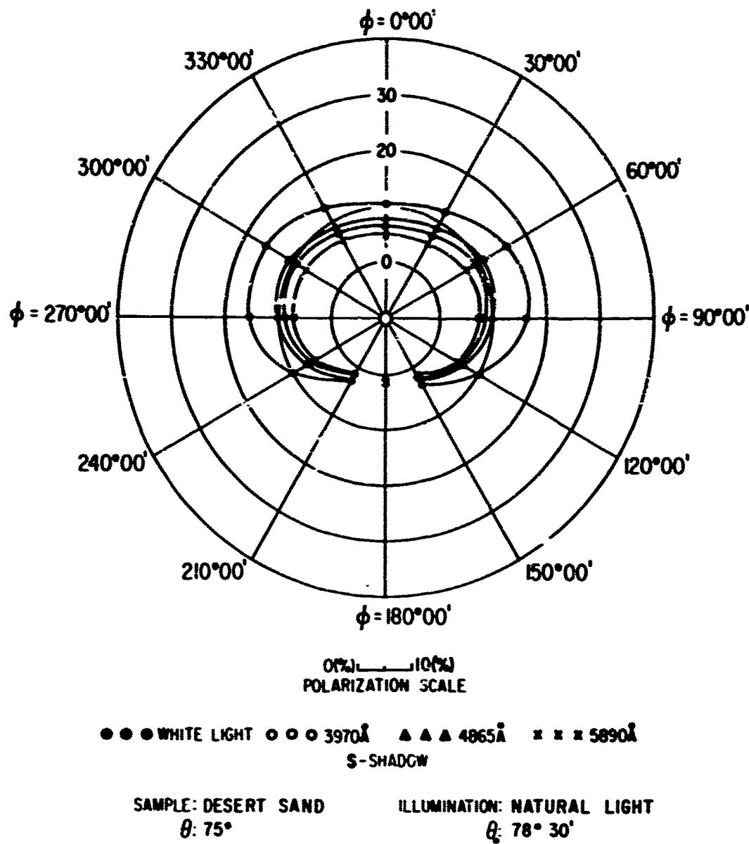
FIG 29. POLAR DIAGRAM SHOWING AZIMUTHAL VARIATION
