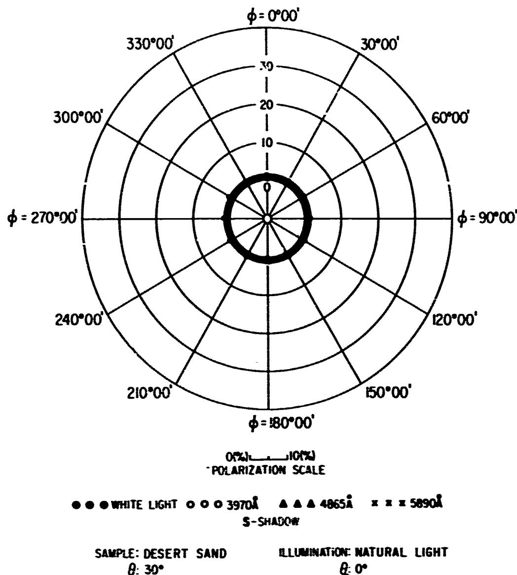
FIG. 4. POLAR DIAGRAM SHOWING AZIMUTHAL VARIATION OF THE POLARIZATION OF REFLECTED LIGHT
