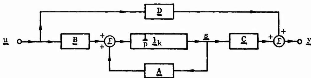
Fig. III-1. BLOCK DIAGRAM FOR CANONICAL EQUATIONS.
