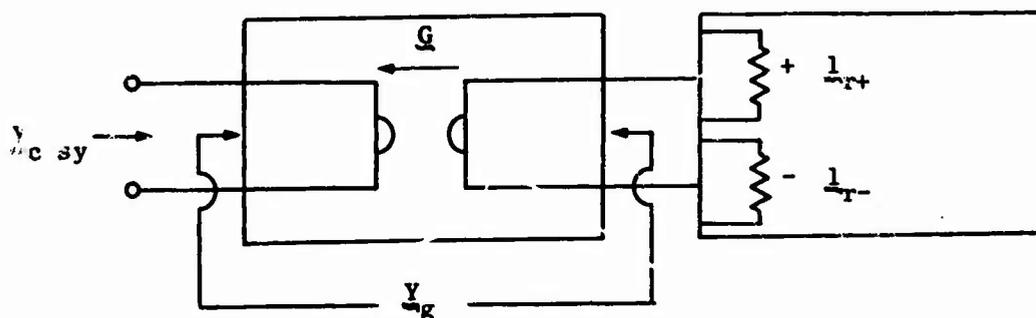
Fig. III-8. CONFIGURATION FOR SYMMETRIC PART OF  $Y_{mc}$ .
