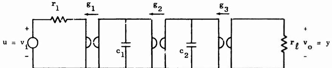
Fig. EII-1. DEGREE TWO FILTER.
