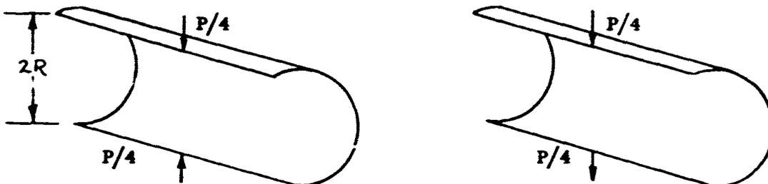
The problem now becomes that of finding the displacements in a semi-cylindrical "membrane" which, in addition to an internal pressure is loaded along its straight edges as shown.
