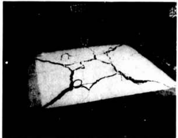
d. 612 psf (2988.0 kg/m 2 ), after failure
