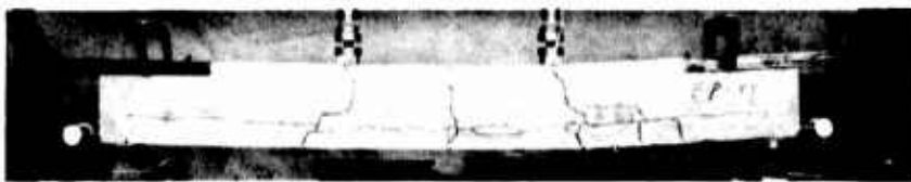
g. Total load = 6000 lb (2721.6 kg), failure
