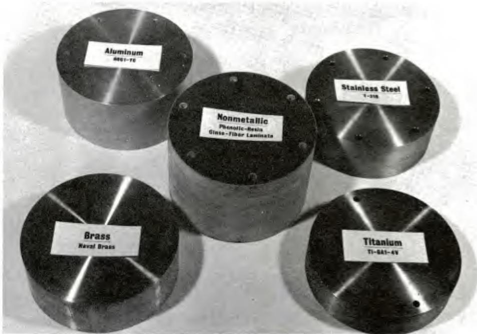
Figure 16. Typical end closures used to evaluate the effect of end-closure material on short-term critical pressure of 4-inch-ID x 6-inch-long glass pipe with flanged ends.
