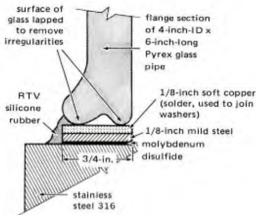
Figure 22. Experimental sealing and bearing system utilizing a composite copper–steel washer between the glass pipe end flange and the metal end-closure plate.
