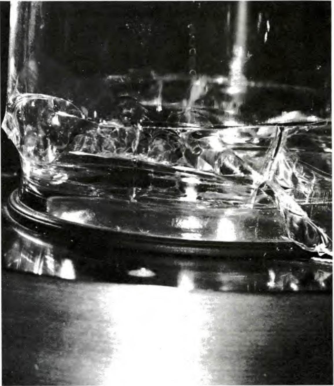
Figure 19. Closeup of failure area of glass pipe tested with O-ring gasket between glass pipe and flange and metal end-closure plate.
