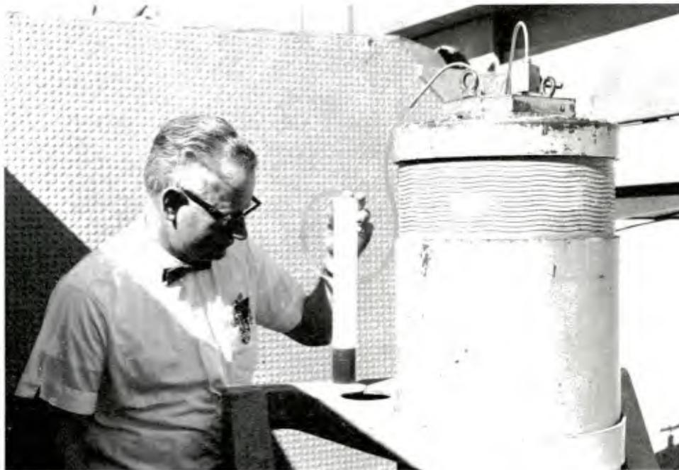
Figure 14. Typical setup used to measure the water displaced from and detect leaks in a test assembly during pressurization. The displaced water is collected and measured in the graduated cylinder at intervals of 1,000-psi pressure increase.
