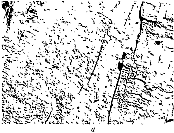
Figure 10. Stress-corrosion failure in a Ti-8Al notched specimen failed in 0.6M KI. 3500 X
