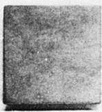
Very light spalling along edges. Coating changing color |
