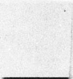
No damage                        | After five cycles from 80° to 1000°F |
