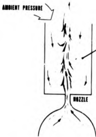
Figure 3. Initial fluid flow between parallel walls.
