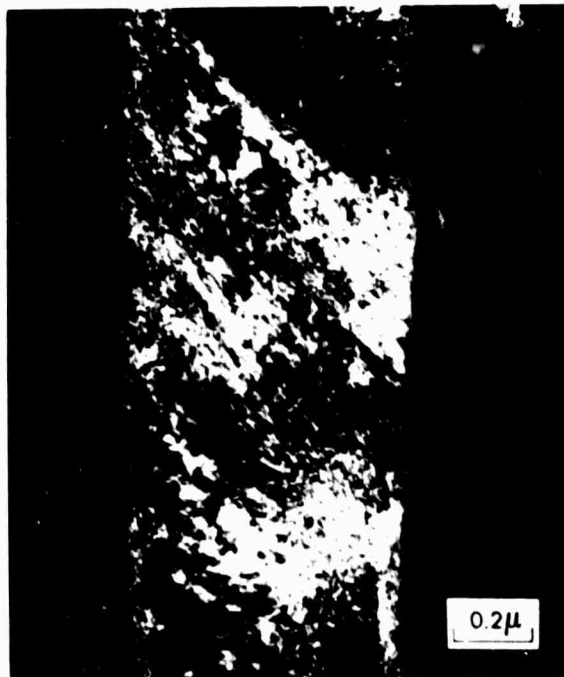
Fig. A-17 - Dark-field electron micrograph imaging on a twin reflection, twin formed during 2% uniform elongation.
