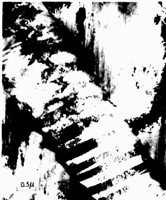
Fig. A-18 - Bright-field electron micrograph of twins formed during 10% uniform elongation
