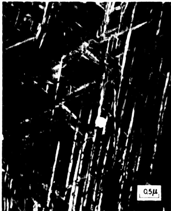
Fig. A-22 - Bright-field electron micrograph of Widmanstätten alpha formed during aging at 850° F for 64 hr.
