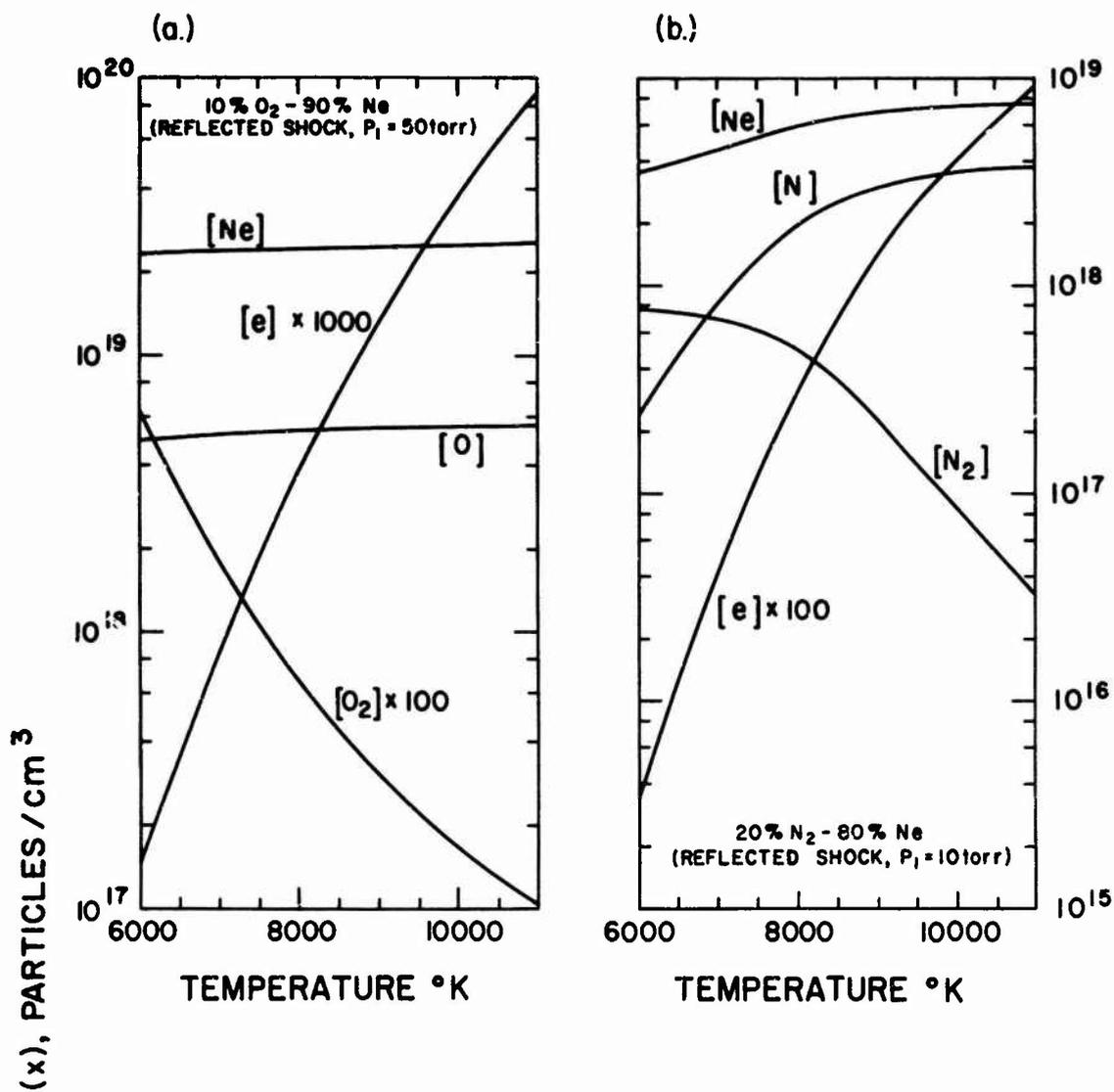
Fig. 1 Experimental conditions for various gas mixtures. Shown are various species concentrations [ ] in particles/cm<sup>3</sup> at the equilibrium temperature behind a reflected shock for (a) 10% O<sub>2</sub>-90% Ne at an initial pressure p<sub>1</sub> = 50 torr, (b) 20% N<sub>2</sub>-80% Ne at p<sub>1</sub> = 10 torr, (c) N<sub>2</sub> at p<sub>1</sub> = 10 torr, and (d) air at p<sub>1</sub> = 10 torr. Only the concentrations of the major neutral species and electrons have been shown.
