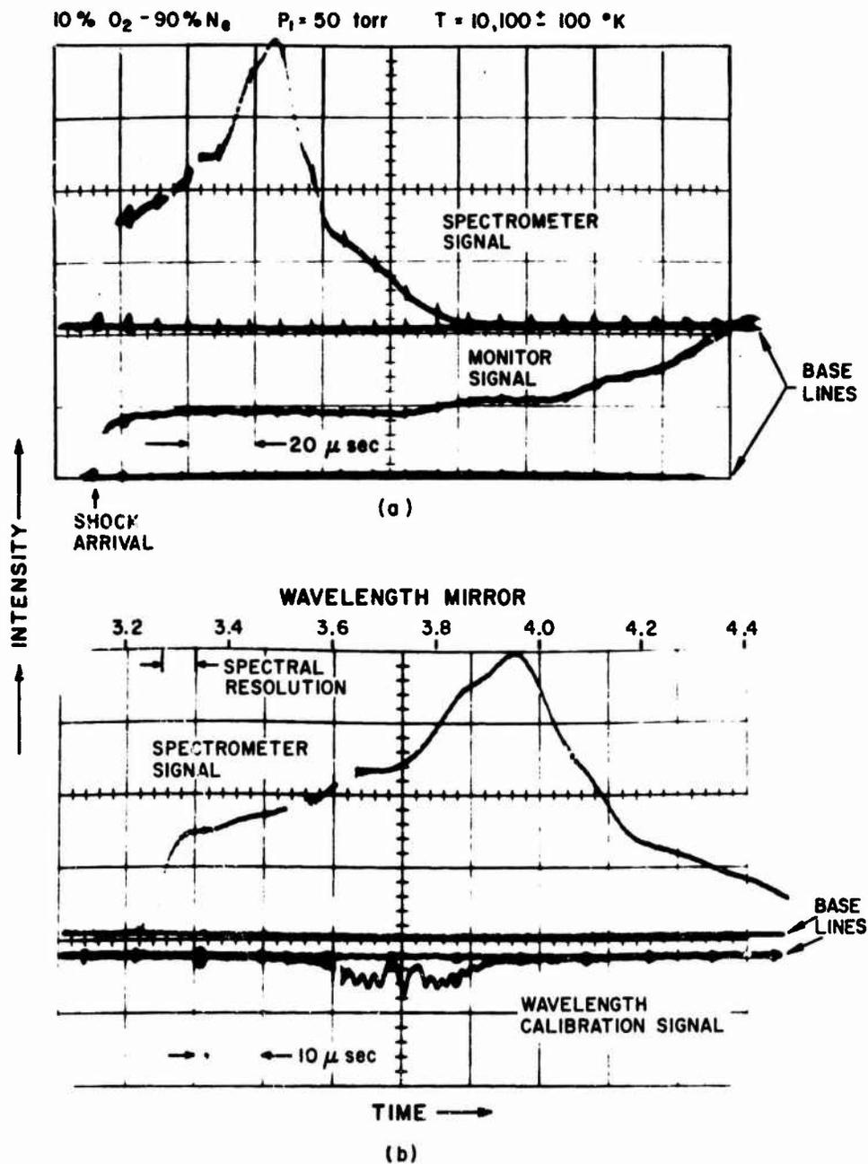
Fig. 2 Oscillograms illustrating data obtained from a shock into  $p_1 = 50$  torr of a 10% O<sub>2</sub>-90% Ne mixture. Final equilibrium temperature was 10,100°K. Scope (a) shows the signals from the scanning infrared spectrometer and monitor PM at a sweep speed of 20  $\mu$ -sec/div. Scope (b) shows signals from the scanning spectrometer and the wavelength calibration at a sweep speed of 10  $\mu$ -sec/div.
