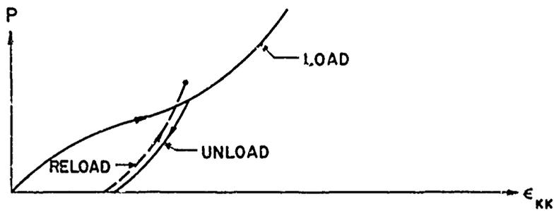
FIG. 6 - LOAD - UNLOAD - RELOAD RELATIONS
