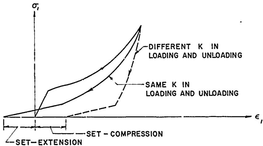
FIG. 5 UNIAXIAL STRAIN - ELIMINATION OF NET DILATION
