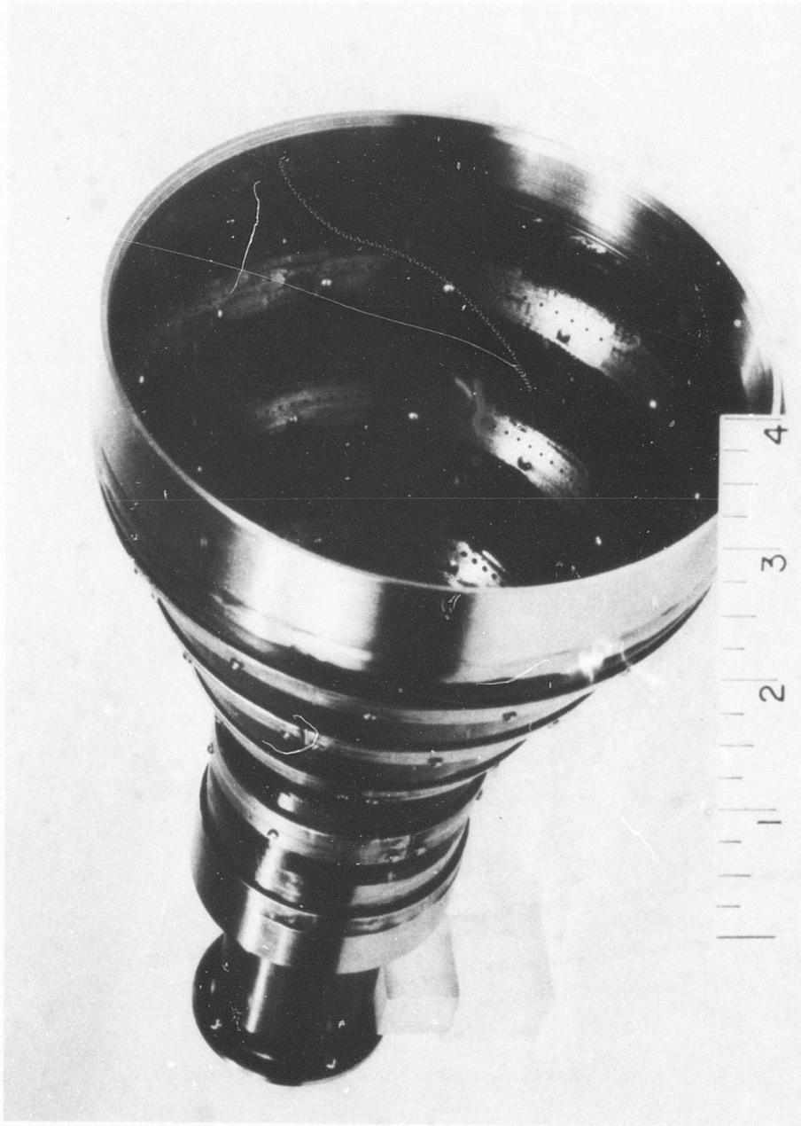
Figure 41. Combustor Inner Liner.
