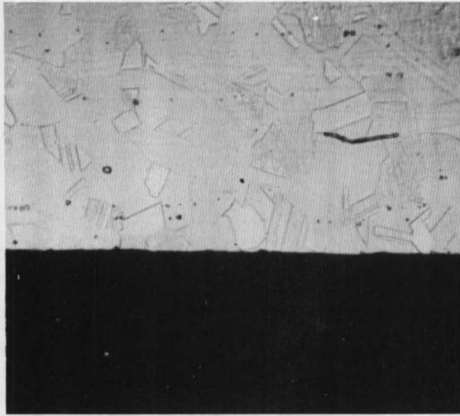
Fig. 21 Composite, Stainless Steel Portion away from Weld, Stressed and Exposed to MMH, 500X
