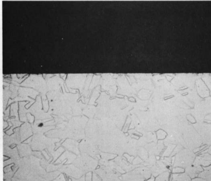
Fig. 11 Copper Control, Unexposed, 500X
