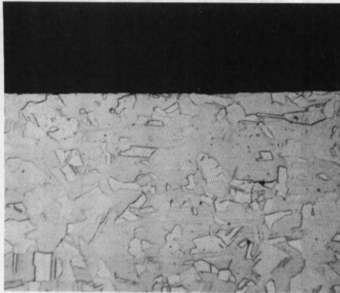
Fig. 14 Brazen Copper Exposed to MMH, Stressed, and Uncoated, 500X
