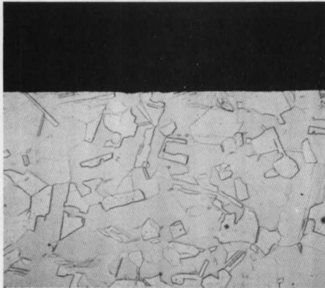
Fig. 25 Composite, Copper Portion away from Weld, Stressed and Exposed to MMH, 500X
