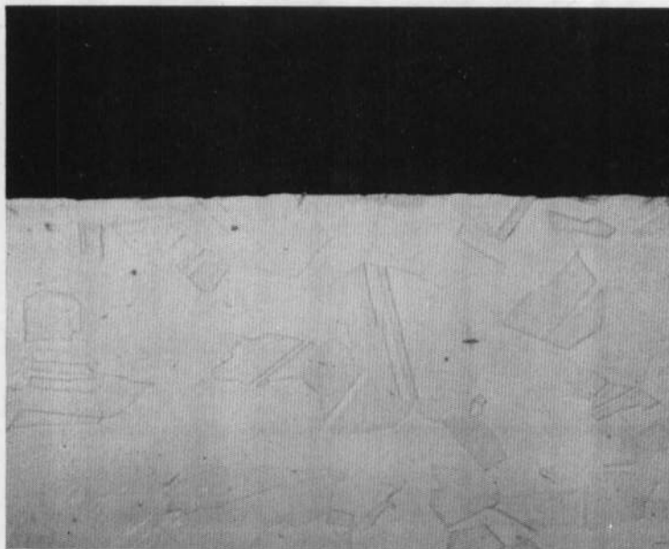
Fig. 30 Control, Stainless Steel Cryopanel, Unexposed, 500X
