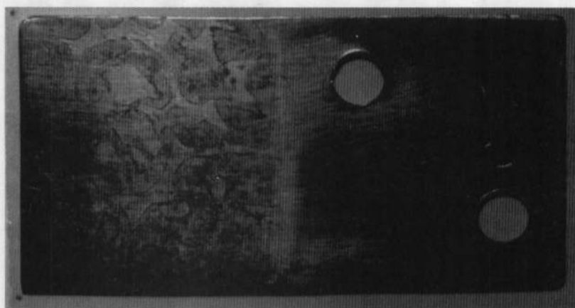
Fig. 10 Coating Stripped from Copper after MMH Exposure, 2X
