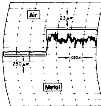
Fig. 14 Surface Profile of Thick Berylco-165 Specimen Shown in Fig. 13.
