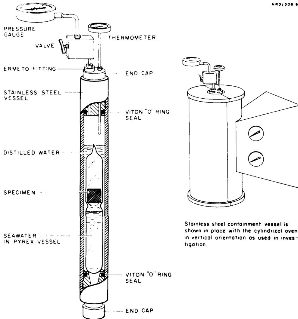
Fig. 1 Exposure Apparatus Used in Hot-Seawater-Vapor Experiment.
