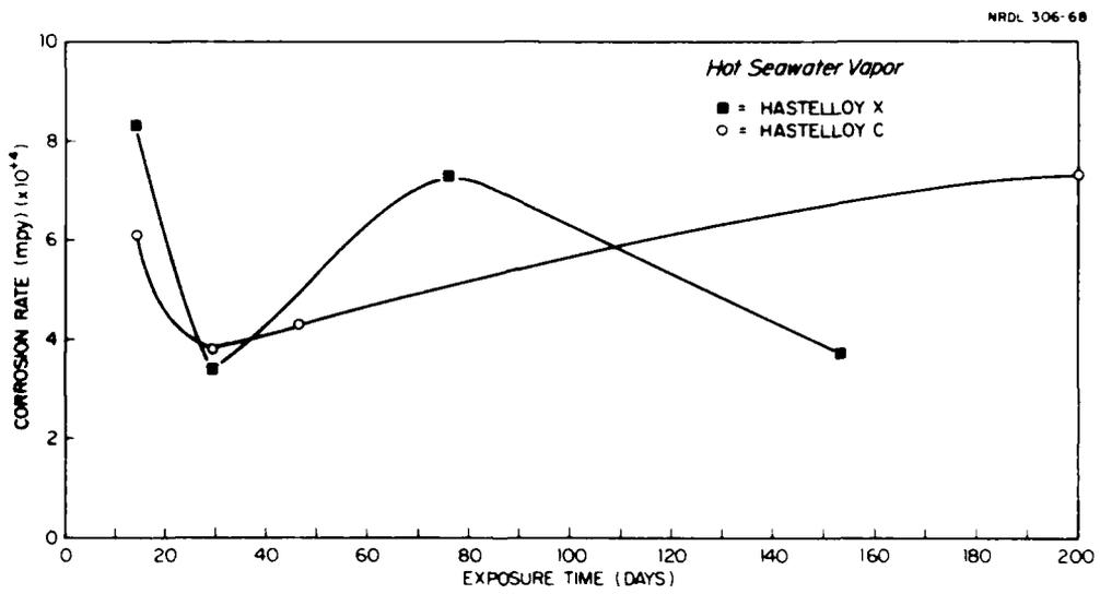
Fig. 20 Corrosion Rates of Hastelloy X and Hastelloy C in a Hot-Seawater-Vapor Environment.
