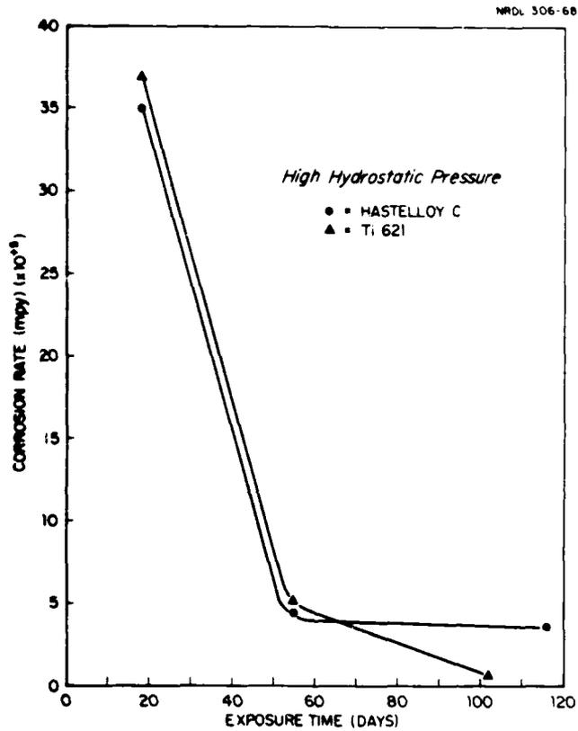
Fig. 21 Corrosion Rates of Hastelloy C and Titanium-621 Alloy in Seawater Under High Hydrostatic Pressure.
