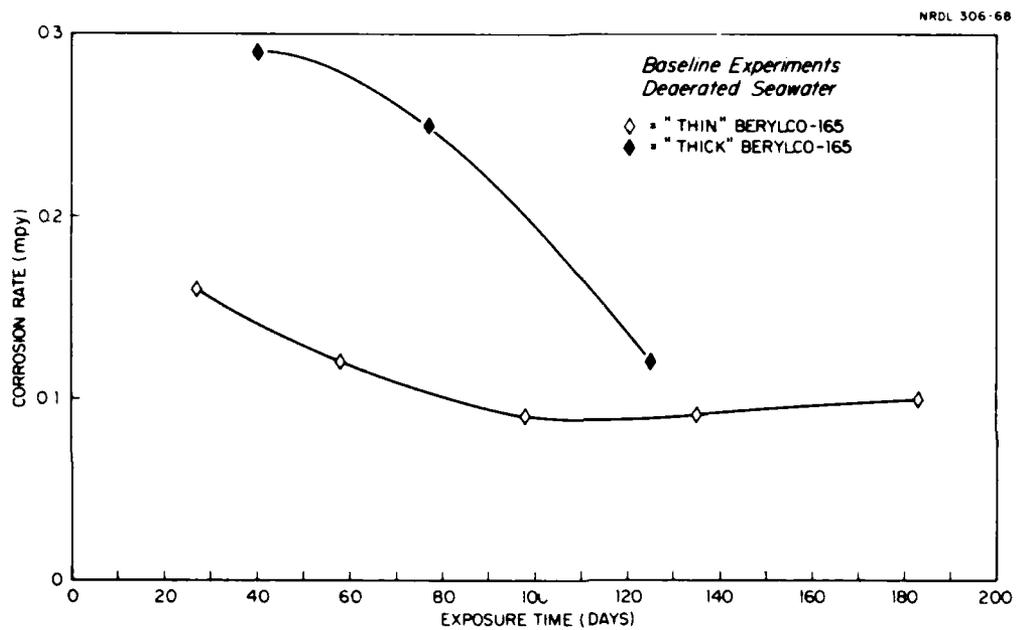
**Fig. 8 Corrosion Rates of Berylco-165 Alloy in Deaerated Seawater - Baseline Values.**
