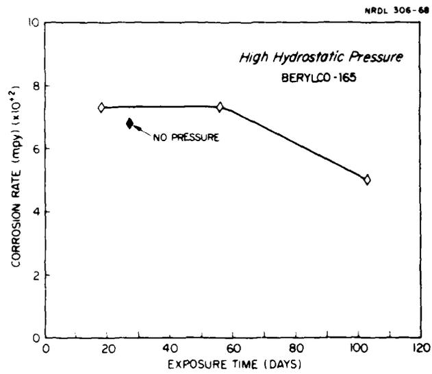
Fig. 22 Corrosion Rate of a Thin Beryllco-165 Specimen in Seawater Under High Hydrostatic Pressure.
