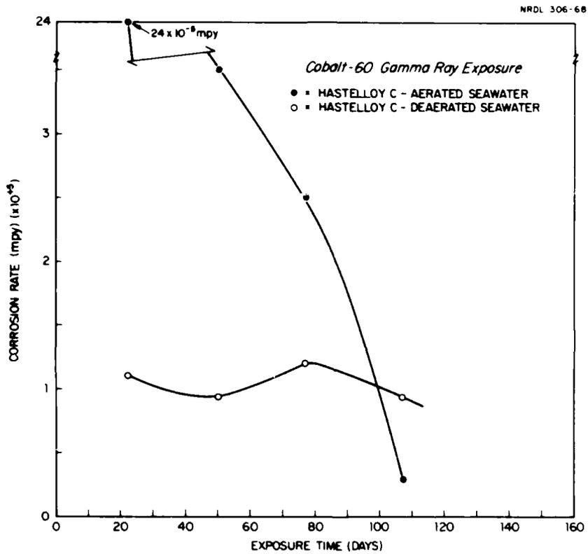
**Fig. 23** Corrosion Rates of Hastelloy C in Seawater in an Ionizing Radiation Field.
