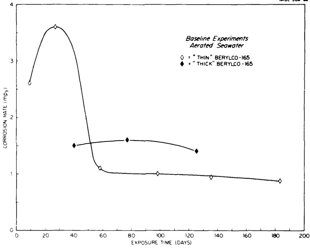
Fig. 7 Corrosion Rates of Berylco-165 Alloy in Aerated Seawater - Baseline Values.
