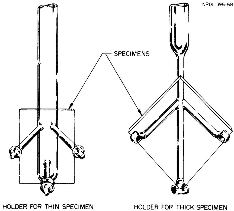
Fig. 4 Pyrex Holders for Thin and Thick Beryllco-165 Specimens.
