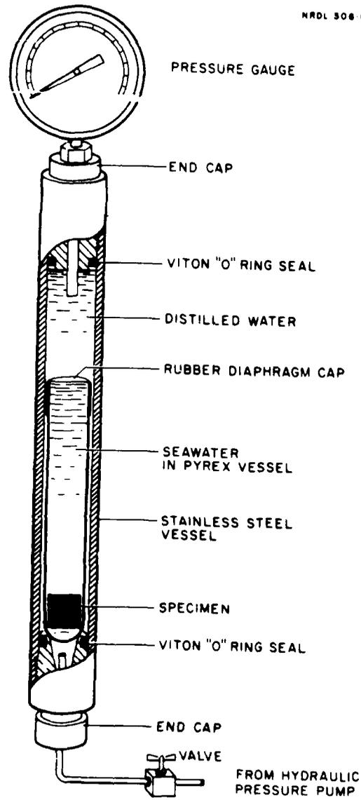
Fig. 2 Exposure Apparatus Used in High-Hydrostatic-Pressure Experiment.
