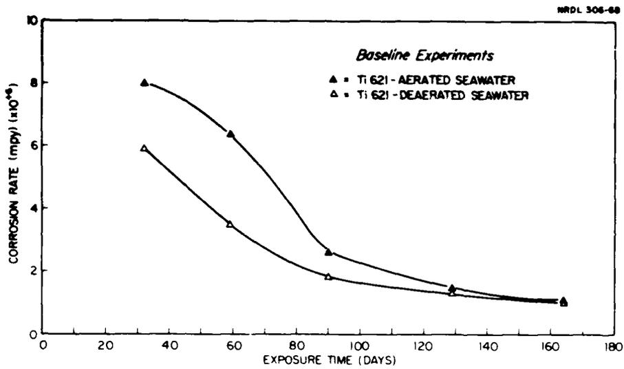
Fig. 6 Corrosion Rates of Titanium-621 Alloy in Seawater - Baseline Values.
