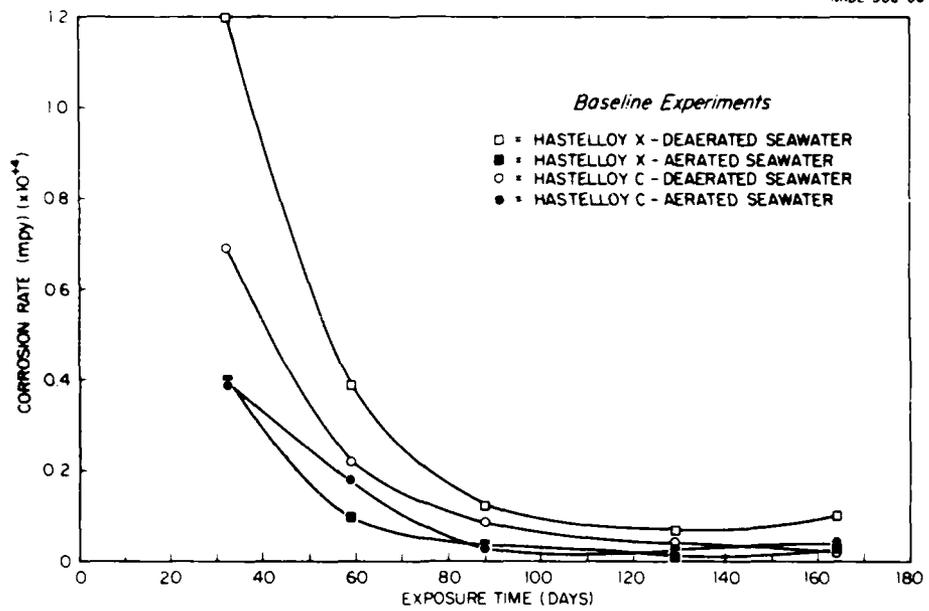
Fig. 5 Corrosion Rates of Hastelloy X and Hastelloy C in Seawater - Baseline Values.
