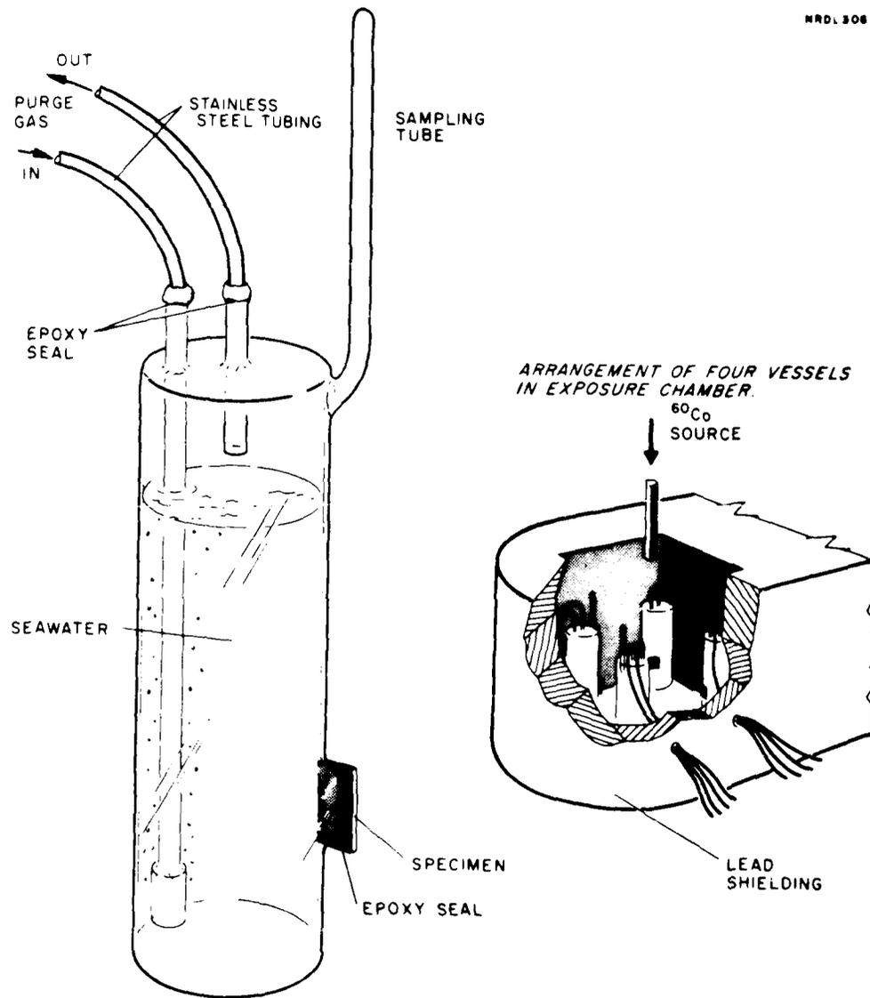
Fig. 3 Exposure Apparatus Used in Cobalt-60 Gamma-Ray Experiment.
