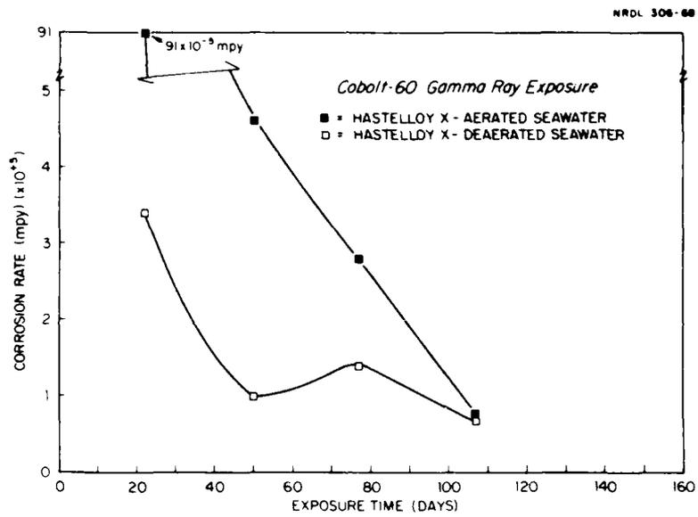
Fig. 24 Corrosion Rates of Hastelloy X in Seawater in an Ionizing Radiation Field.
