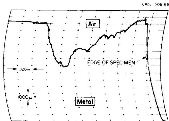
Fig. 11 Surface Profile of Local Corrosion on the Thin Beryllco-165 Specimen Shown in Fig. 9.
