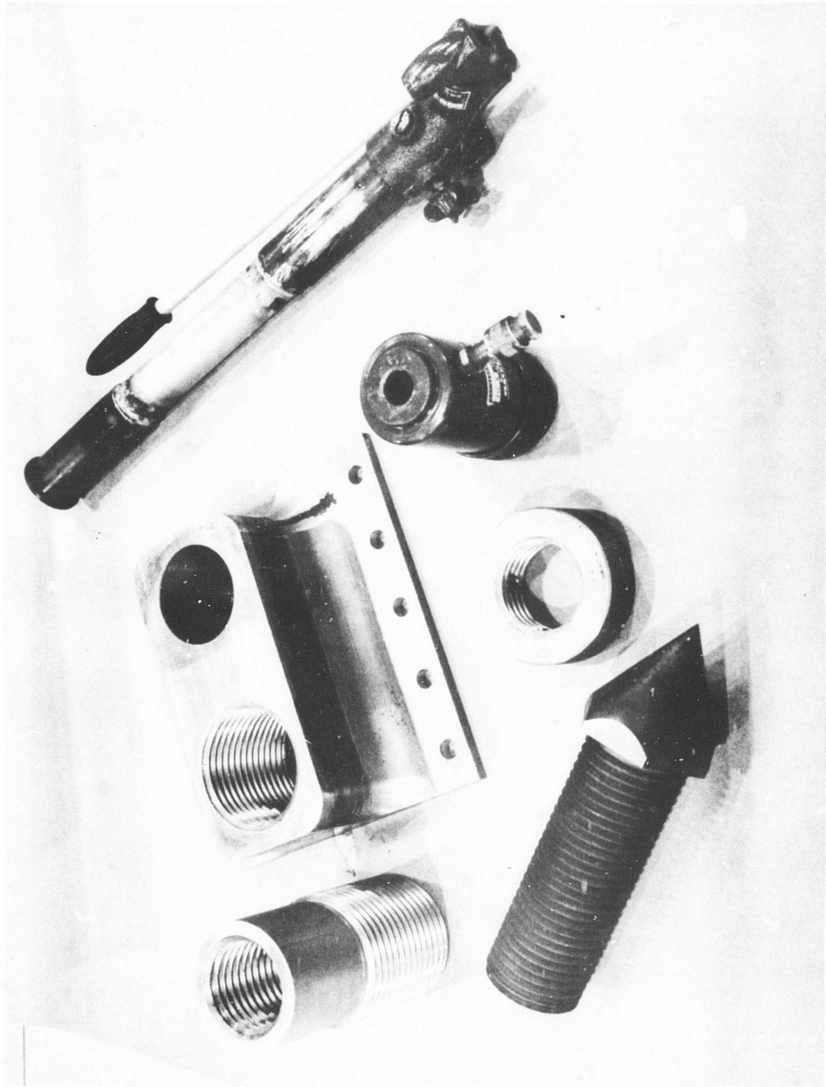
FIG. 18 Hydraulic Pump, Ram and Leveling Screw Support Units.
