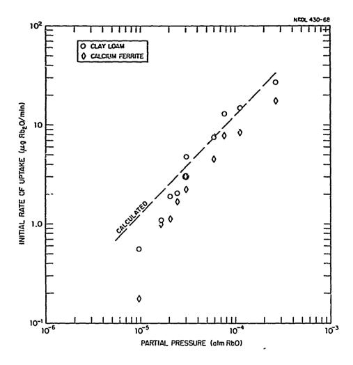
Fig. 7 Initial Rates of Uptake of RbO at  $1400^{\circ}$ C as a Function of RbO Partial Pressure. The initial rates are shown for both clay loam and calcium ferrite. The dashed line indicates the theoretically calculated uptake rate based on Maxwell's equation. Average particle diameter is  $0.345 \pm 0.010$  cm.
