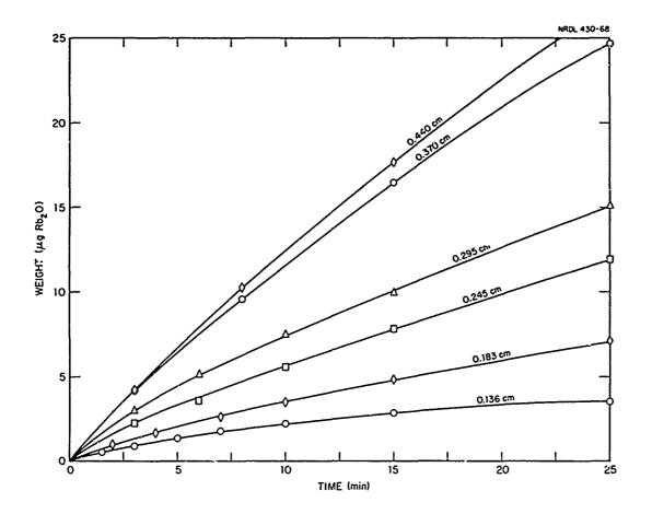
Fig. 5 Uptake of RbO by Calcium Ferrite as a Function of Particle Diameter and Time.  $T = 1200^{\circ}$ C, RbO partial pressure = 1.46 x 10<sup>-5</sup> atm.
