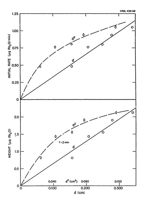
Fig. 12 The Initial Rate of RbO Uptake and the Amount of RbO Uptake at 2 Minutes by the Calcium Ferrite Particles as a Function of Particle Diameter and Diameter Squared.  $T = 1400^{\circ}$ , RbO partial pressure = 1.46 x 10-5 atm.
