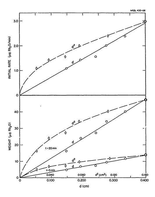
Fig. 10 The Initial Rate of RbO Uptake and the Amount of RbO Uptake at 5 and 20 Minutes by the Clay Loam Particles as a Function of Particle Diameter and Diameter Squared.  $T = 1400^{\circ}C$ , RbO partial pressure: 1.46 x 10<sup>-5</sup> atm.
