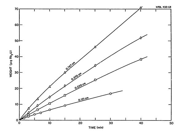
Fig. 6 Uptake of RbO by Calcium Aluminum Silicate as a Function of Particle Diameter and Time.  $T = 1400^{\circ}$ C, RbO partial pressure = 1.46 x 10<sup>-5</sup> atm.
