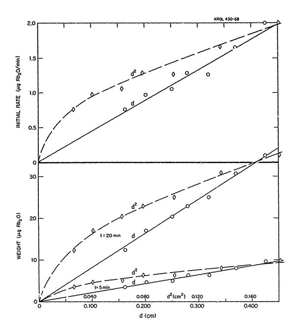
Fig. 11 The Initial Rate of RbO Uptake and the Amount of RbO Uptake at 5 and 20 Minutes by the Clay Loam Particles as a Function of Particle Diameter and Diameter Squared.  $T = 1200^{\circ}C$ , RbO partial pressure =  $1.46 \times 10^{-5}$  atm.
