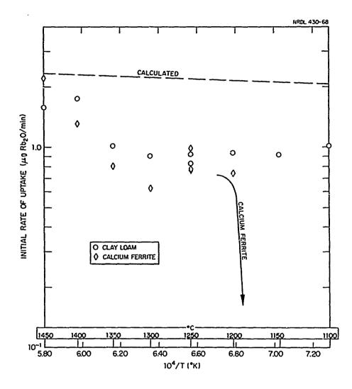
Fig. 8 Initial Rates of Uptake of RbO as a Function of Temperature at a Constant RbO Partial Pressure of  $1.85 \times 10^{-5}$  atm. The initial rates are shown for both the clay loam and the calcium ferrite. The dashed line indicates the theoretically calculated uptake rate based on Maxwell's equation. Average particle diameter is  $0.345 \pm 0.010$  cm.
