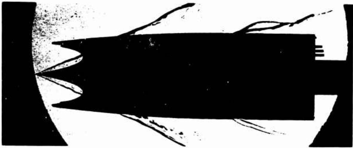
FIG. 12 SHADOWGRAPH OF UNSTARTED FOUR-MODULE INLET WITH COWL A
