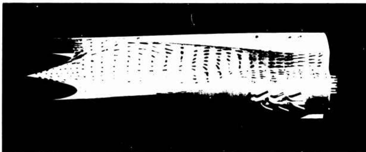
FIG. 16 OIL DOT STREAKS IN MODULE WITH UNSTARTED FLOW
