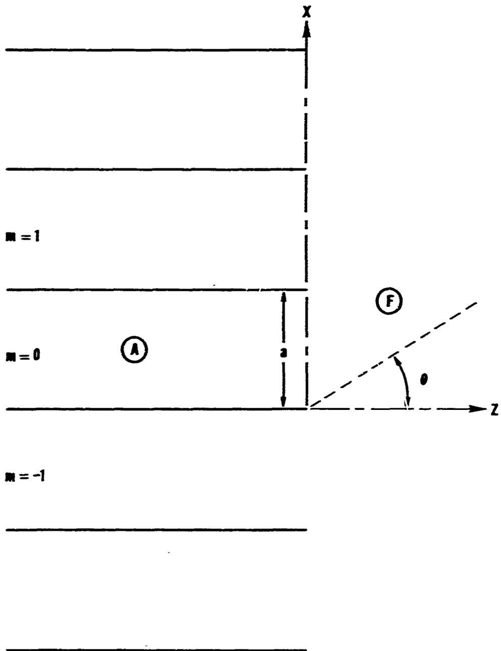
Figure 4.2 Infinite array of thin parallel plates
