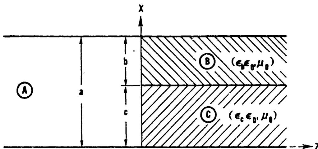
Figure 3.1 Inhomogeneously-filled waveguide bifurcation
