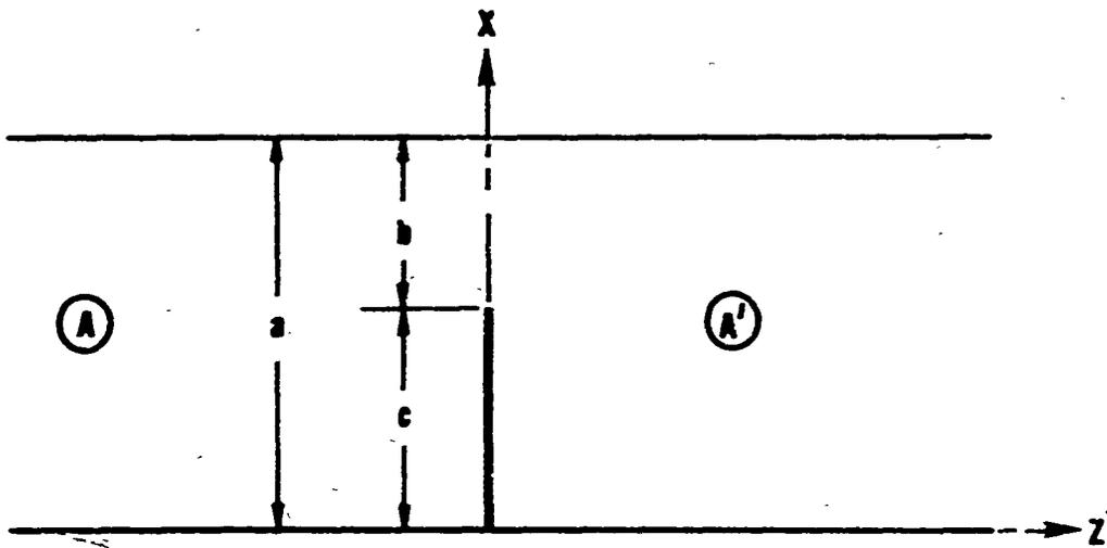
Figure 3.9 Waveguide inductive diaphragm
