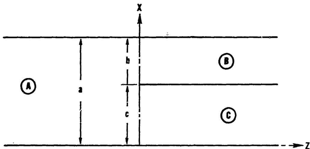
Figure 2.1 H-plane waveguide bifurcation
