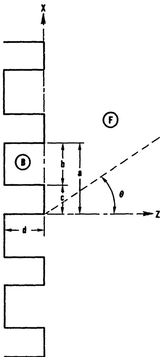
Figure 5.2 Metallic modulated diffracting surface
