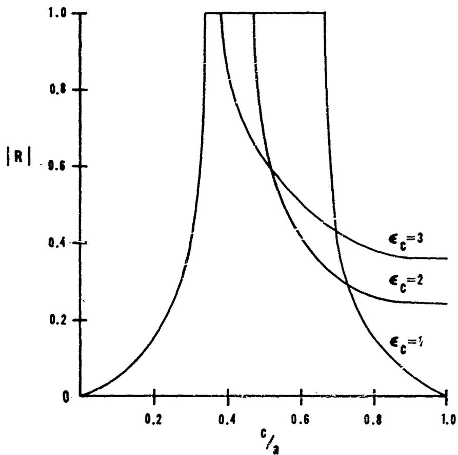
Figure 3.5 Reflection coefficient for inhomogeneously-filled bifurcation ( $\epsilon_b = 1.0$ ,  $a = 0.75\lambda$ )
