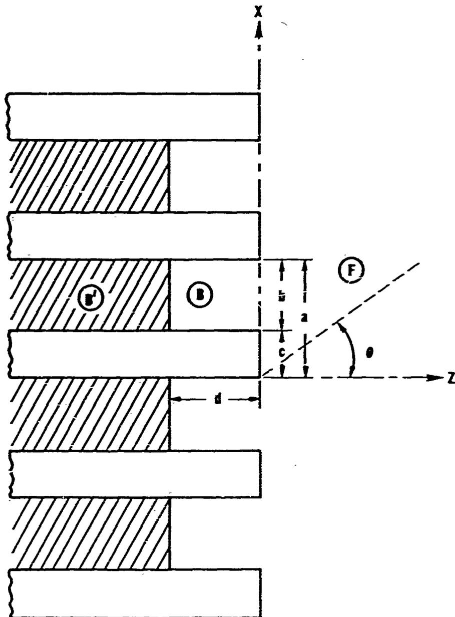
Figure 5.1 Infinite periodic diffracting surface
