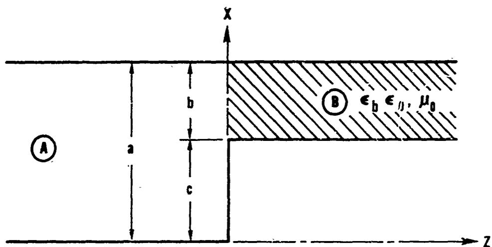
Figure 3.3 Waveguide step discontinuity
