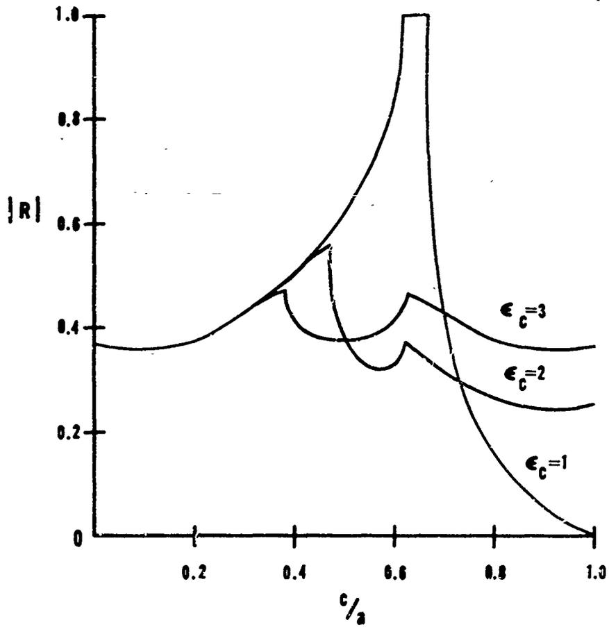
Figure 3.6 Reflection coefficient for inhomogeneously-filled bifurcation ( $\epsilon_b = 3.0$ ,  $a = 0.75\lambda$ )
