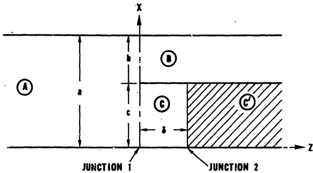
Figure 2.3 Auxiliary geometry for singly-inhomogeneous bifurcation
