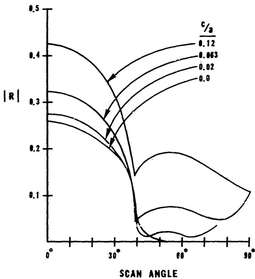
Figure 4.6 Reflection coefficients for thick-wall phased array
