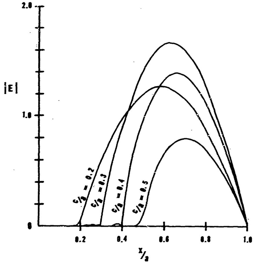
Figure 3.7 Amplitude of aperture electric field ( $a = 0.75\lambda$ )
