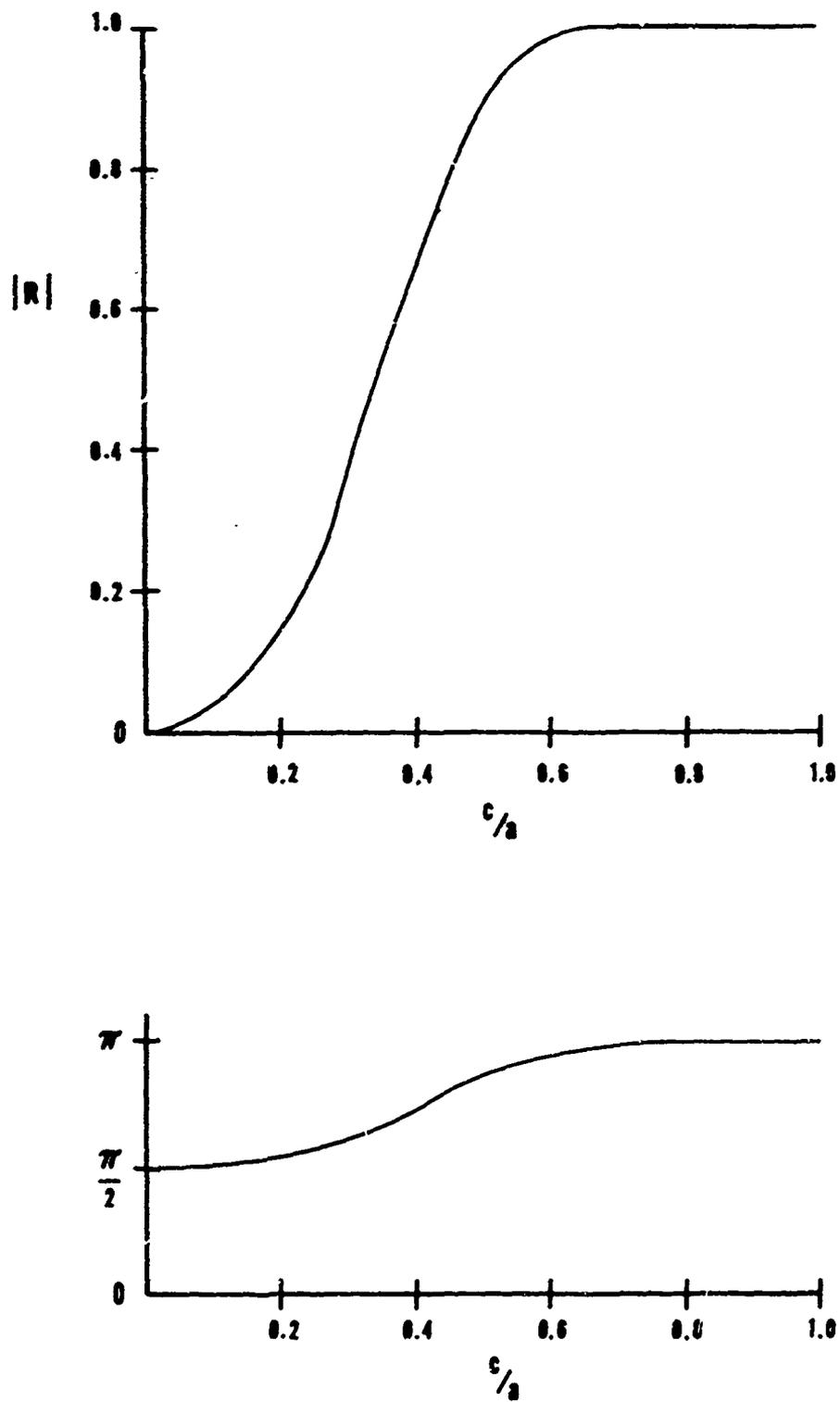
Figure 3.10 Reflection coefficient for waveguide diaphragm discontinuity
