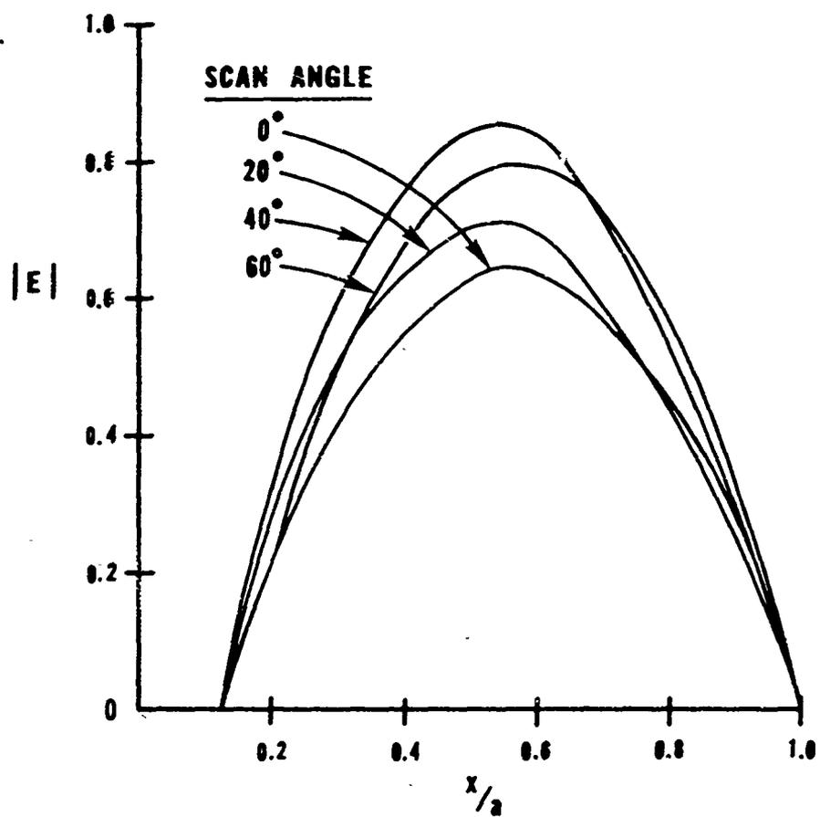
Figure 4.7 Aperture field for thick-wall array
