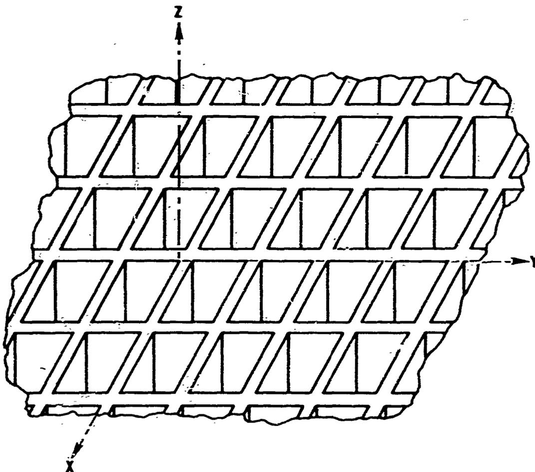
Figure 4.1 Phased array of open-end rectangular waveguides
