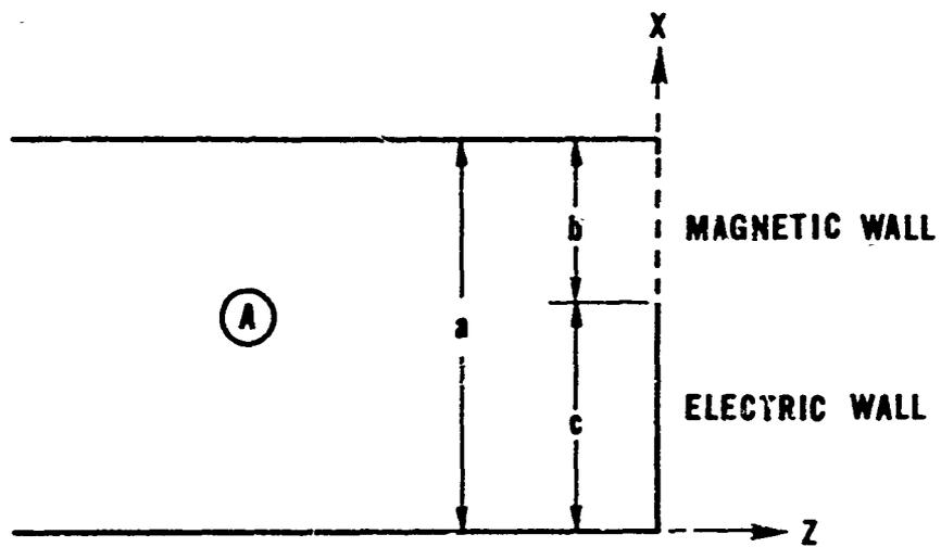
Figure 3.4 Magnetic-wall, electric-wall termination
