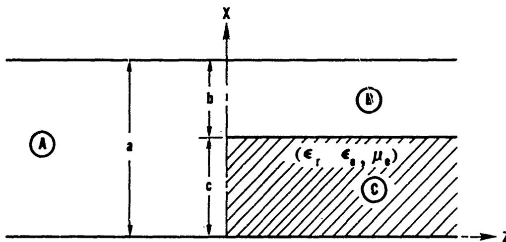
Figure 2.2 Singly-inhomogeneous waveguide bifurcation
