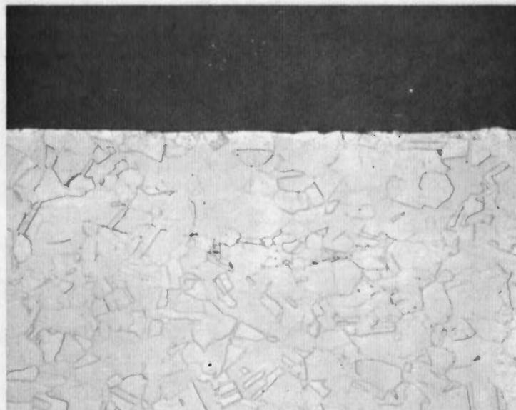
**Fig. 23 Unbraided Copper, Contacted Copper Fin, Exposed 58 hr to Cryodeposit, 441 hr to Gas, 9 cycles, 500X**
