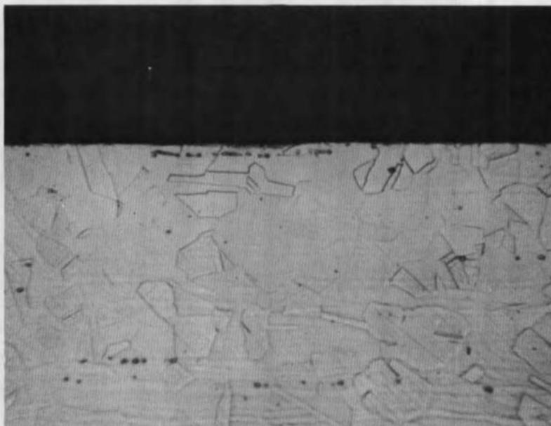
**Fig. 32 Composite Specimen, Stainless Steel Side, Exposed 58 hr to Cryodeposit, 441 hr to Gas, 9 cycles, Stressed, 500X**
