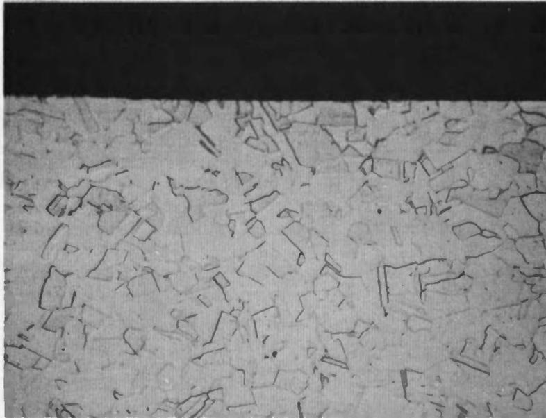
**Fig. 22 Control Specimen, Unbraided Copper, 500X**
