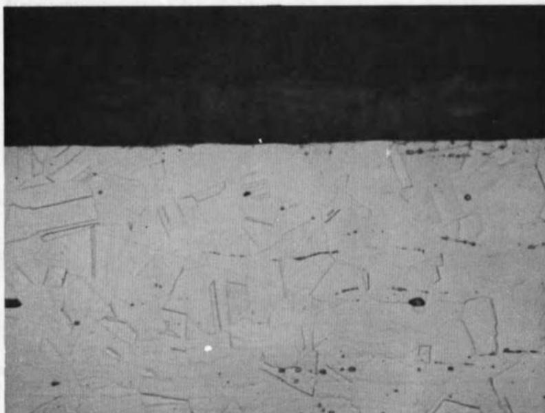
**Fig. 10** Stainless Steel 304L, Exposed 58 hr to Cryodeposit, 441 hr to Gas, 9 cycles, 500X
