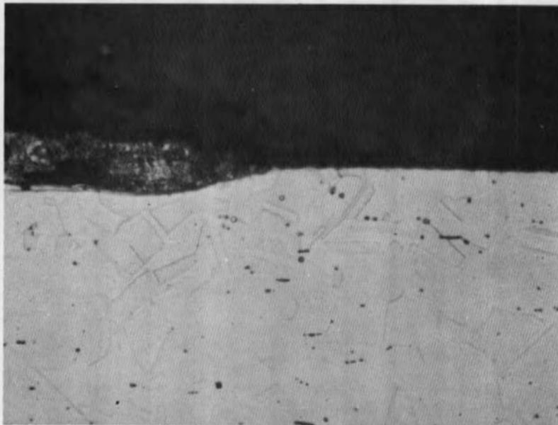
**Fig. 17** Stainless Steel 304L, at Resistance Spot Weld, Exposed 720 hr to Cryodeposit, 2816 hr to Gas, 20 cycles, 500X
