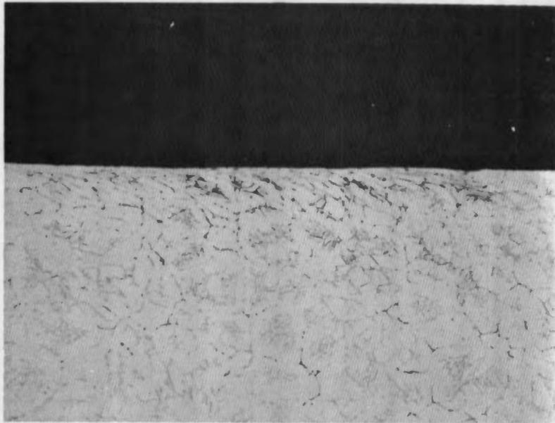
**Fig. 16** Stainless Steel 304L, Stressed, at 347 Rod Weld, Exposed 720 hr to Cryodeposit, 2816hr to Gas, 20 cycles, 500X
