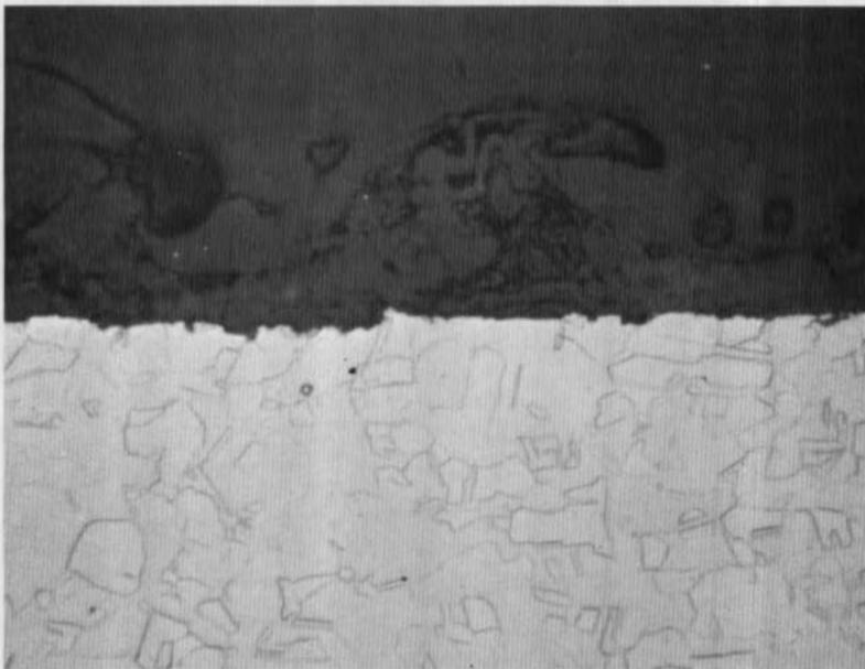
**Fig. 25 Unbrozed Copper, Contacted Aluminum Fin, Exposed 720 hr to Cryodeposit, 2816 hr to Gas, 20 cycles, 500X**
