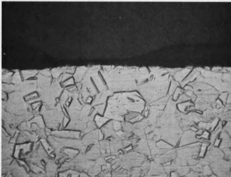
**Fig. 35 Composite Specimen, Copper Side, Exposed 58 hr to Cryodeposit, 441 hr to Gas, 9 cycles, Stressed, 500X**
