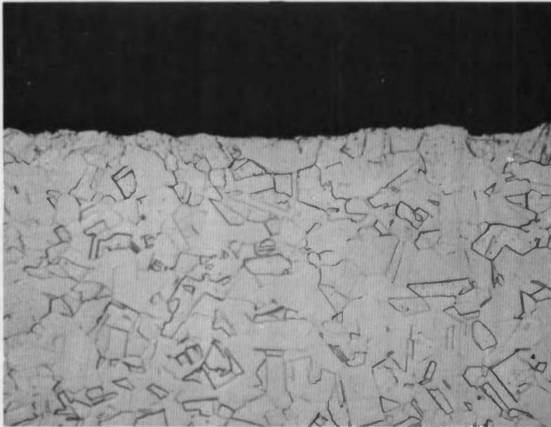
**Fig. 24 Brozed Copper, Contacted Copper Fin, Exposed 420 hr to Cryodeposit, 1190 hr to Gas, 8 cycles, 500X**
